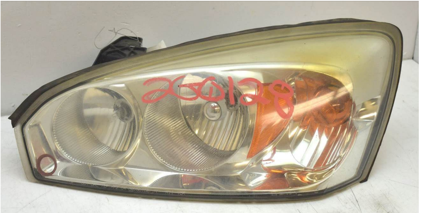
H-LH2 from 2005 Chevy Malibu (lens markings cleaned off with alcohol prior to testing)
