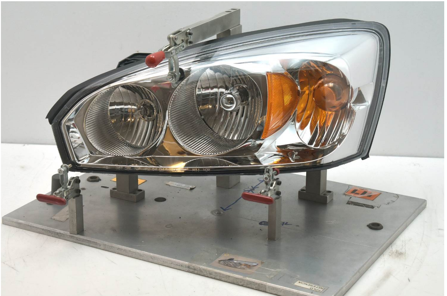
Lamp on Provided Fixture
