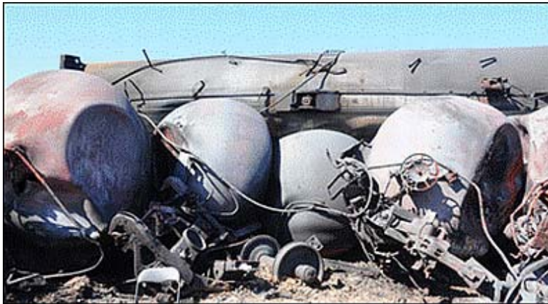
Figure 9 Class 111 Tank Cars Assumed in DEIR to Transport Crude (TSBC)
