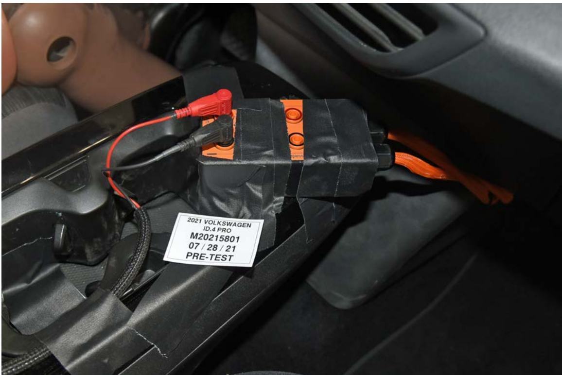
FIGURE 305-022. Pre-Impact View of High Voltage Leads Attached
