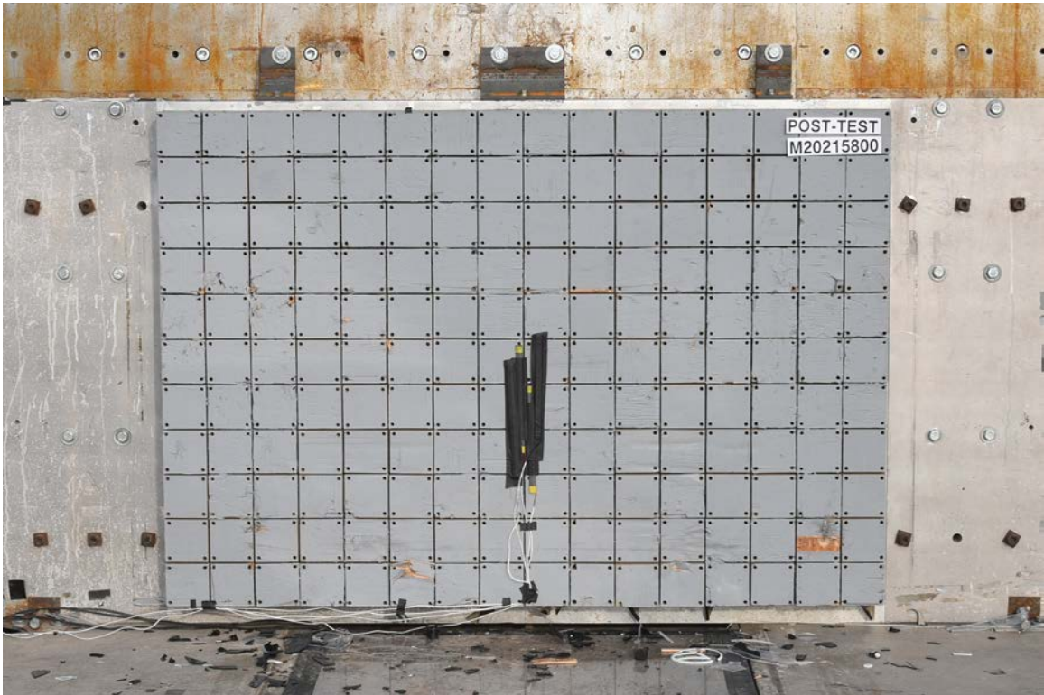
FIGURE 3. Post-Test Load Cell Wall
