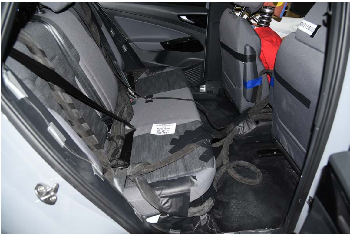
FIGURE 28. Pre-Test Dummy Cable Routing
