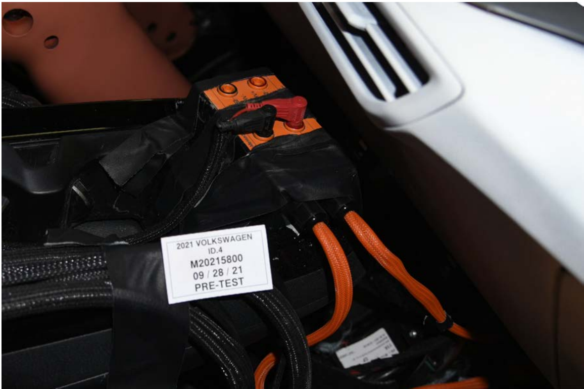
FIGURE 305-022. Pre-Impact View of High Voltage Leads Attached
