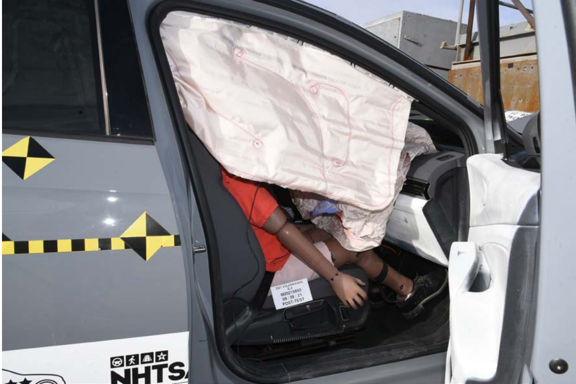
FIGURE 58. Post-Test Passenger Dummy and Vehicle Interior View
