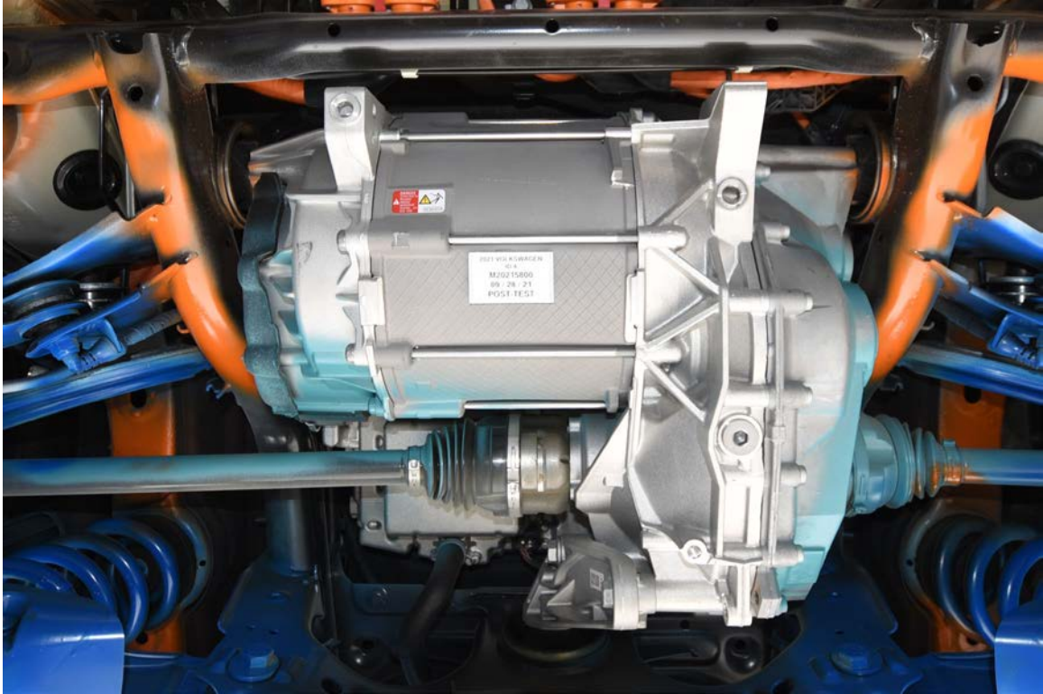
FIGURE 305-017. Post-Impact View of Electric Propulsion Drive
