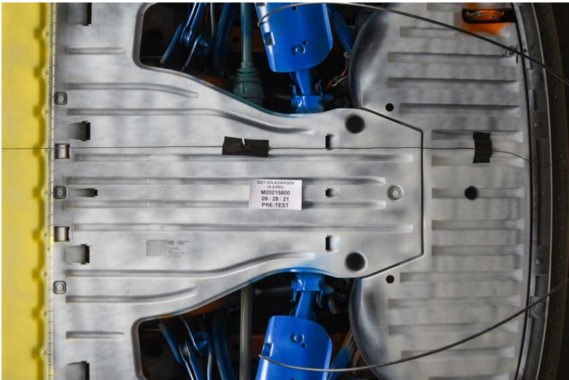
FIGURE 305-016. Pre-Impact View of Electric Propulsion Drive
