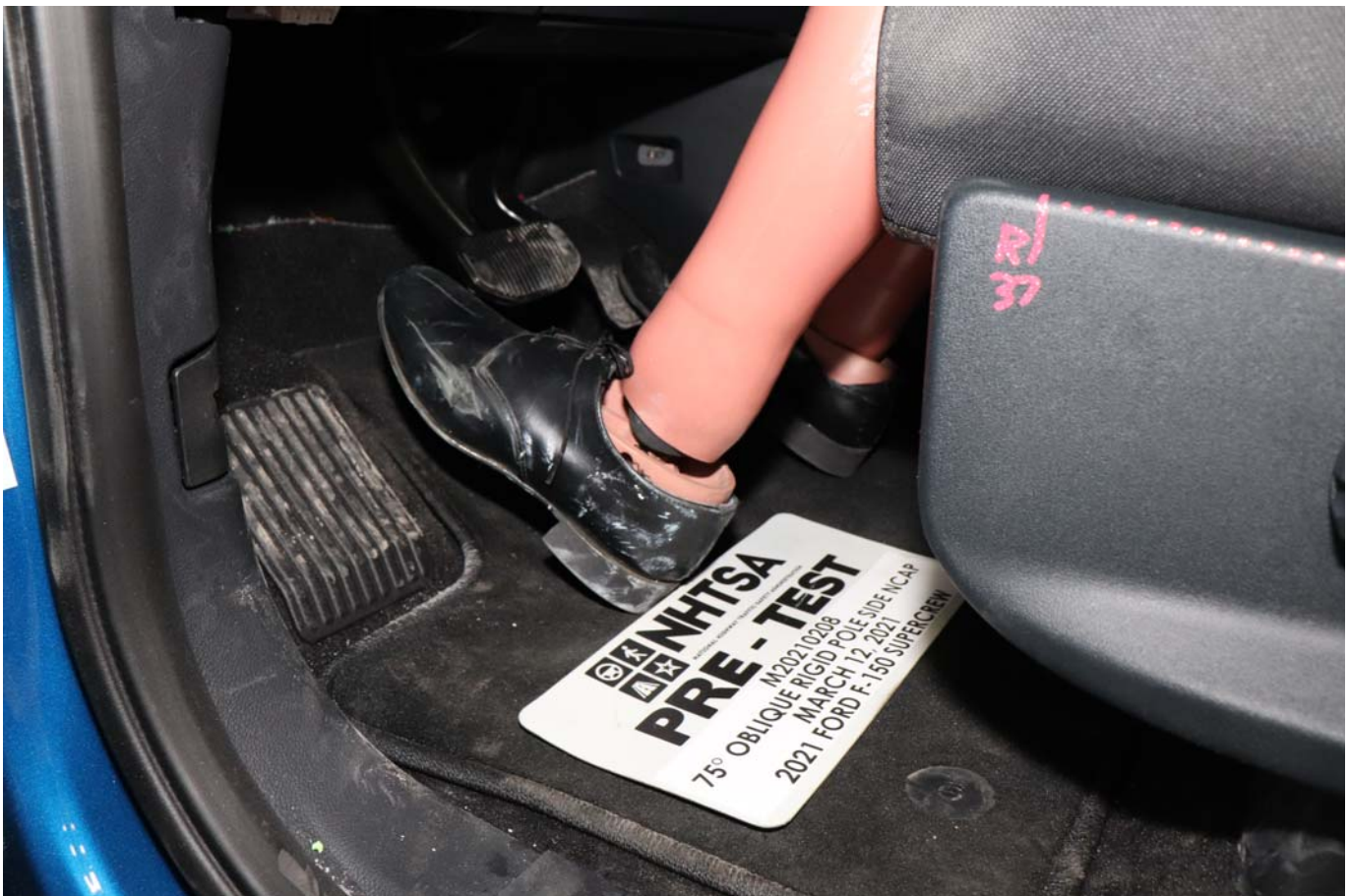
Photo No. 032 - Pre-Test Placement of Dummy Feet
