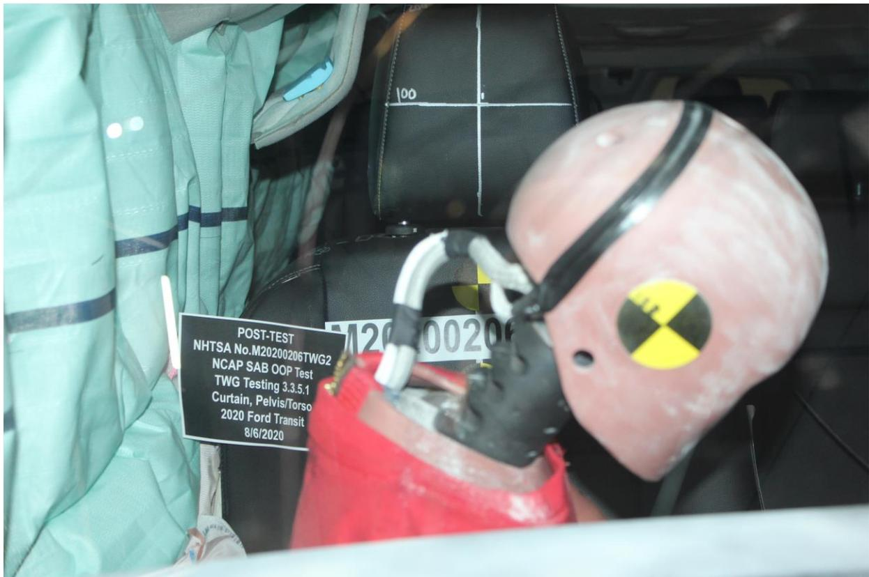
**Figure A-20: Post-Test Dummy Front Close-up View**
