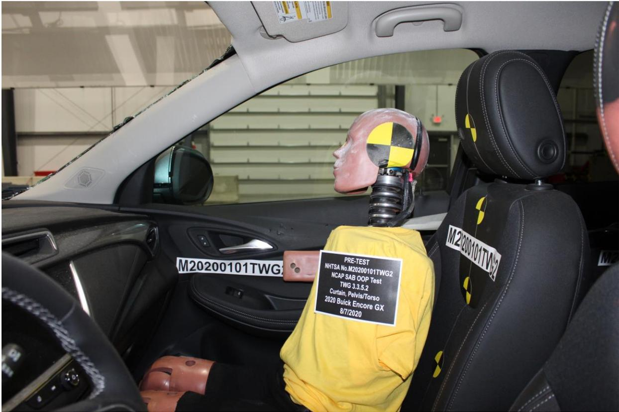
**Figure A-9: Pre-Test Dummy Left Side View**
