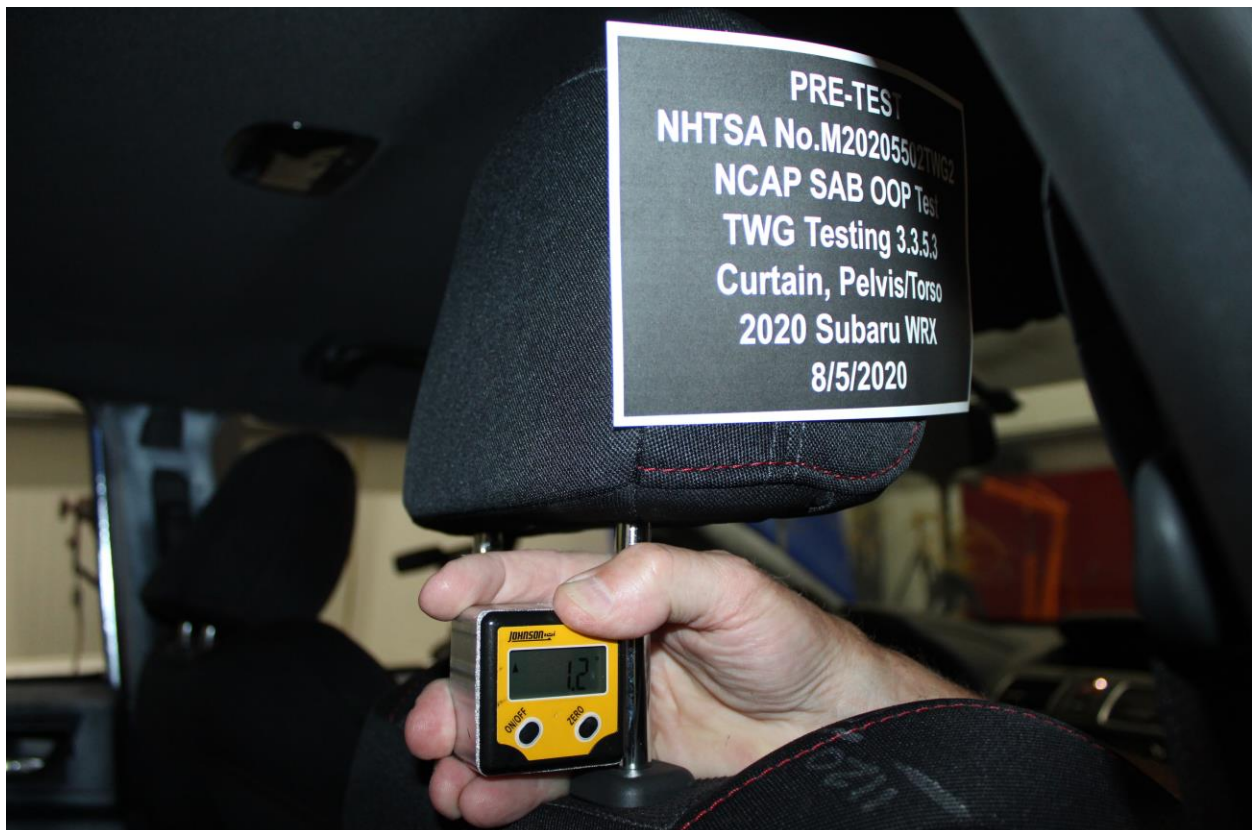
Figure A-8: Pre-Test Vehicle Seat Back Angle
