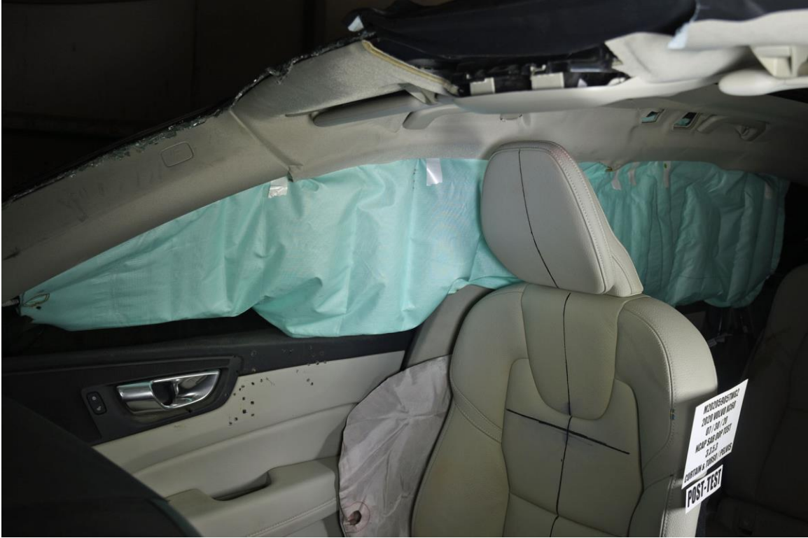
FIGURE 27. Post-Test Curtain Air Bag Front Left ¾ View
