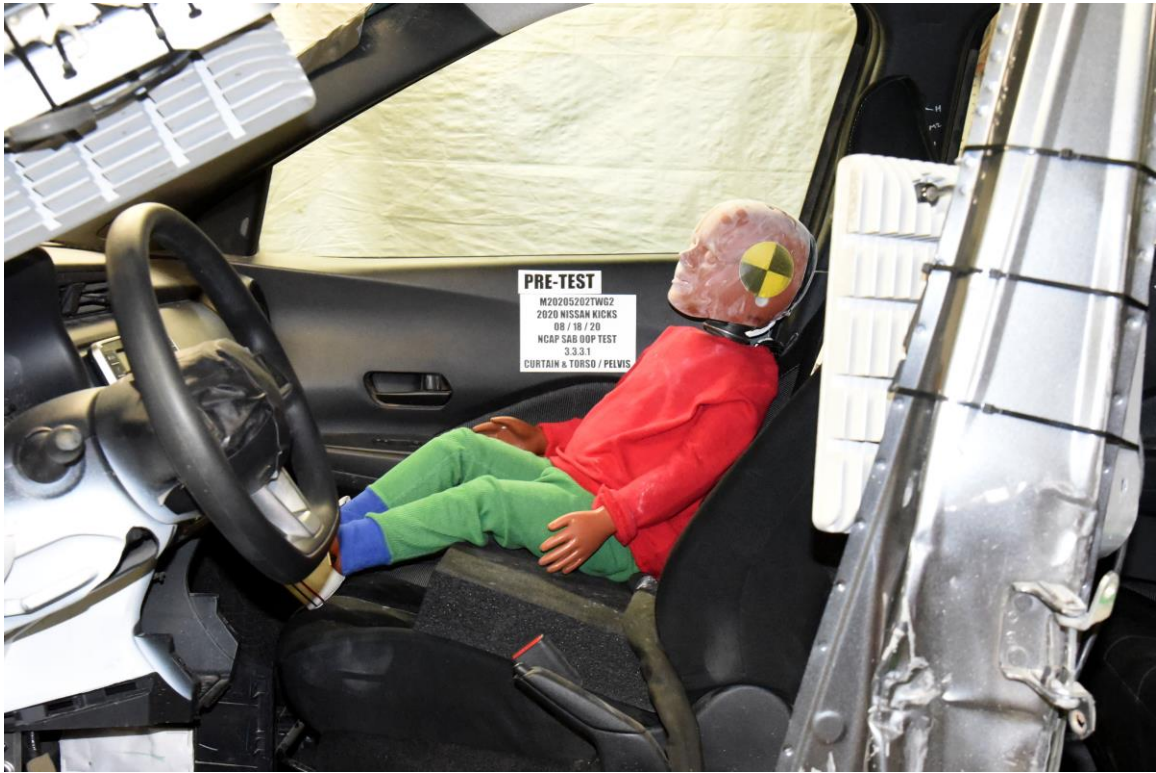
FIGURE 9. Pre-Test Dummy Left Side View
