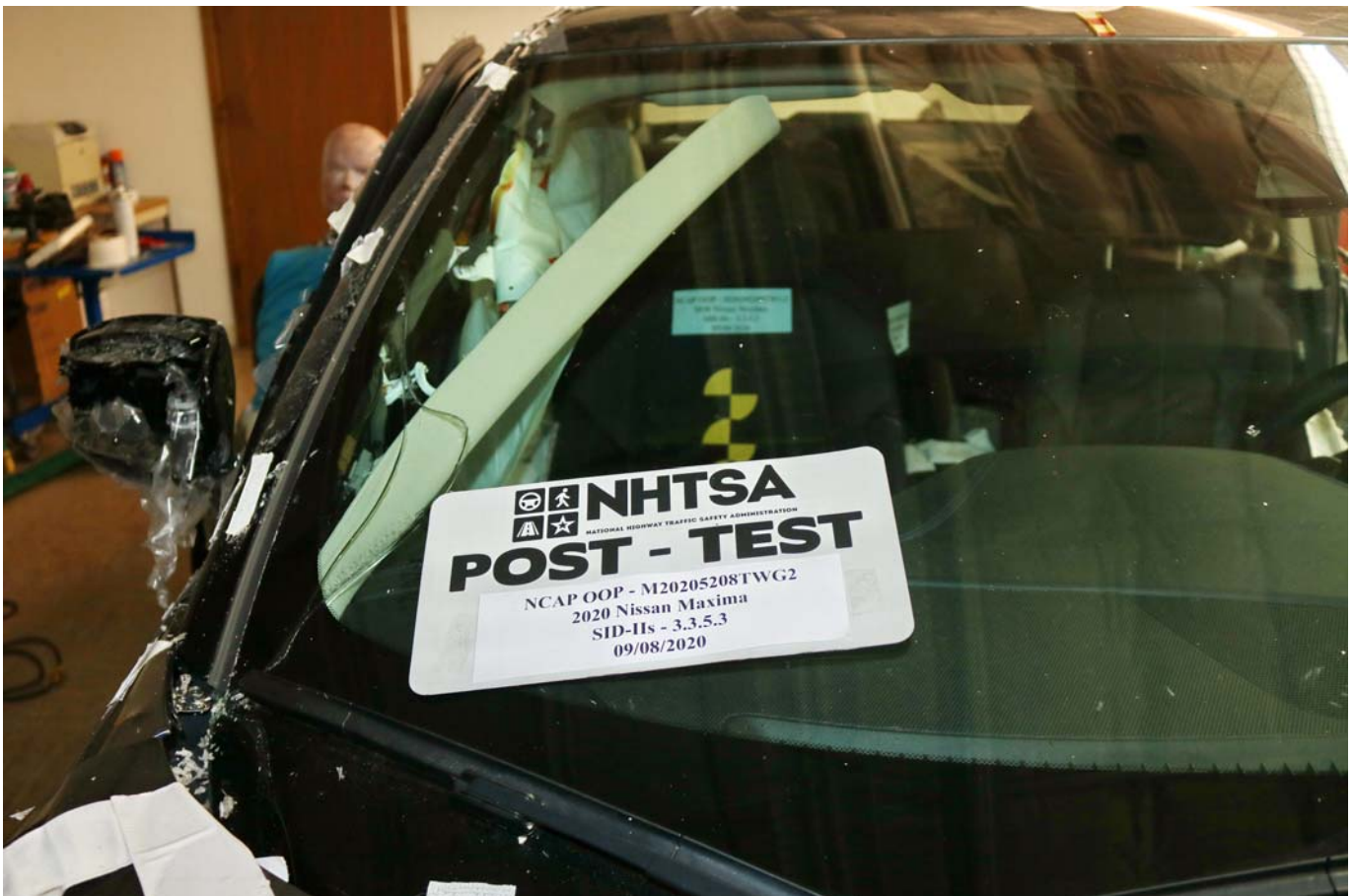
Photo No. 024 - Post-Test Curtain Airbag Front View
