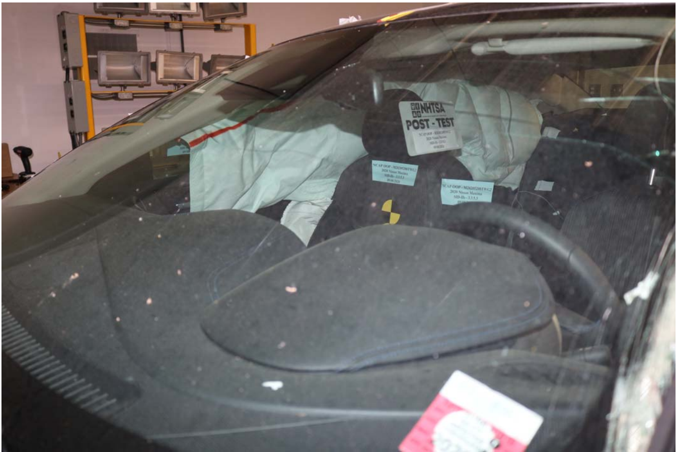
Photo No. 023 - Post-Test Curtain Airbag Left Three-Quarter Front View
