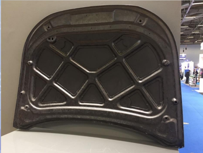
Hood inner panel via compression molding
