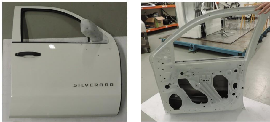
Figure 157: Baseline Front Door Frame
