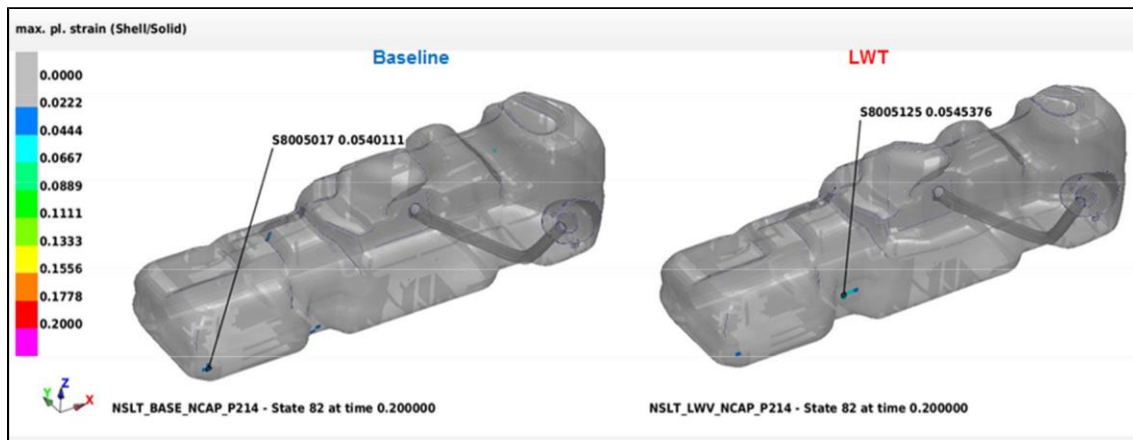
Figure 330: NCAP Side Rigid Pole – Post-Crash Comparison Test Versus CAE Baseline and LWT
