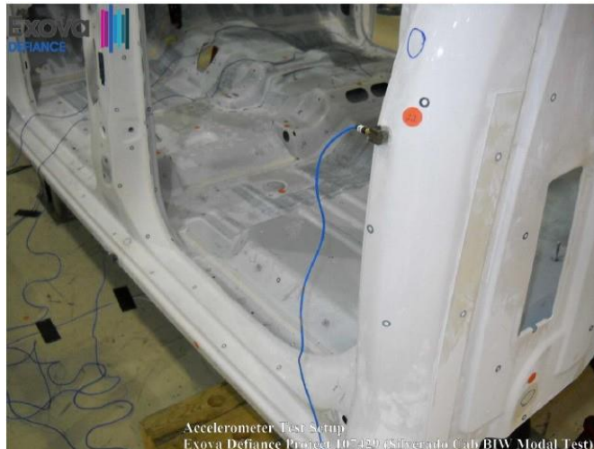
Figure 101: 2014 Silverado 1500 With Tri-Axial Accelerometer for Cab Modal Testing 55
