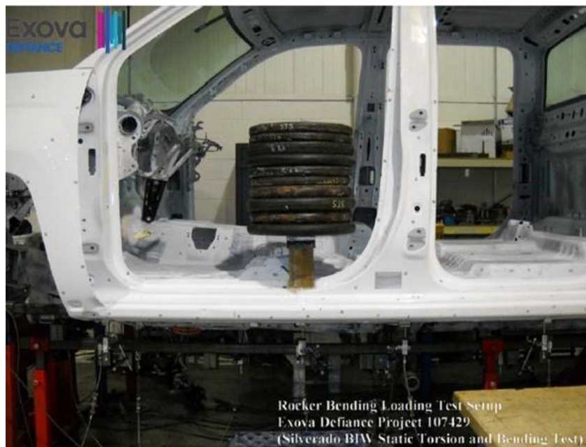
Figure 110: 2014 Silverado Sill Loaded Bending Test
