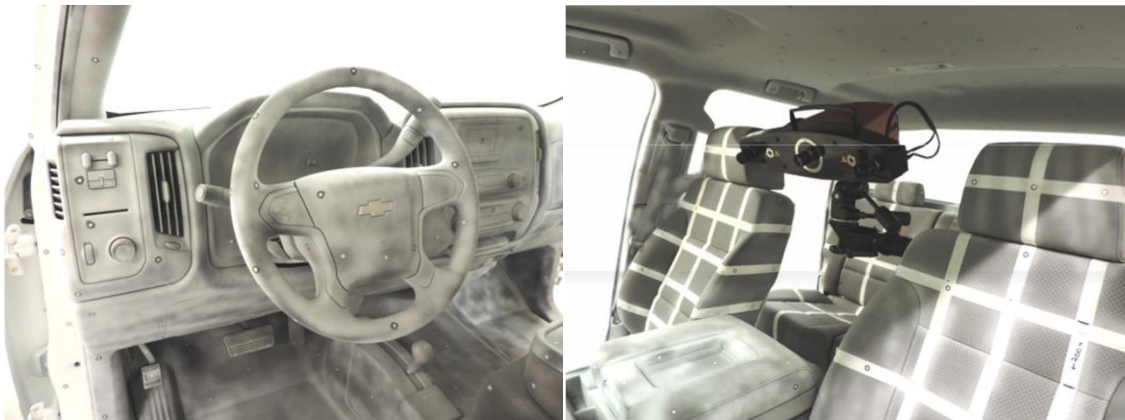
Figure 17: Silverado 1500 Interior Prepared for White Light Scanning
