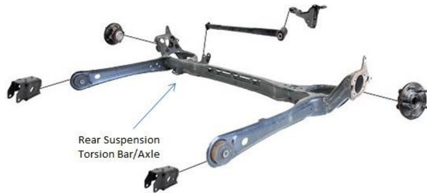
Figure 540: Chrysler Town & Country rear suspension showing torsion bar/axle 212
