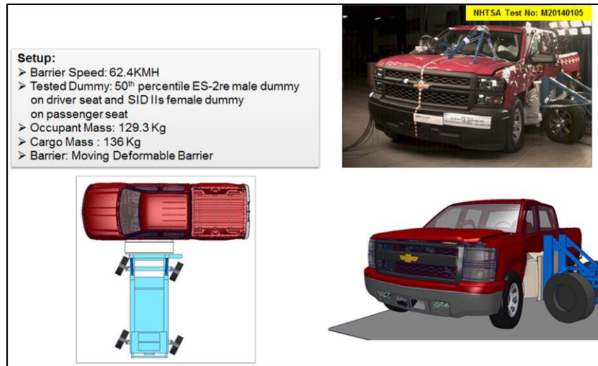
Figure 315: NCAP Side MDB - Test and LS-DYNA Model set up
