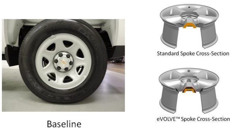
Figure 478: Baseline Wheels Versus LWT Wheels
