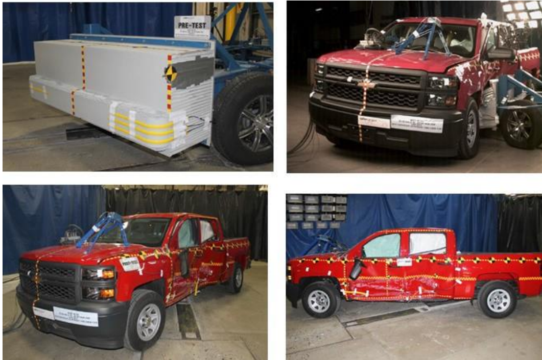
Figure 71: MDB and Post-Test Vehicle 2014 Silverado 1500 NCAP Side Impact Test (NHTSA Report SINCAP-MGA-2014-007)
