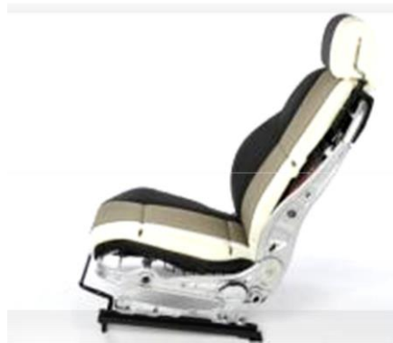
Figure 246: The Evolution Seat by Lear Corporation ( http://articles.sae.org/8268/ )
