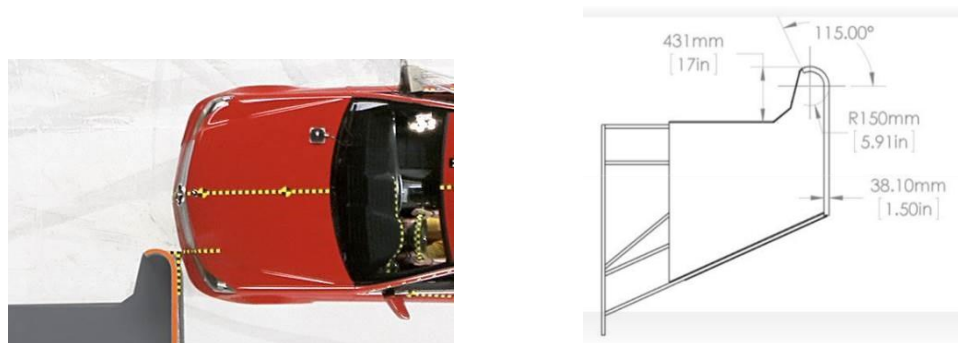
Figure 96: Configuration of the IIHS small overlap frontal barrier test
