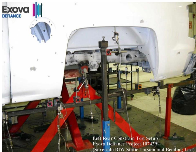
Figure 107: 2014 Silverado 1500 Left Rear Constraint for Static Bending and Torsion Testing
