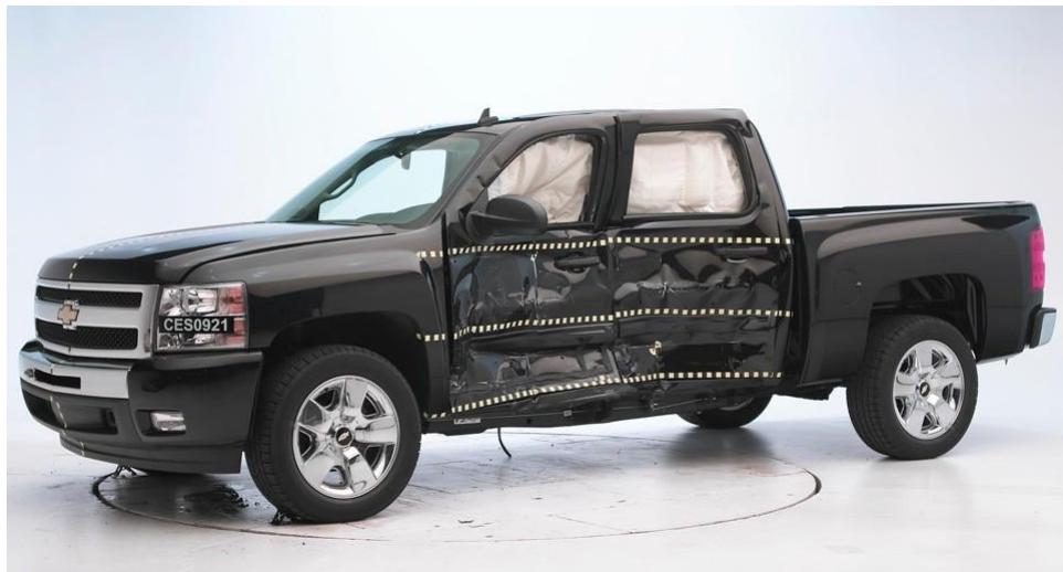
Figure 89: 2010 Chevrolet Silverado 1500 Following IIHS Side Impact Test
