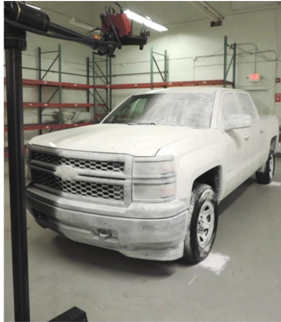
Figure 16: Silverado 1500 Exterior Prepared for White Light Scanning
