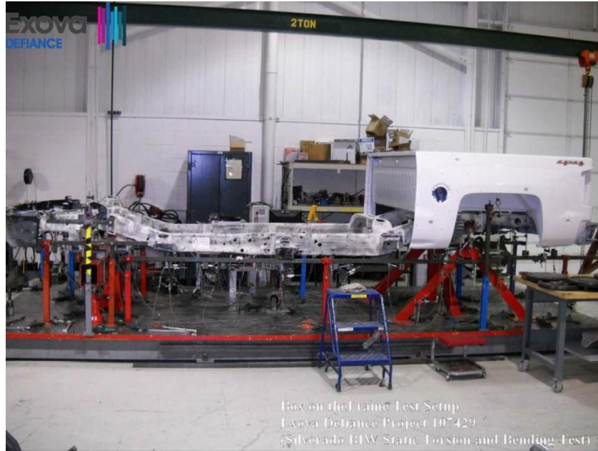
Figure 106: 2014 Silverado 1500 Set-Up for Static Bending and Torsion Testing of Frame With Pickup Box
