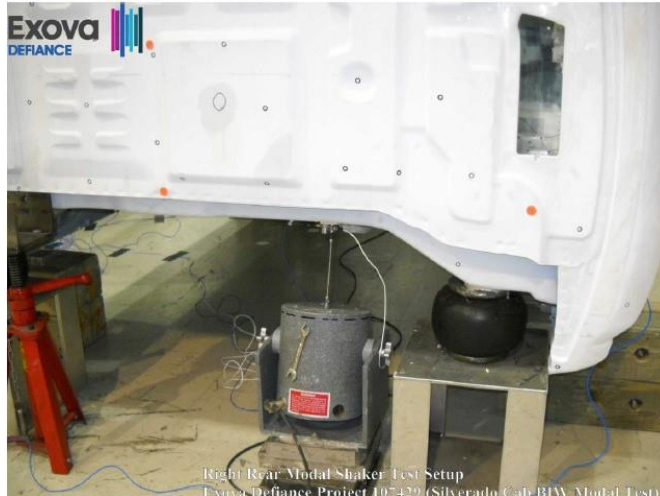
Figure 100: 2014 Silverado With Shaker and Air bag Support for Cab Modal Testing
