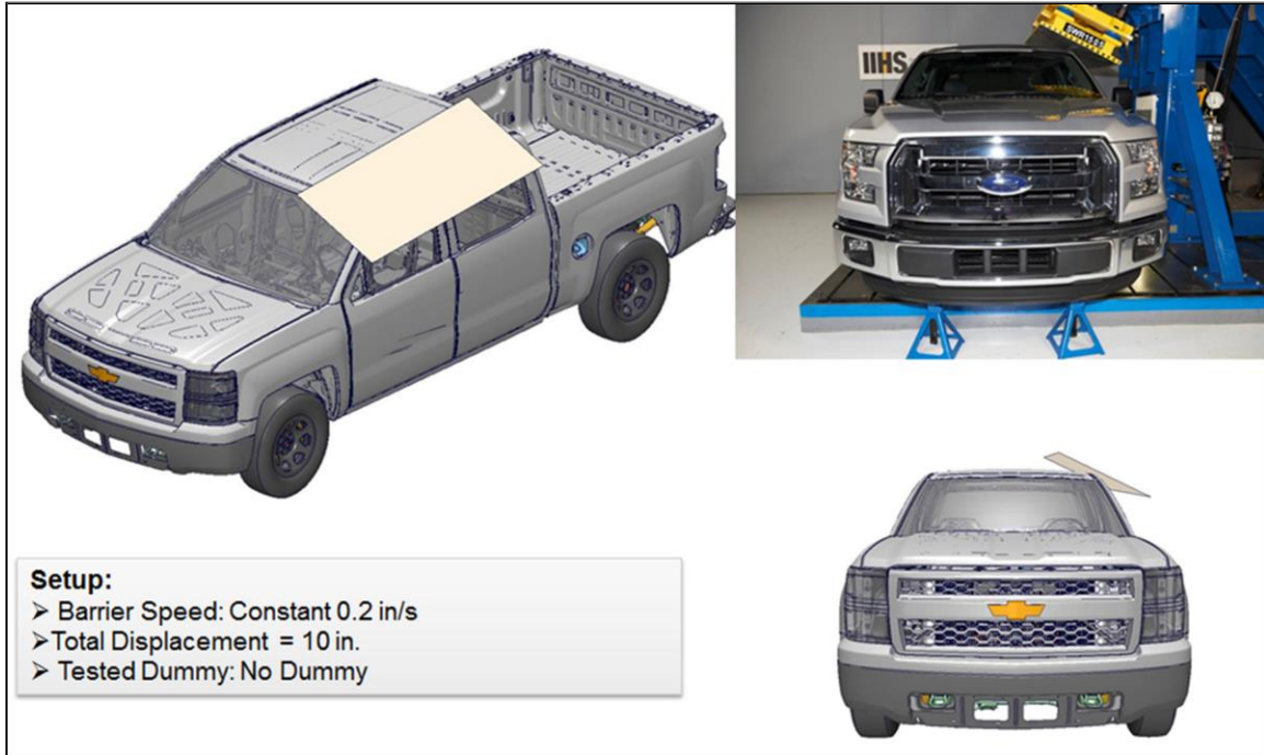
Figure 331: IIHS Roof Strength Test - LS-DYNA Model Setup
