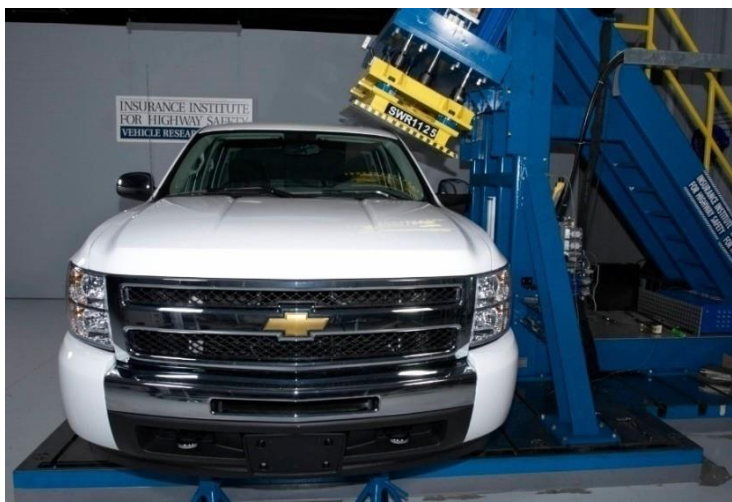
Figure 81: 2011 Chevrolet Silverado in IIHS Roof Strength Test Fixture
