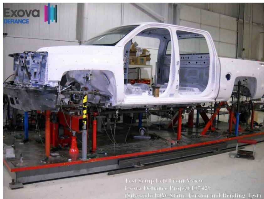
Figure 105: 2014 Silverado 1500 Set-Up for Static Bending and Torsion Testing of Frame, Cab, and Pickup Box
