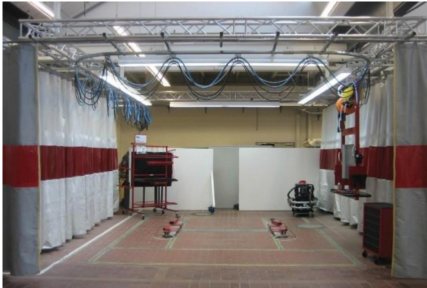
Figure 396: Dedicated Screened Aluminum Clean Room Repair Area
