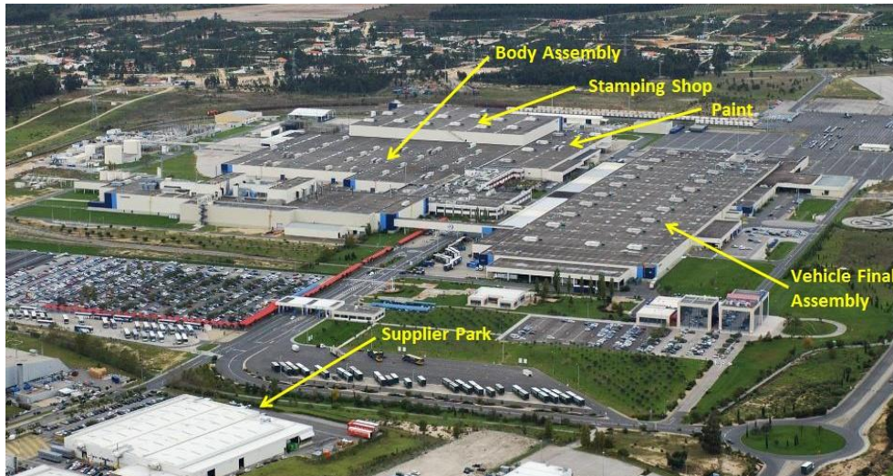
Figure 408: Integrated Vehicle Assembly Facility "Greenfield" Site
