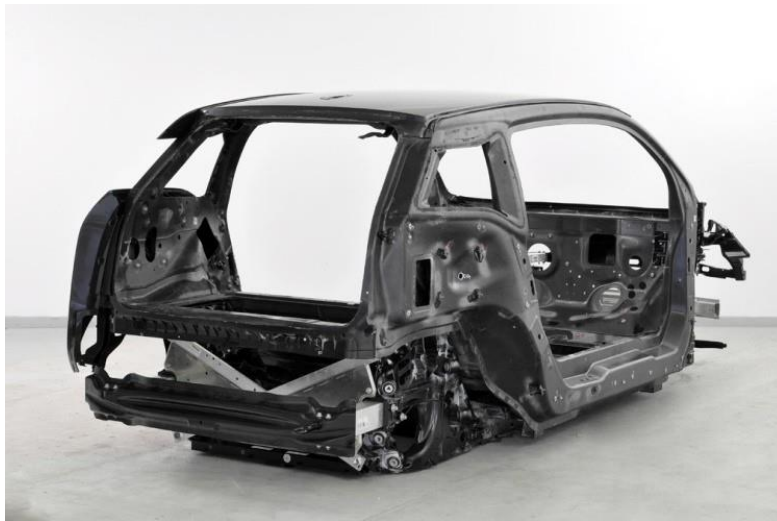
Figure 131: 2014 BMW i3 – Composite and Aluminum Structure 94
