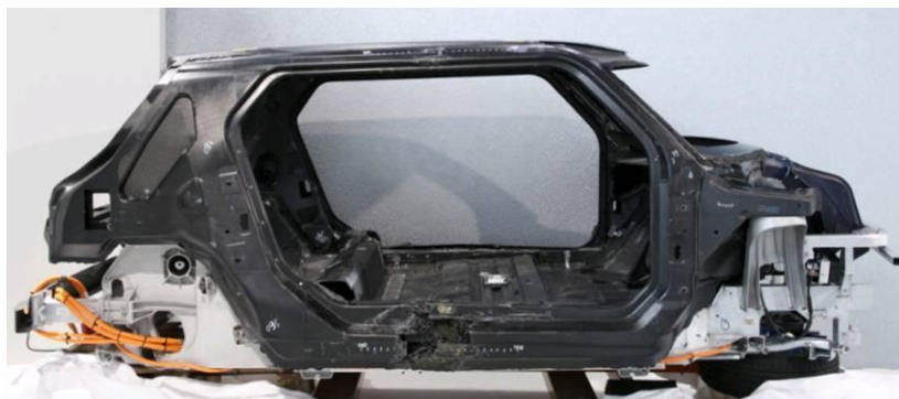
Figure 151: BMW i3 – Composite and Aluminum Structure – Production Year 2013
