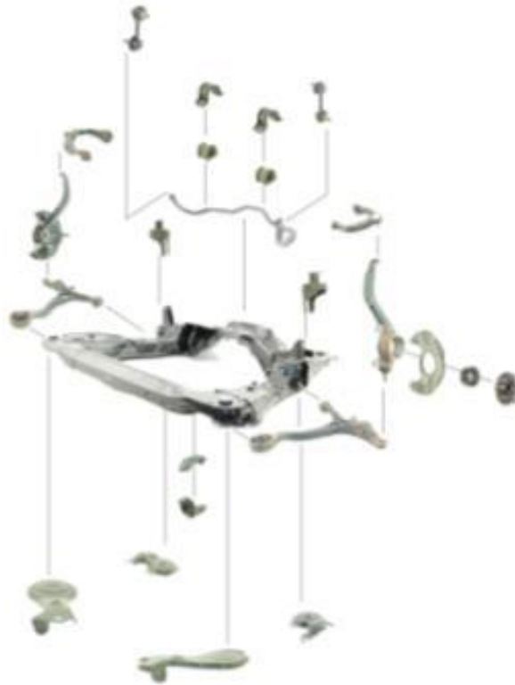
Figure 29: Components That Make Up the Front Suspension Module 31
