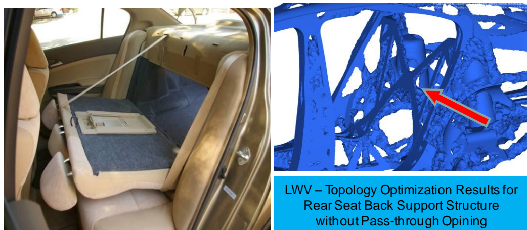
Figure 93: Topology Optimization Results – Rear Seat Back
