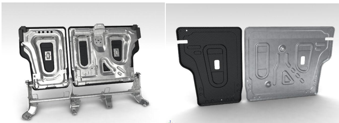
Figure 226: Fiber-Reinforced Composite Rear Seat Back (JCI) 157
