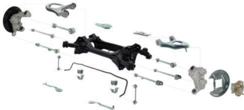
Figure 32: Components That Make Up the Rear Suspension Module 34
