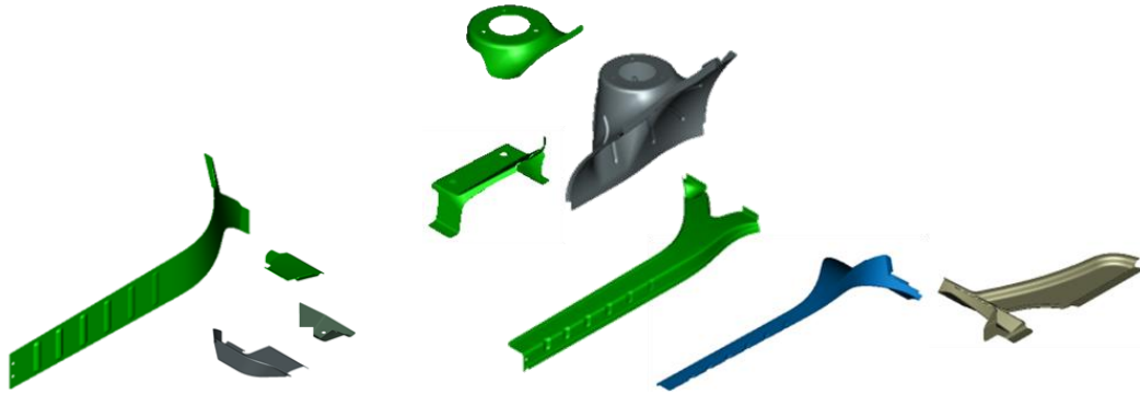
Figure 494: Front rail inner (left) and outer (right) subassembly
