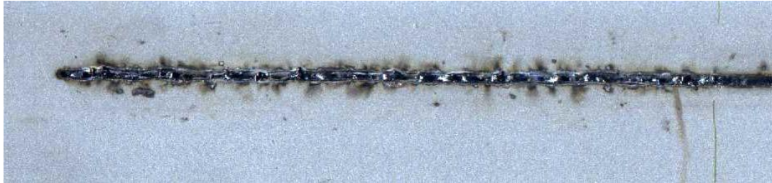
Figure 475: Splatter on surface caused by Zinc coating vapour blowout – Zero Gap between the welded panels 238
