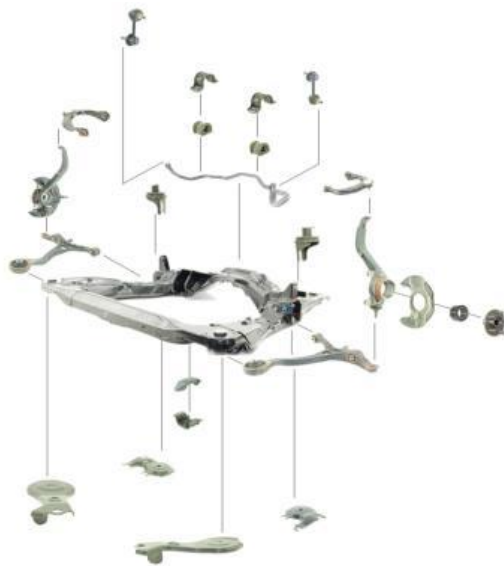
Figure 196: Baseline Front Suspension Exploded View 141
