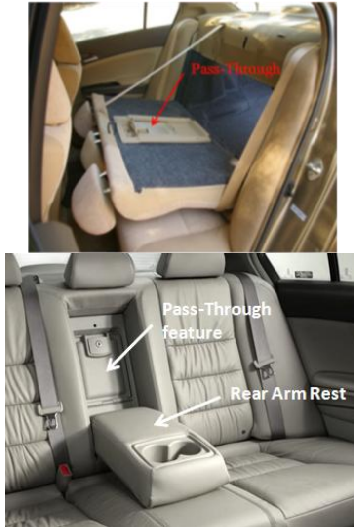
Figure 38: Rear Seat with Pass-Through Feature 45
