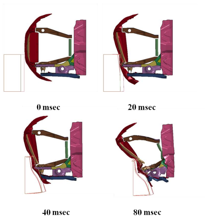
Figure 313: Crush of LWV five key structural parts over the time of the IIHS frontal offset test
