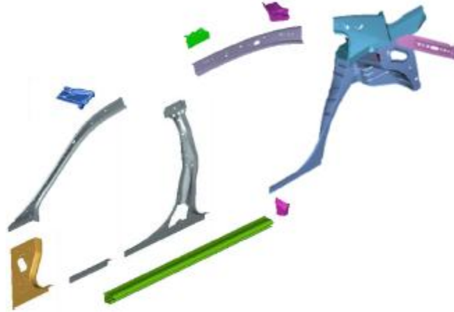
Figure 510: Inner body side inner subassembly of the laser welded structure
