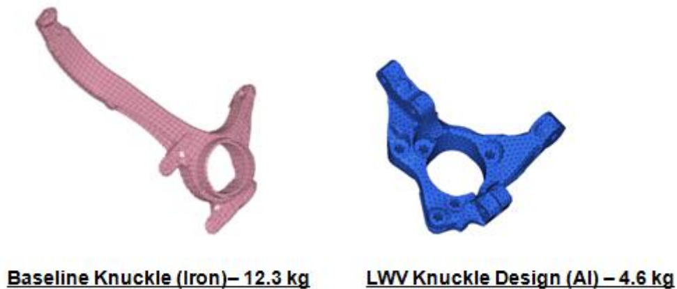
Figure 202: Steering Knuckle – Baseline and LWV Design
