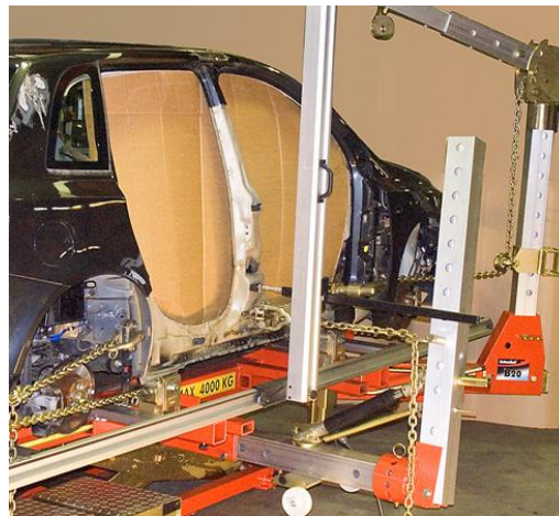
Figure 136: Straightening of a b-pillar in a repair rig
