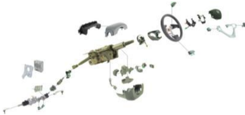
Figure 27: Components That Make Up the Steering Subsystem 29
