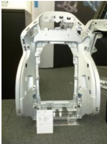
Figure 224: Magnesium Seat Back – Mercedes Benz SLZ (Lear)
