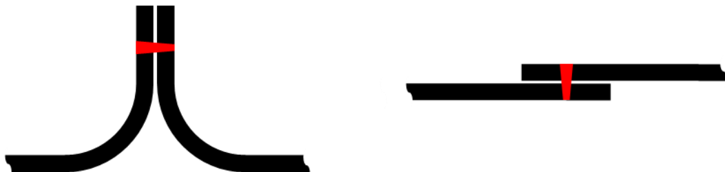
Figure 483: Schematic representation of a flange weld (left) and a lap joint weld (right)
