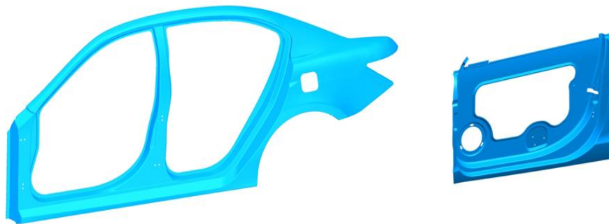
Figure 334: Typical parts, Body Side outer panel and Door Inner panel that would be stamped using a transfer press line.
