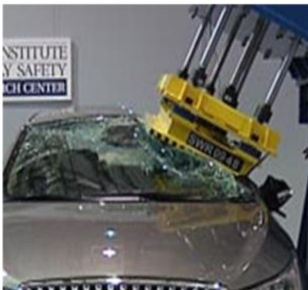
Figure 68: Test set up for IIHS roof crush test 80
