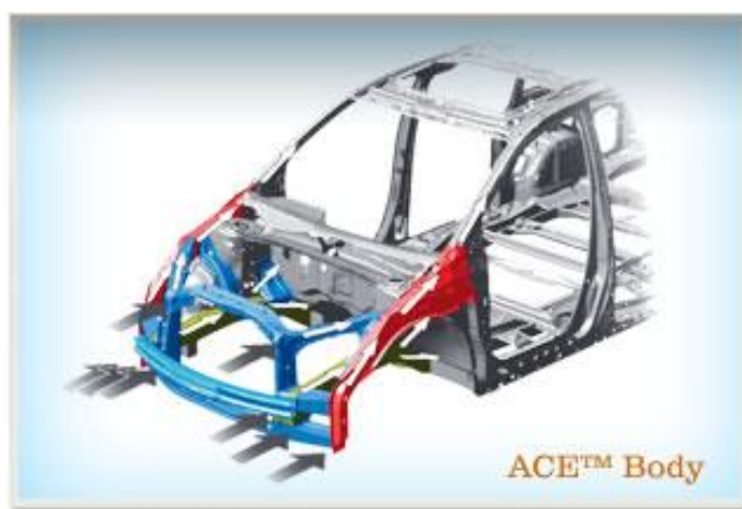
Figure 51: ACE improved body structure 54
