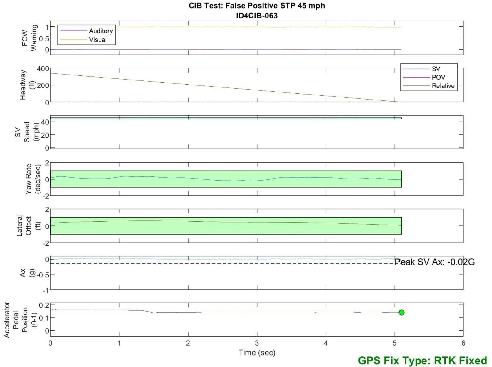
Figure D50. Time History for CIB Run 63, SV Encounters Steel Trench Plate, SV 45 mph
