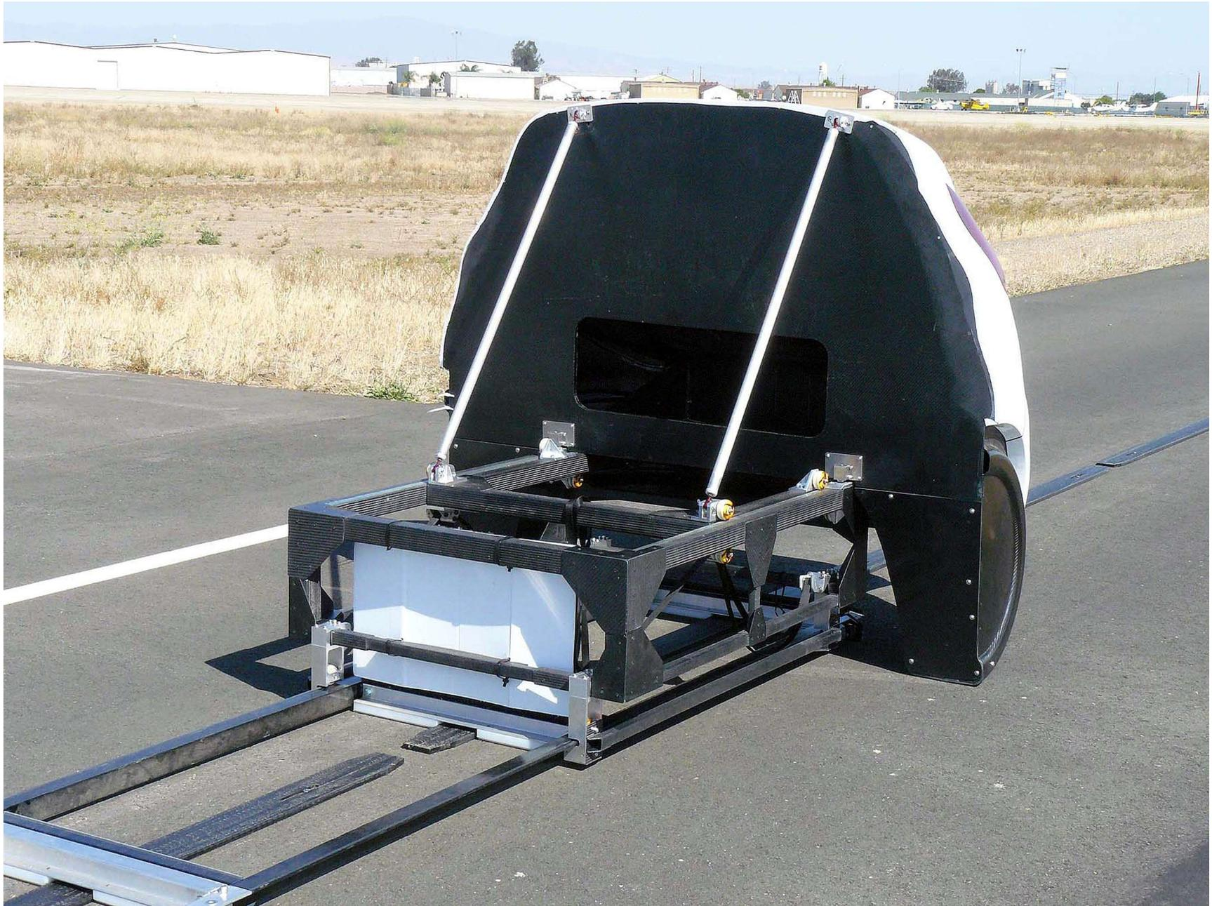
Figure A7. Load Frame/Slider of SSV
