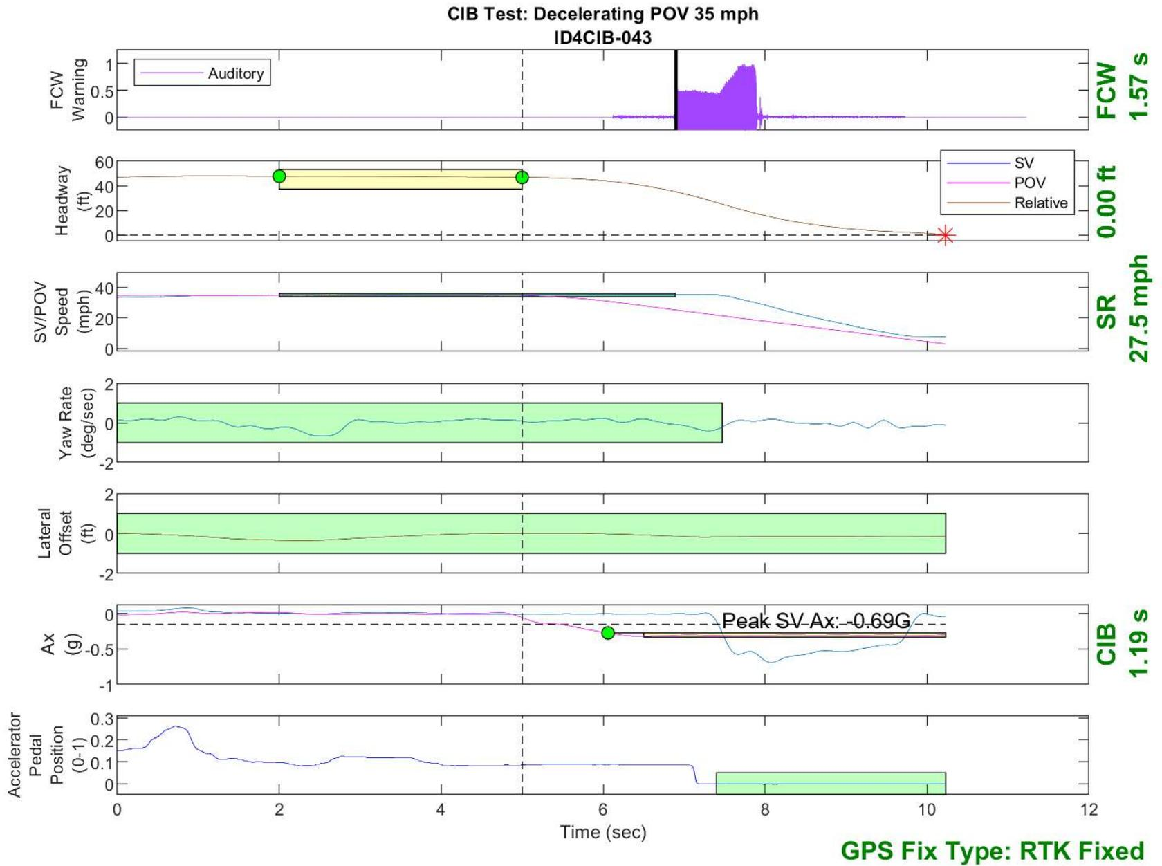
Figure D33. Time History for CIB Run 43, SV Encounters Decelerating POV, SV 35 mph, POV 35 mph
