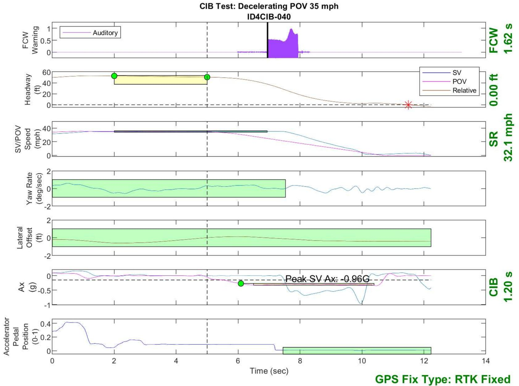
Figure D31. Time History for CIB Run 40, SV Encounters Decelerating POV, SV 35 mph, POV 35 mph
