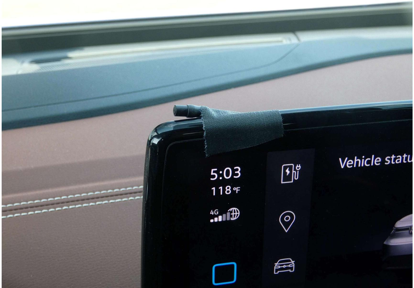
Figure A11. Sensor for Detecting Auditory Alert
