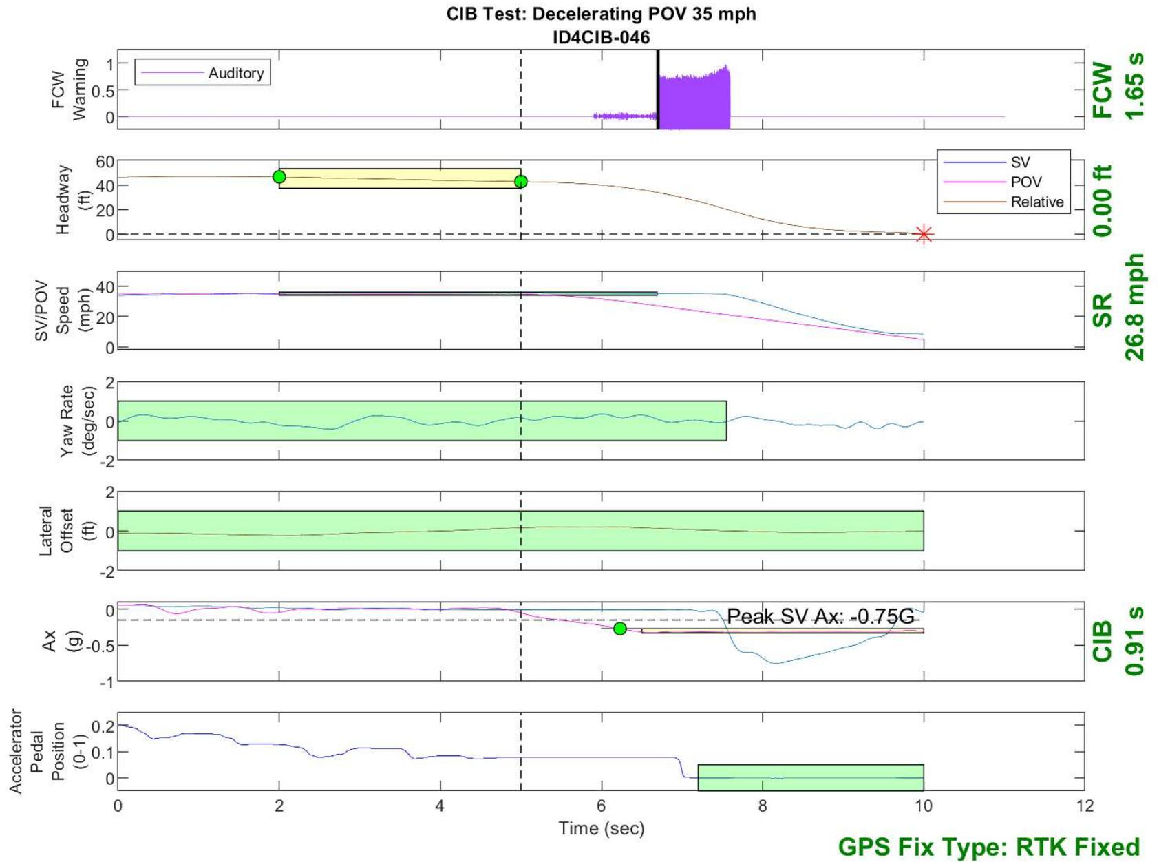
Figure D36. Time History for CIB Run 46, SV Encounters Decelerating POV, SV 35 mph, POV 35 mph
