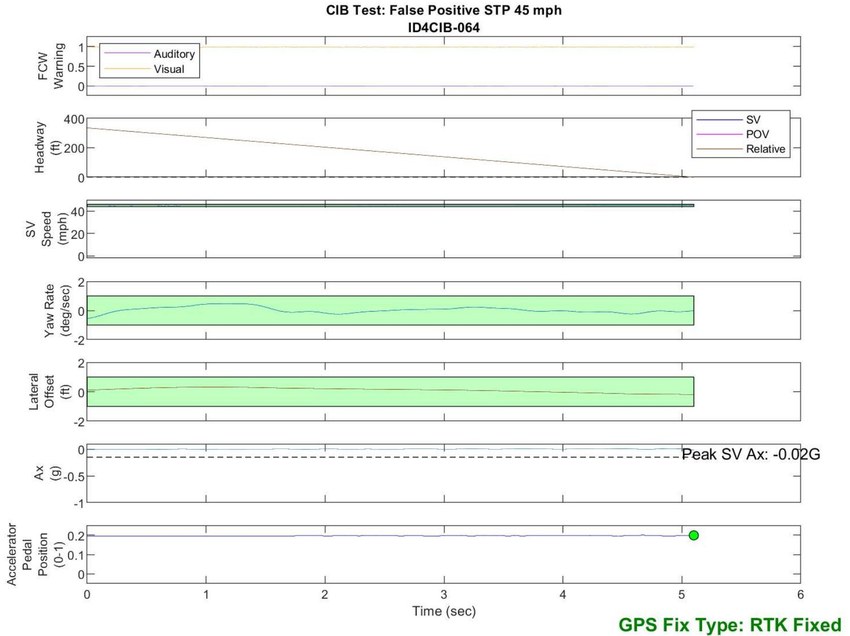
Figure D51. Time History for CIB Run 64, SV Encounters Steel Trench Plate, SV 45 mph
