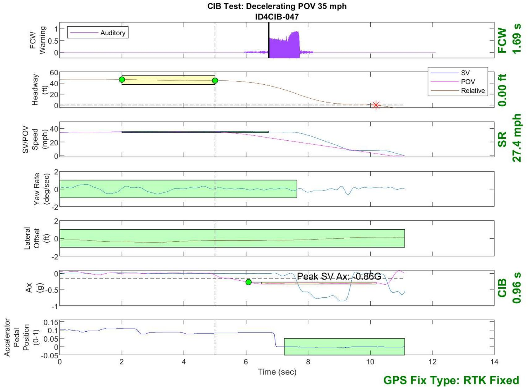
Figure D37. Time History for CIB Run 47, SV Encounters Decelerating POV, SV 35 mph, POV 35 mph
