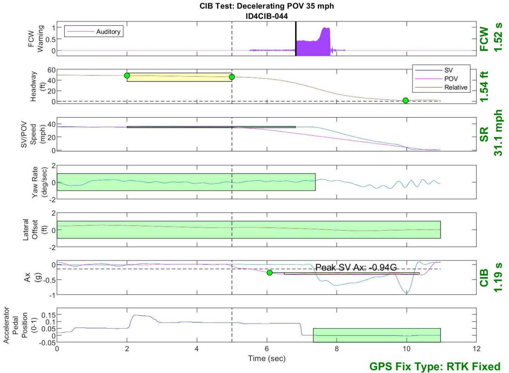
Figure D34. Time History for CIB Run 44, SV Encounters Decelerating POV, SV 35 mph, POV 35 mph
