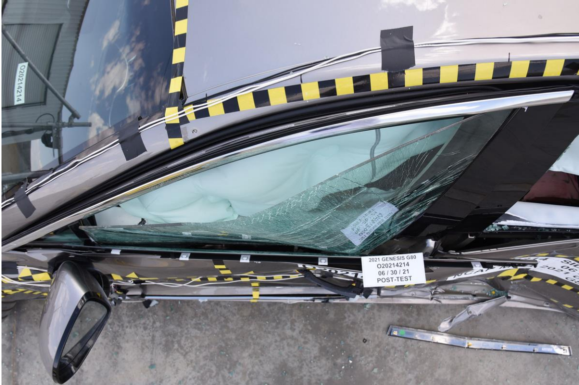
FIGURE 43. Post-Test Driver Dummy and Door Clearance View
