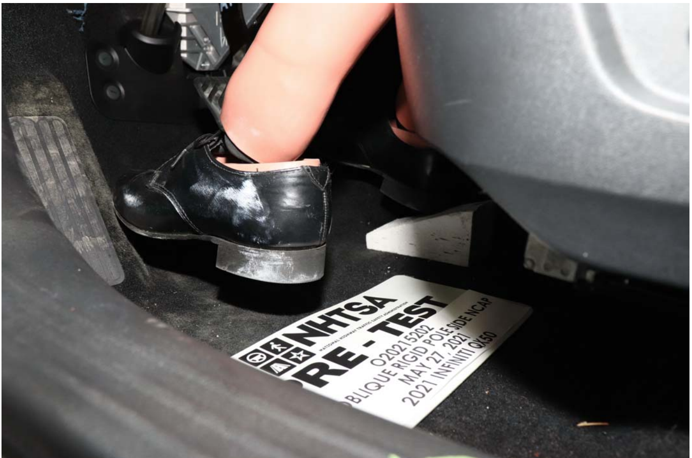
Photo No. 032 - Pre-Test Placement of Dummy Feet
