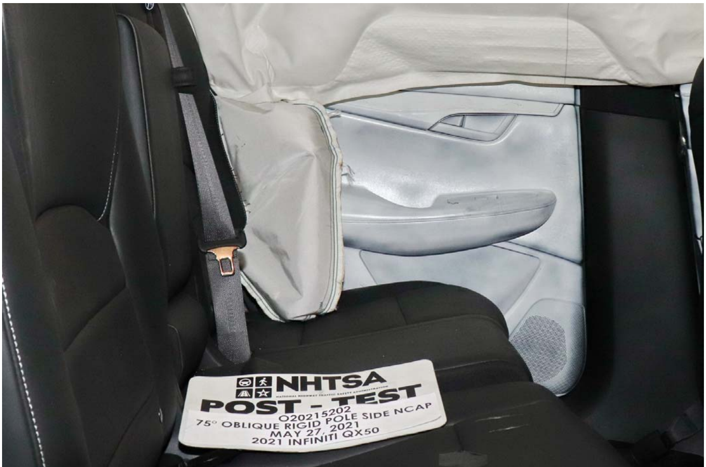
Photo No. 054 - Post-Test Inner Rear Passenger Torso Air Bag Deployment View
