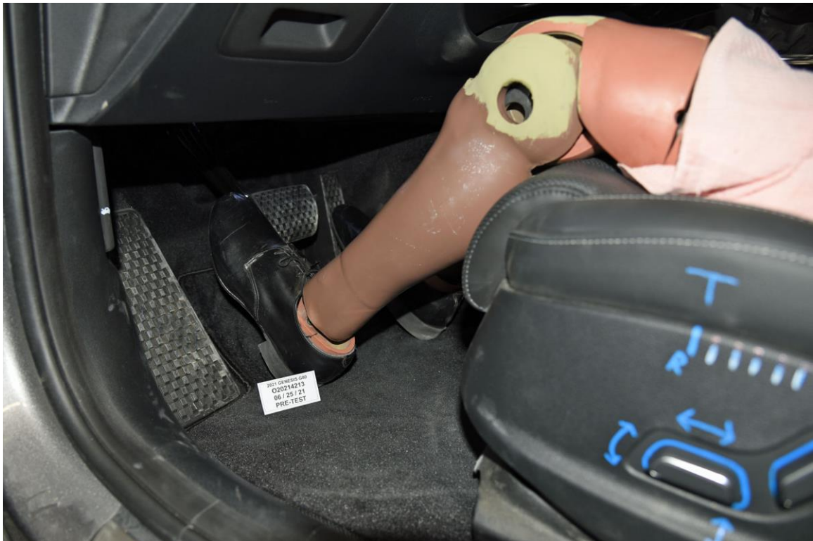
FIGURE 32. Pre-Test Placement of Dummy's Feet
