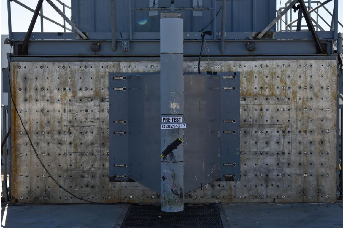
FIGURE 59. Pre-Test Pole Barrier Front View
