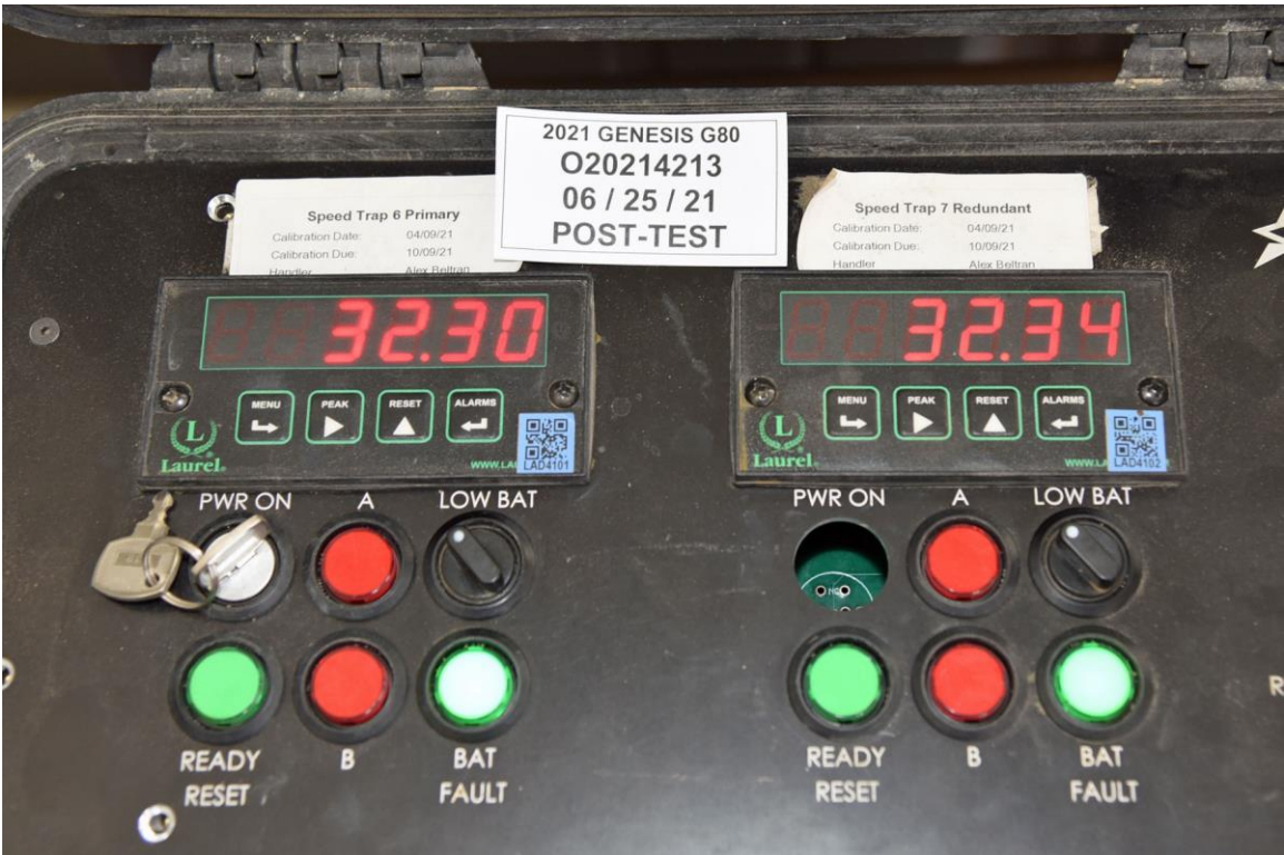
FIGURE 64. Post-Test Primary and Redundant Speed Trap Read-Out
