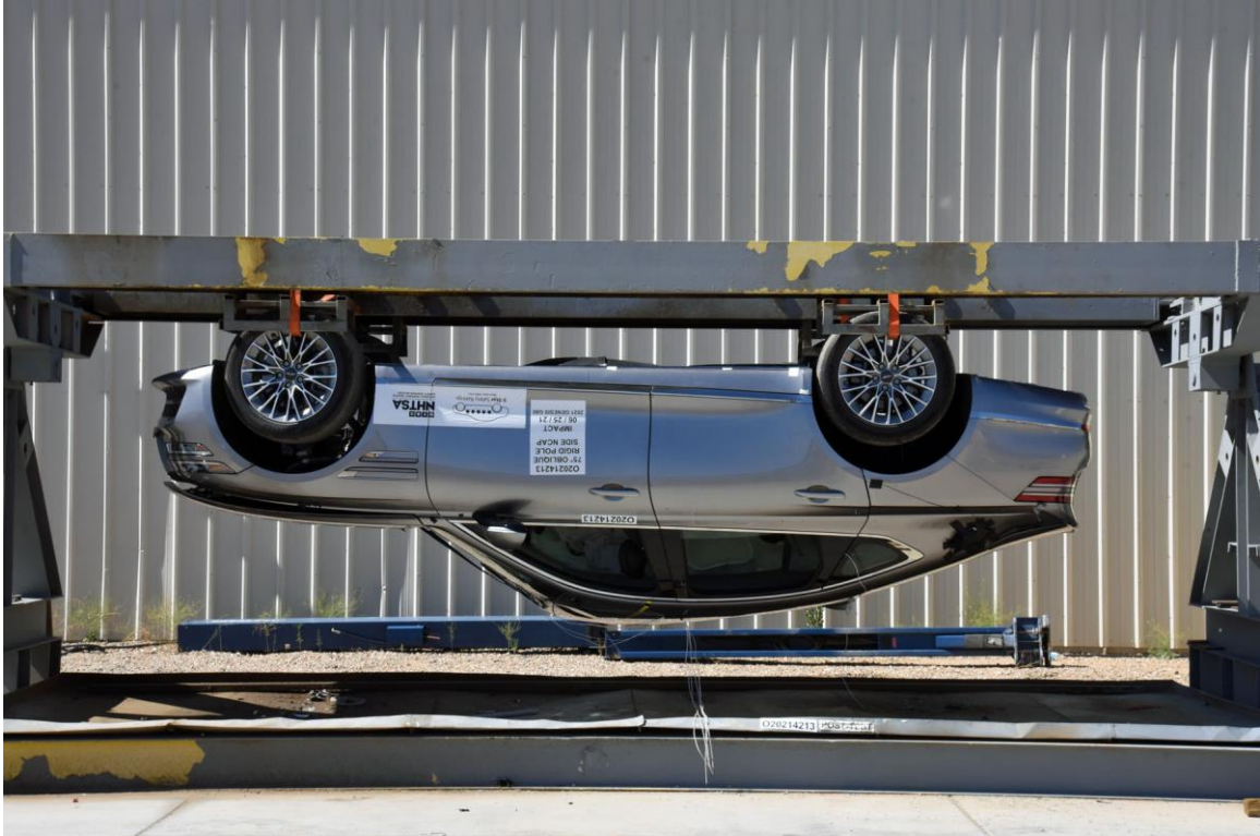
FIGURE 67. FMVSS No. 301 Static Rollover 180 Degrees
