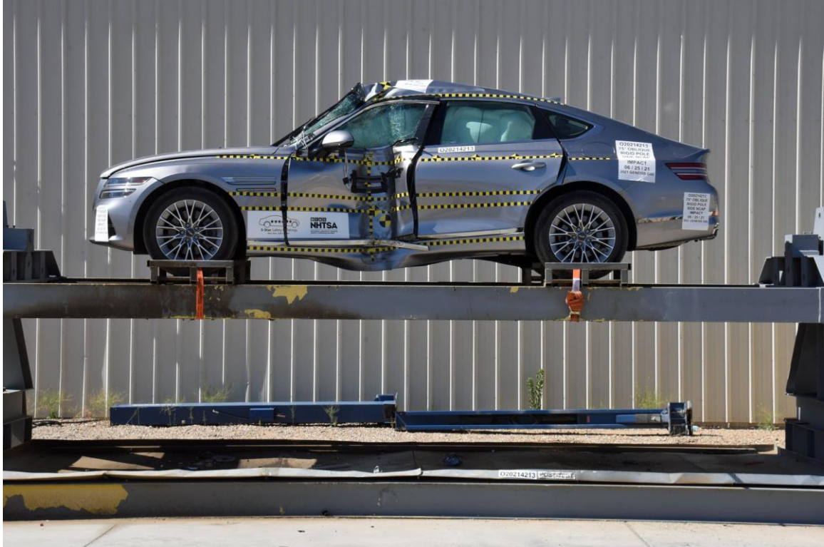
FIGURE 65. FMVSS No. 301 Static Rollover 0 Degrees
