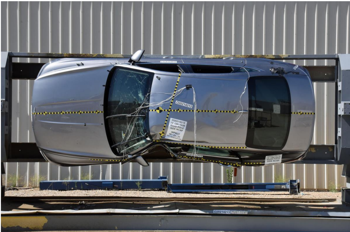
FIGURE 66. FMVSS No. 301 Static Rollover 90 Degrees
