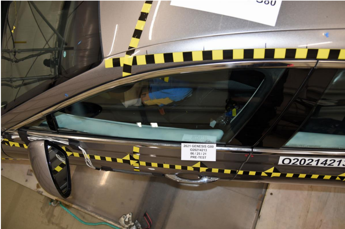
FIGURE 40. Pre-Test Dummy and Door Clearance View
