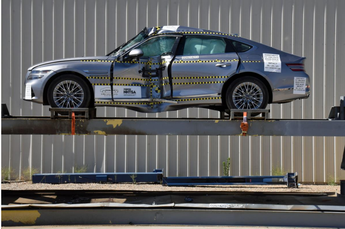
FIGURE 69. FMVSS No. 301 Static Rollover 360 Degrees
