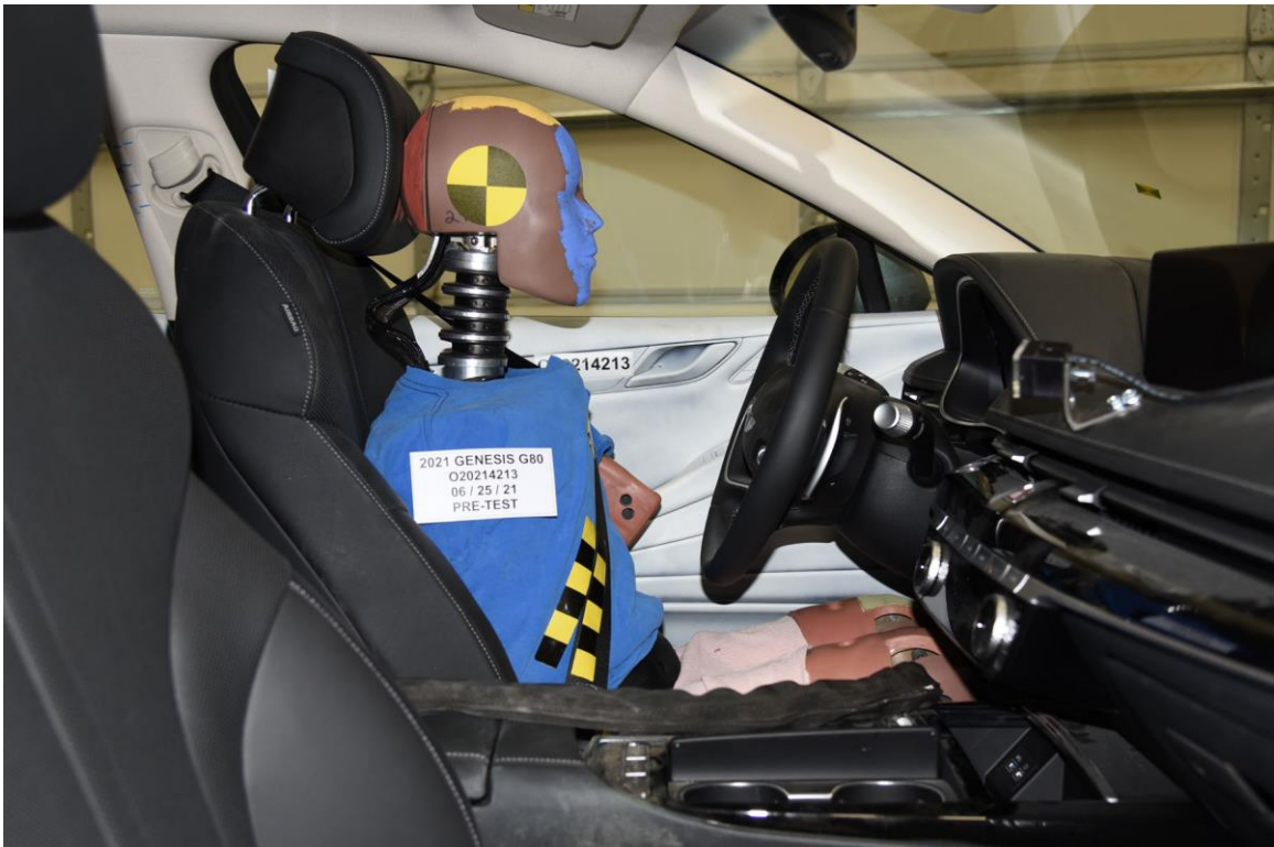
FIGURE 42. Pre-Test Right Side View of Dummy and Front Seat of Occupant Compartment
