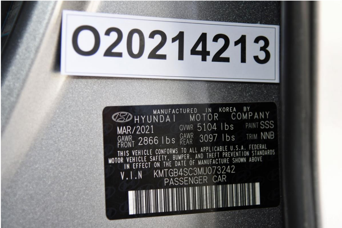
FIGURE 57. Close-Up View of Vehicle's Certification Label
