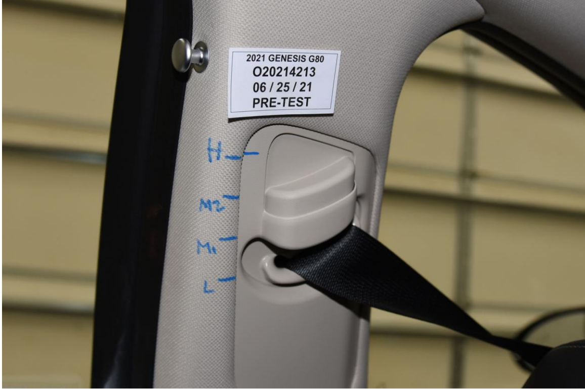
FIGURE 33. Pre-Test View of Belt Anchorage for Dummy
