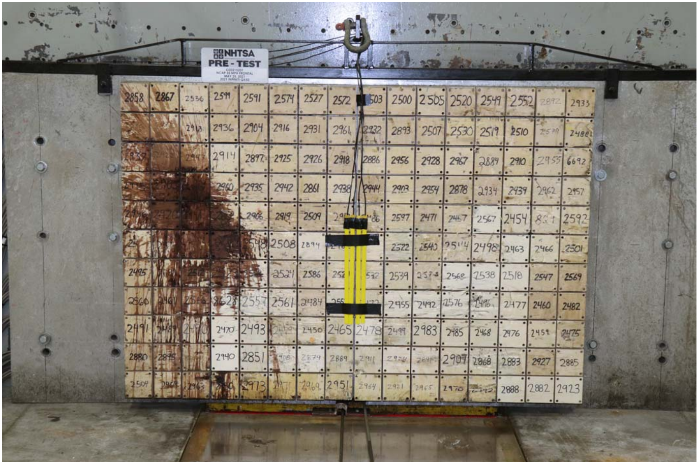
Photo No. 002 - Pre-Test Load Cell Wall
