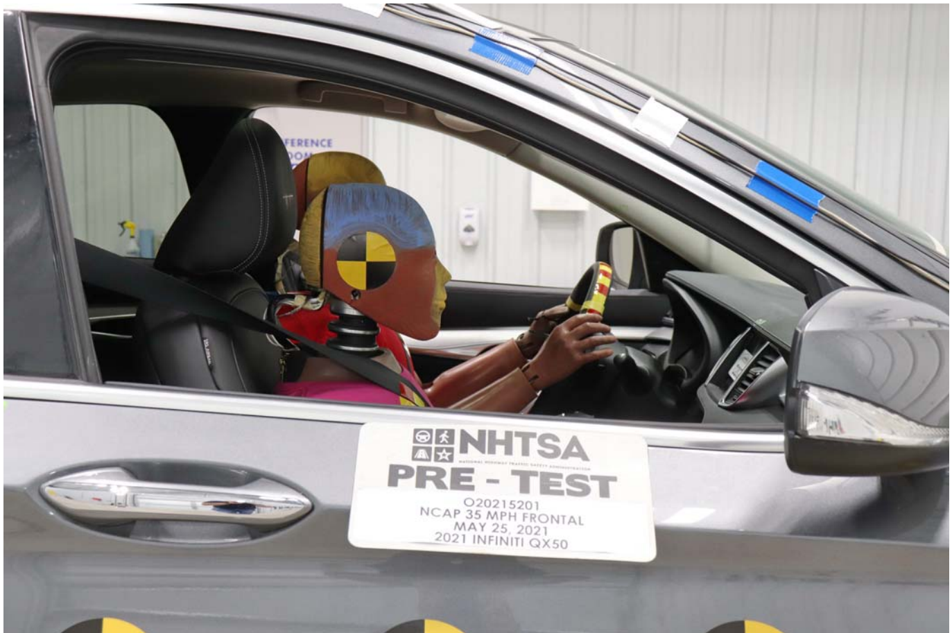
Photo No. 055 - Pre-Test Passenger Dummy Window View
