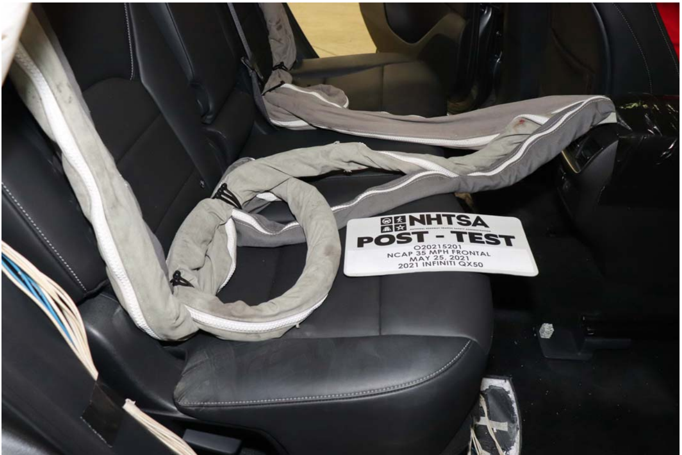
Photo No. 029 - Post-Test Dummy Cable Routing
