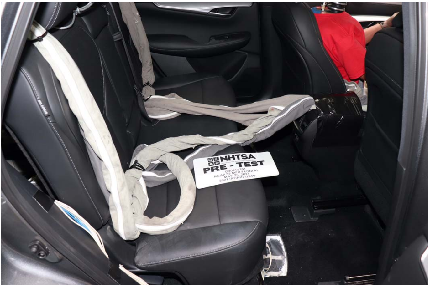
Photo No. 028 - Pre-Test Dummy Cable Routing
