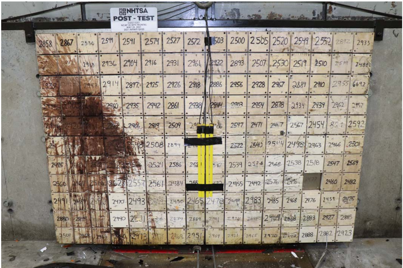
Photo No. 003 - Post-Test Load Cell Wall
