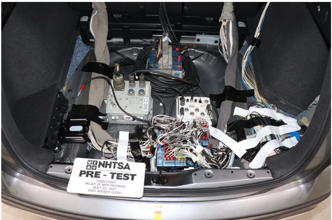
Photo No. 074 - Ballast Installed in Vehicle
