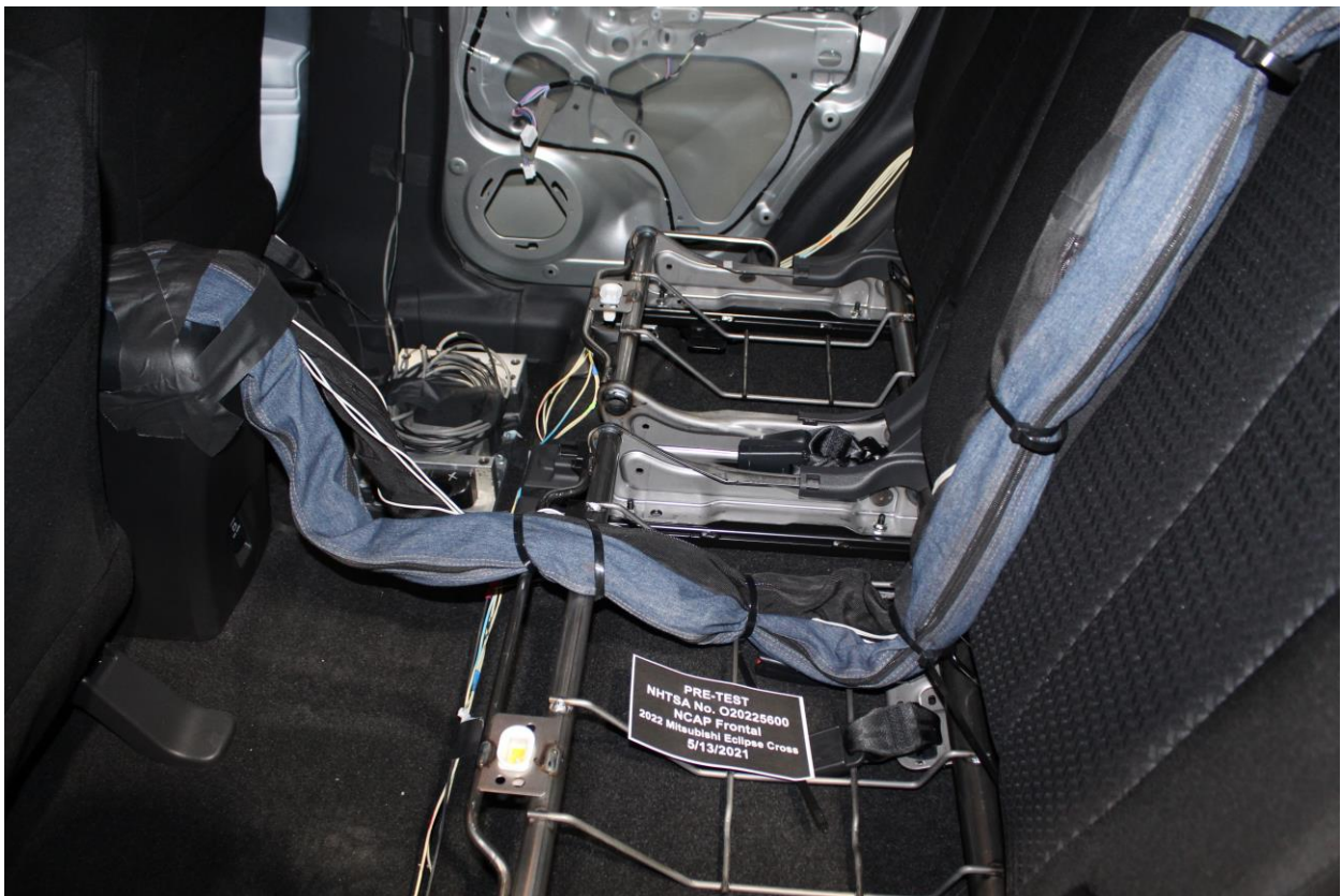
Figure A-28: Pre-Test Dummy Cable Routing
