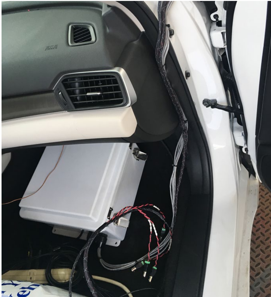
Figure 96. Power Supply and TTL Circuitry Enclosure
