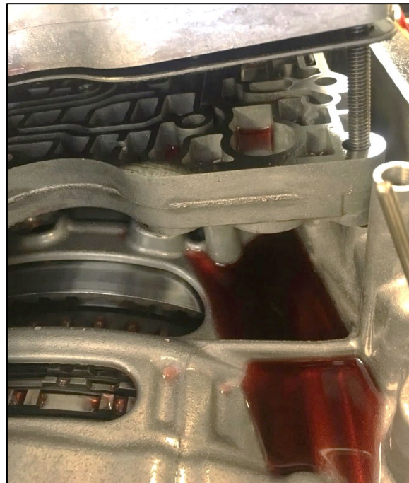
Figure 71. Ford 10R80 Valvebody Elevated to Show Pump Outlet Channel Into Valvebody
