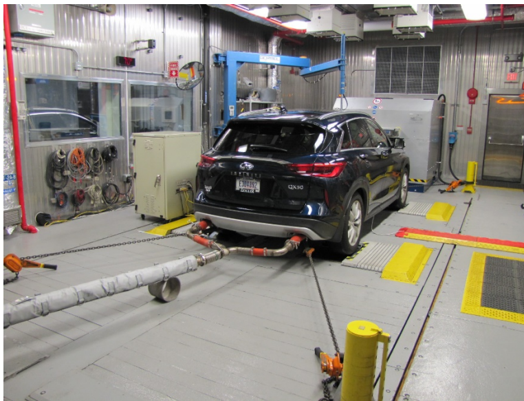
Figure 11. 2019 Infiniti QX50 test vehicle mounted to the chassis dynamometer inside the test cell
