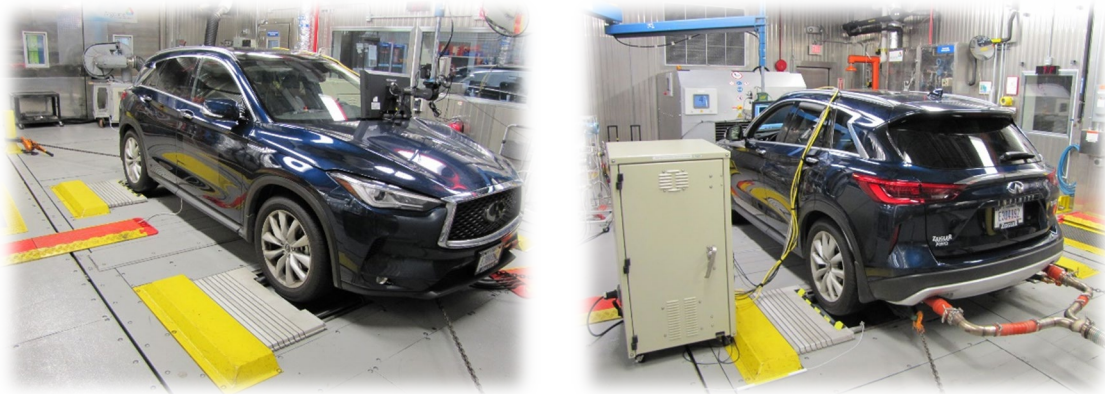
Figure 4. Vehicle mounted for full testing inside the AMTL 4WD chassis dynamometer.
