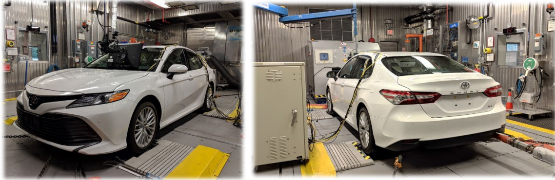
Figure 9. Figure 9: Vehicle mounted for full testing inside the AMTL 4WD chassis dynamometer.
