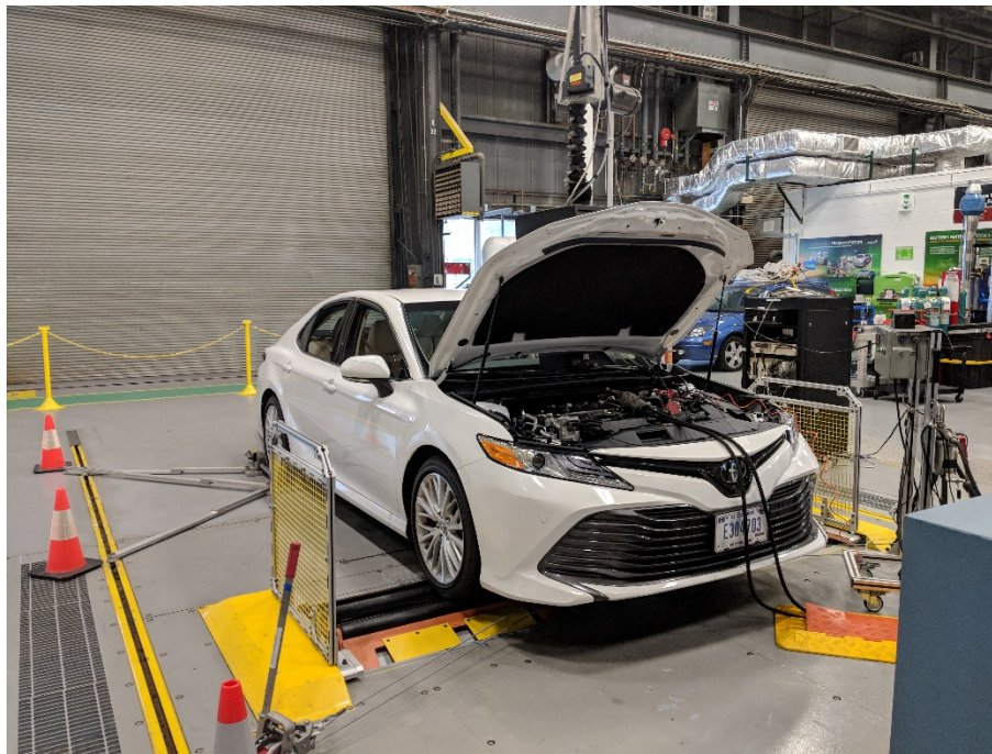
Figure 8. Vehicle mounted for mileage accumulation on the AMTL two-wheel drive (2WD) chassis dynamometer
