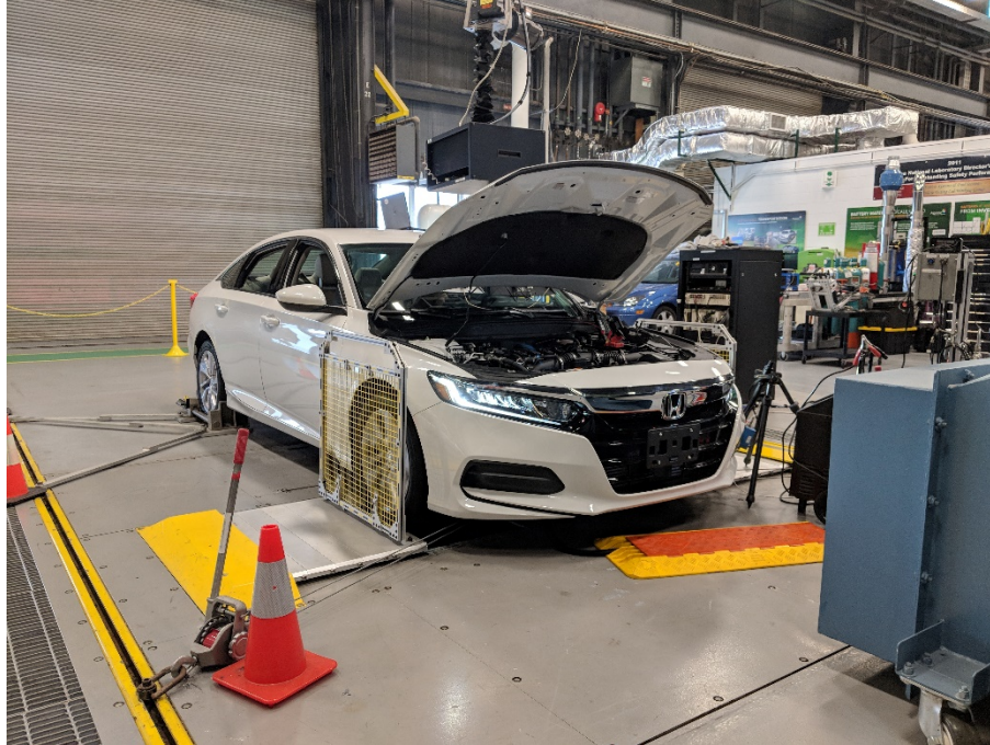
Figure 8: Vehicle mounted for mileage accumulation on the AMTL 2WD chassis dynamometer
