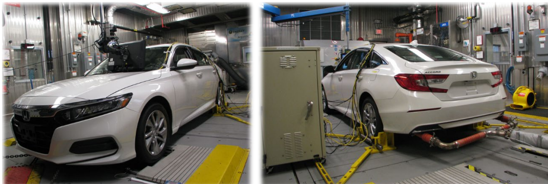
Figure 9: Vehicle mounted for full testing inside the AMTL 4WD chassis dynamometer
