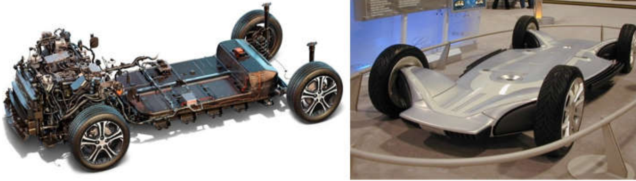
Figure 6. 2017 Chevrolet Bolt BEV Chassis with Powertrain (left); Example of a Flat Skateboard Chassis Containing Electric Powertrain (right).
