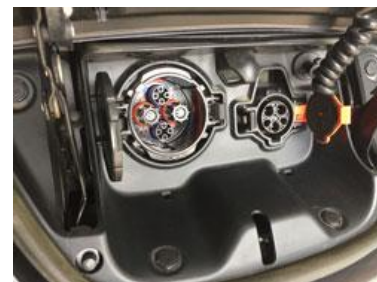
The SAE J1772 charge port (right) on a vehicle can be used to accept charge with Level 1 or 2 charging equipment. The DC fast charging receptacle (left) uses a different type of connector. In this photo, it is a CHAdeMO.
