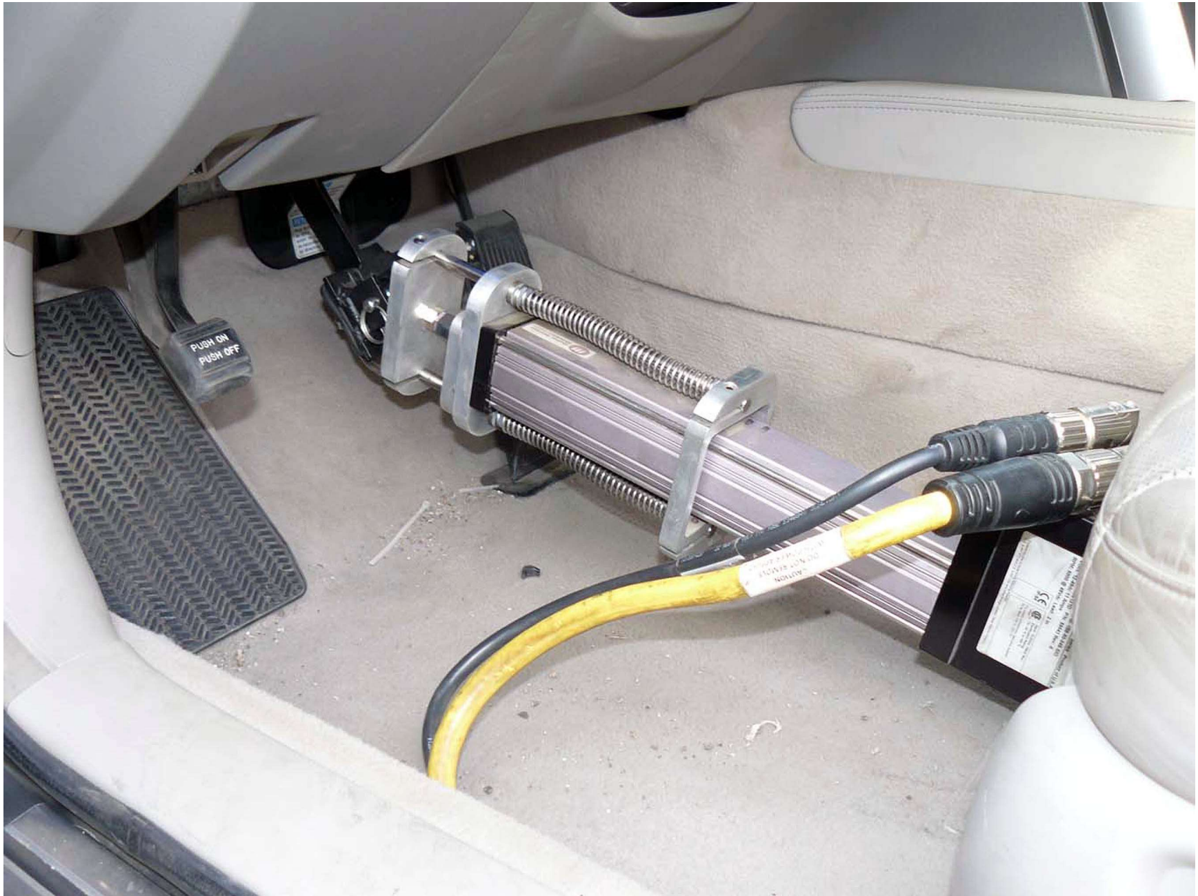
Figure A13. Brake Actuator Installed in POV System A-15
