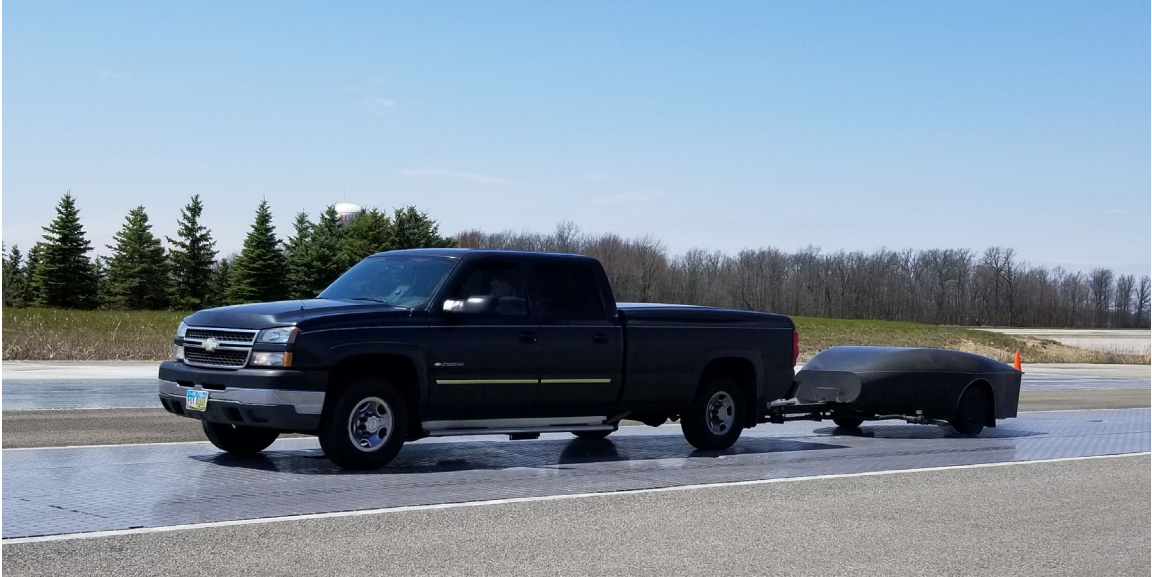
TRC Inc. ASTM E274 Locked Wheel Friction Tester on Ceramic Tile Course
