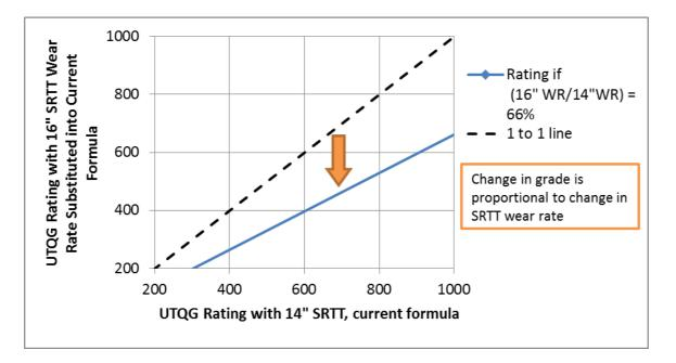
These calculations used the results of the first two quarters of testing to determine a ratio of 16" to 14" wear rate (66%). This ratio is not final, and is used here as an example.
