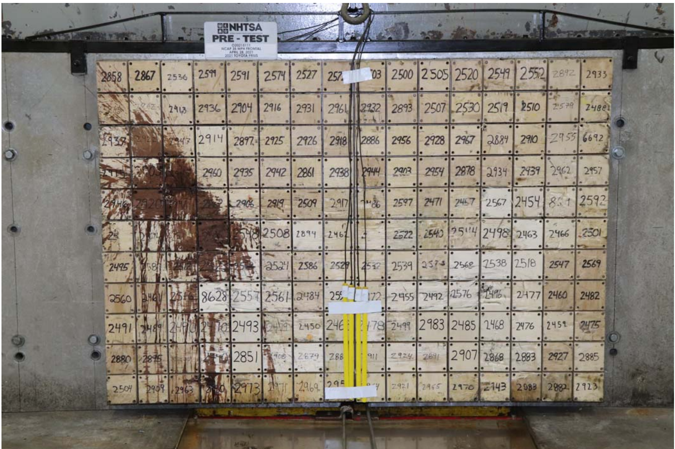
Photo No. 002 - Pre-Test Load Cell Wall
