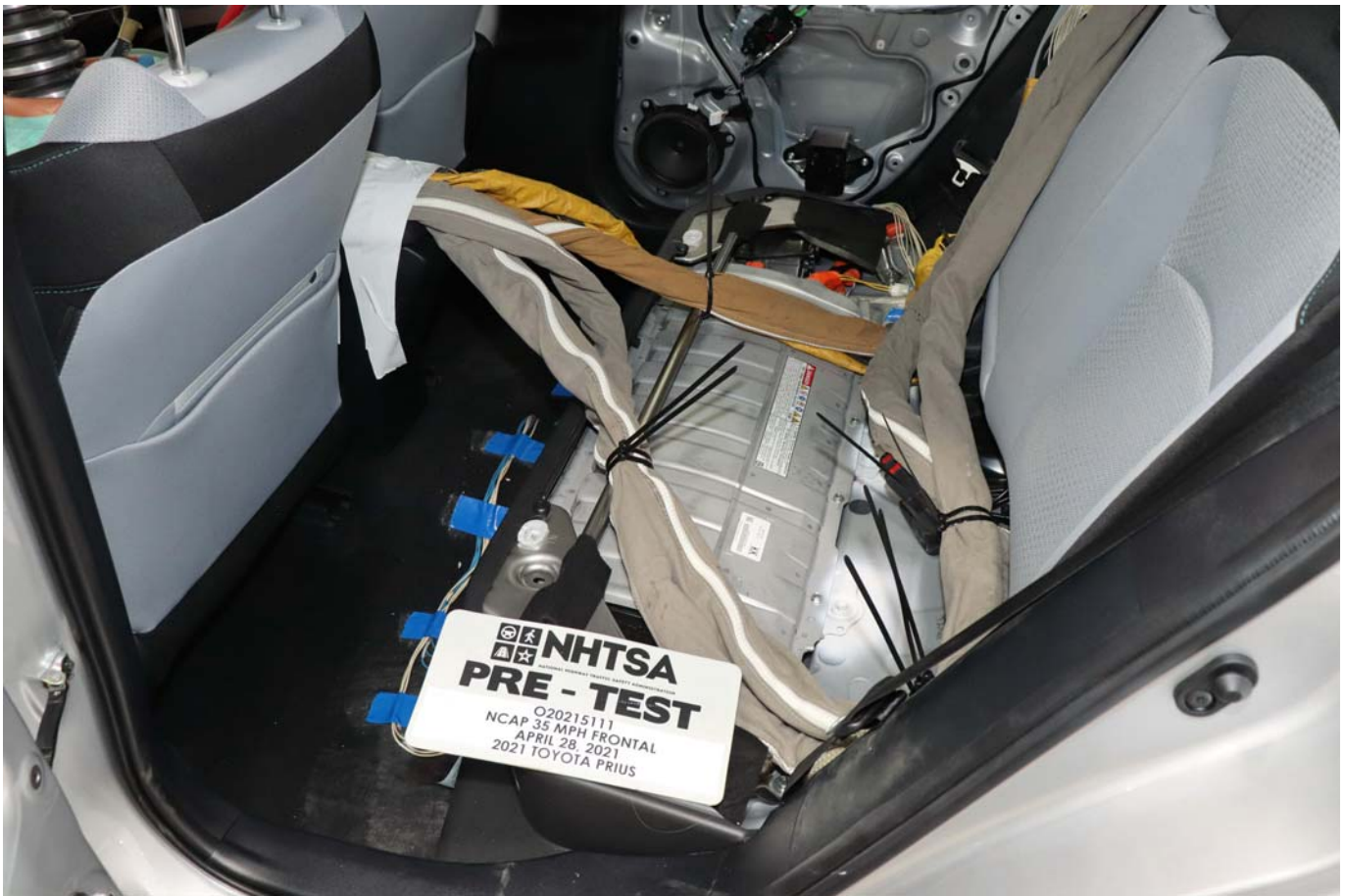
Photo No. 028 - Pre-Test Dummy Cable Routing
