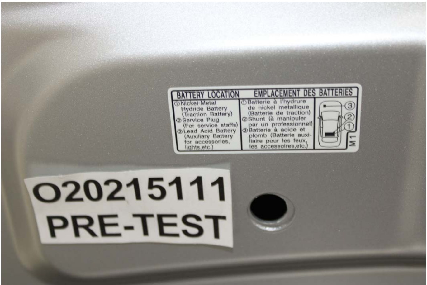
Photo No. 305-03 - First Responder Warning Label
