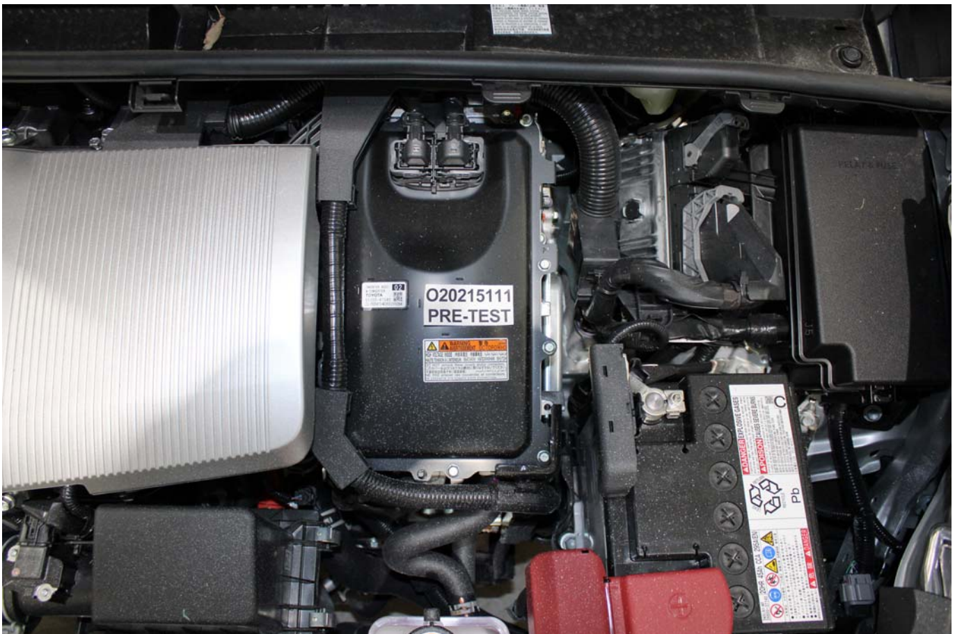
Photo No. 305-02 - Power Inverter Warning Label
