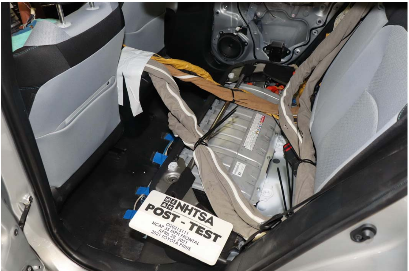
Photo No. 029 - Post-Test Dummy Cable Routing
