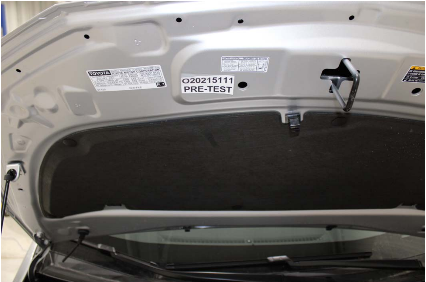
Photo No. 305-04 - First Responder Warning Location
