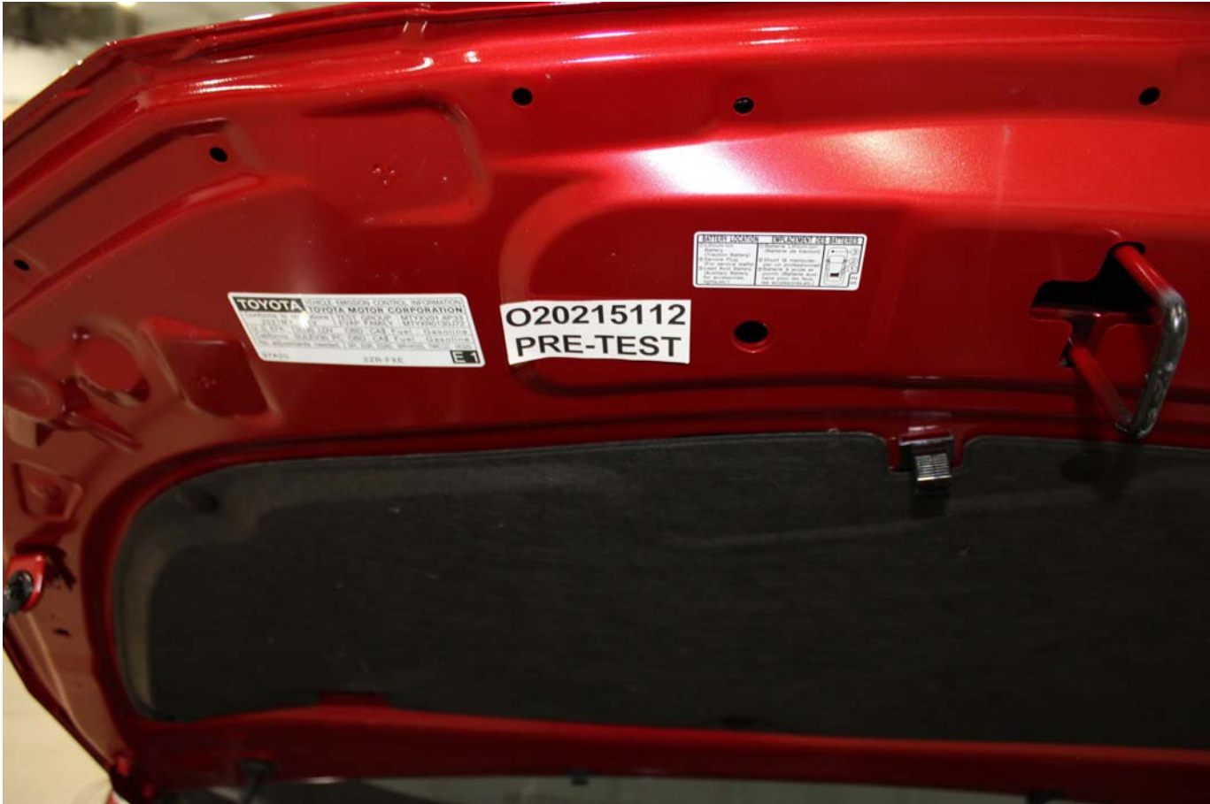
Photo No. 305-04 - First Responder Warning Location
