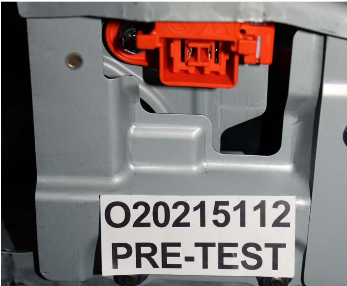
Photo No. 305-07 - Manual High Voltage Service Disconnect Removed
