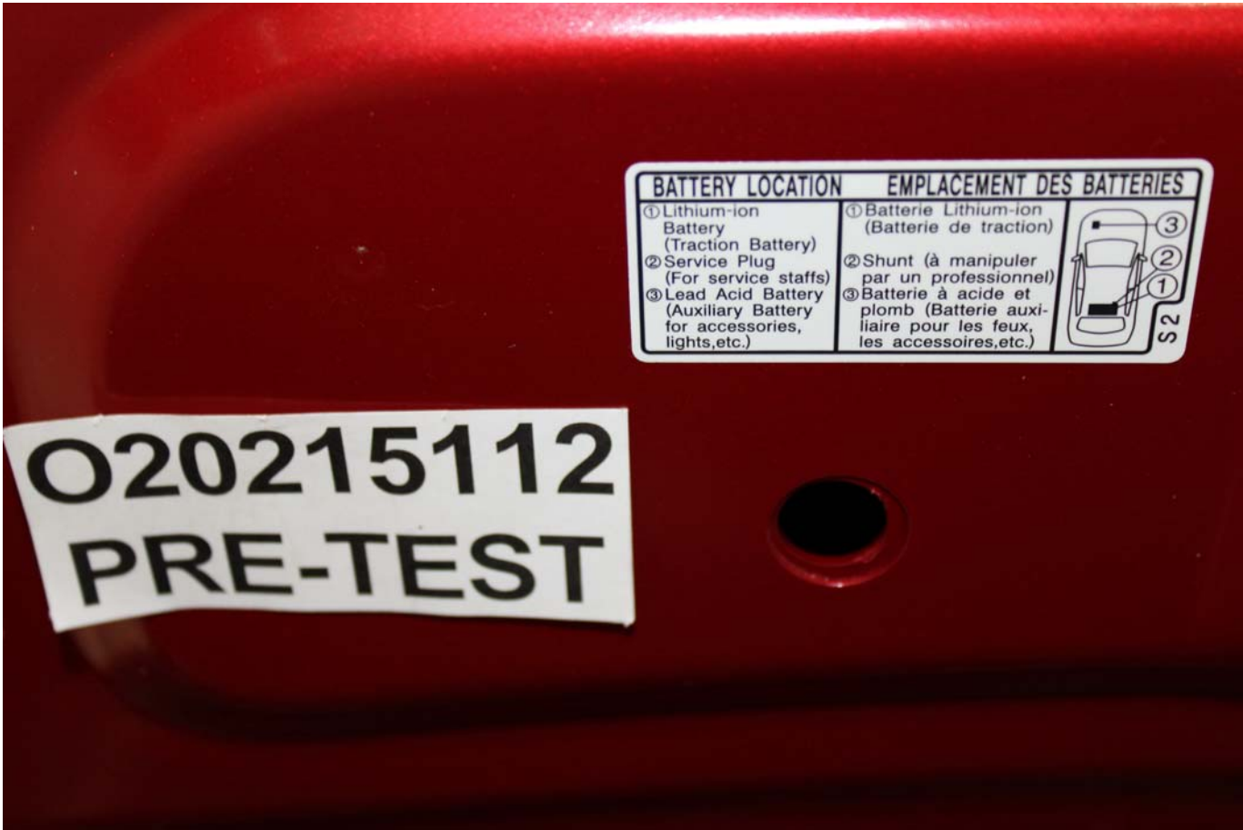
Photo No. 305-03 - First Responder Warning Label
