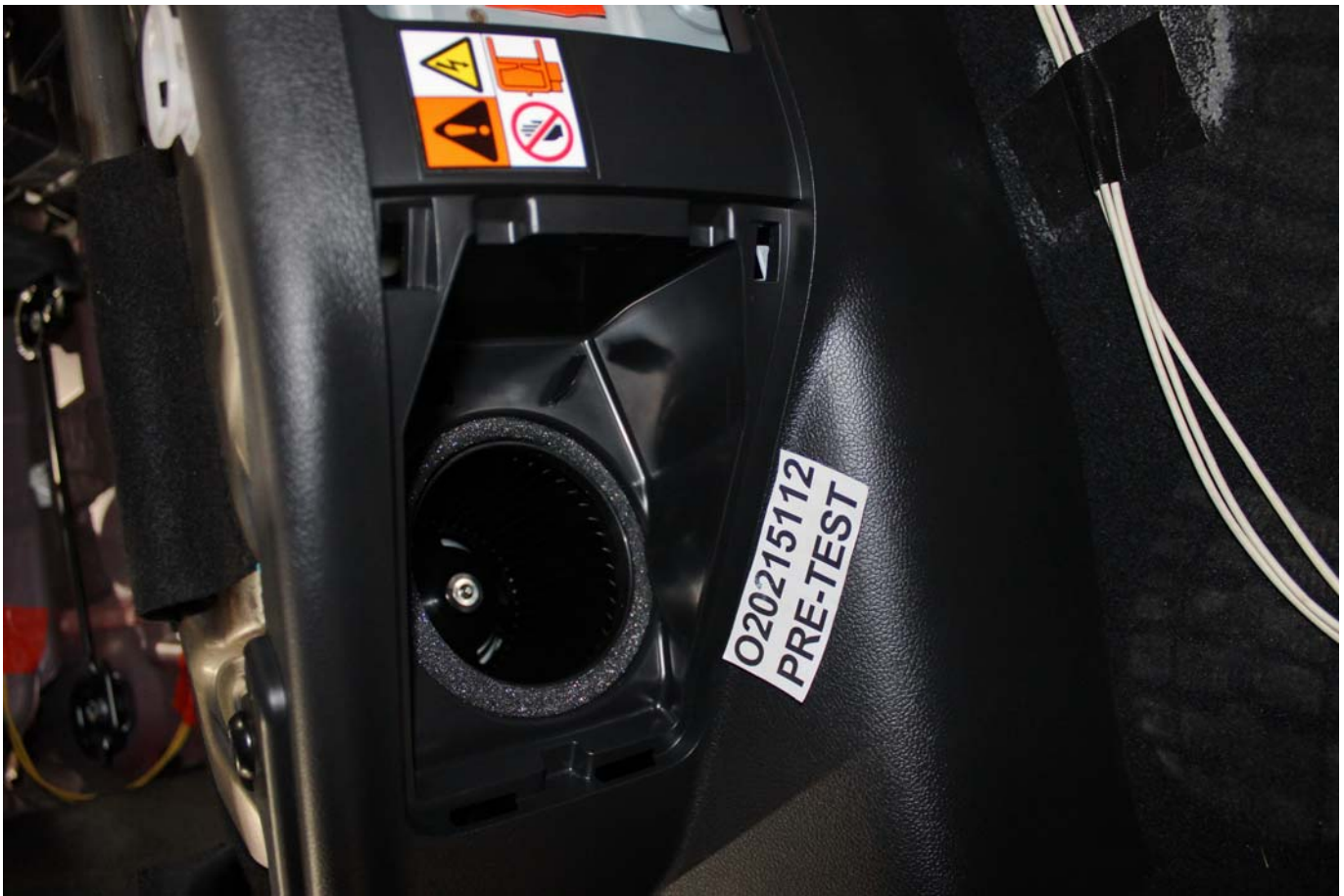
Photo No. 305-19 - Pre-Impact View Propulsion Battery Venting System(s)
