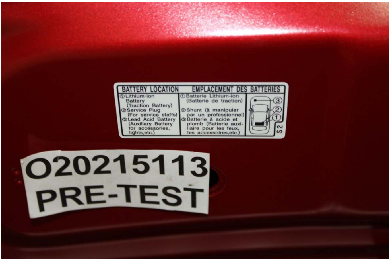
Photo No. 305-03 - First Responder Warning Label
