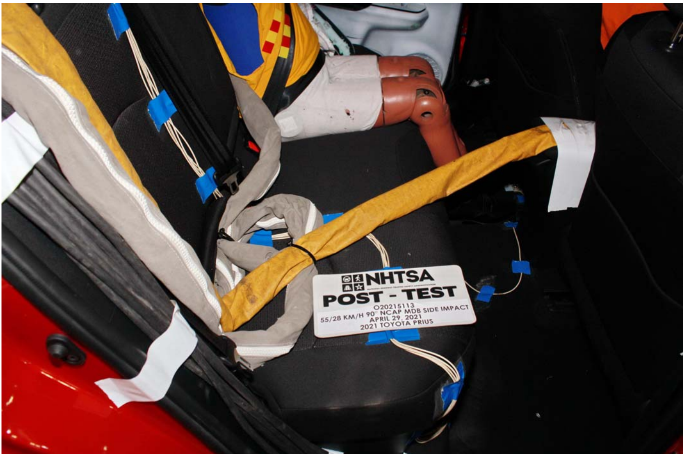
Photo No. 305-33 - Post-Impact View of the Vehicle Passenger Compartment Adjacent to Propulsion Battery
