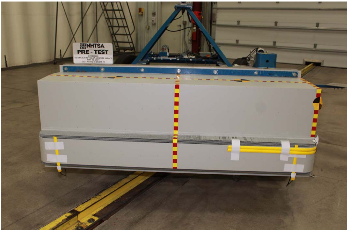
Photo No. 084 - Pre-Test Front View of MDB Impactor Face
