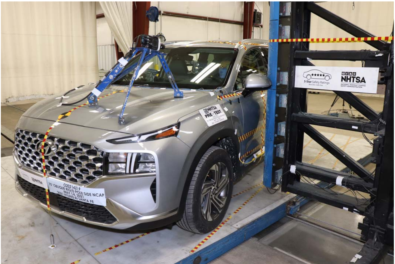
Photo No. 017 - Pre-Test Left Side View of Pole Positioned Against Side of Vehicle
