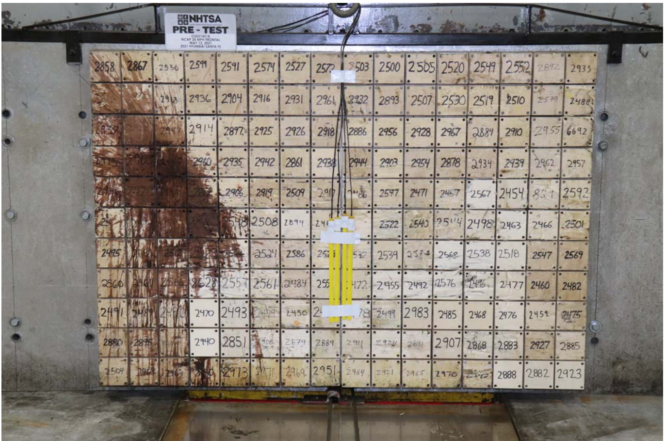
Photo No. 002 - Pre-Test Load Cell Wall
