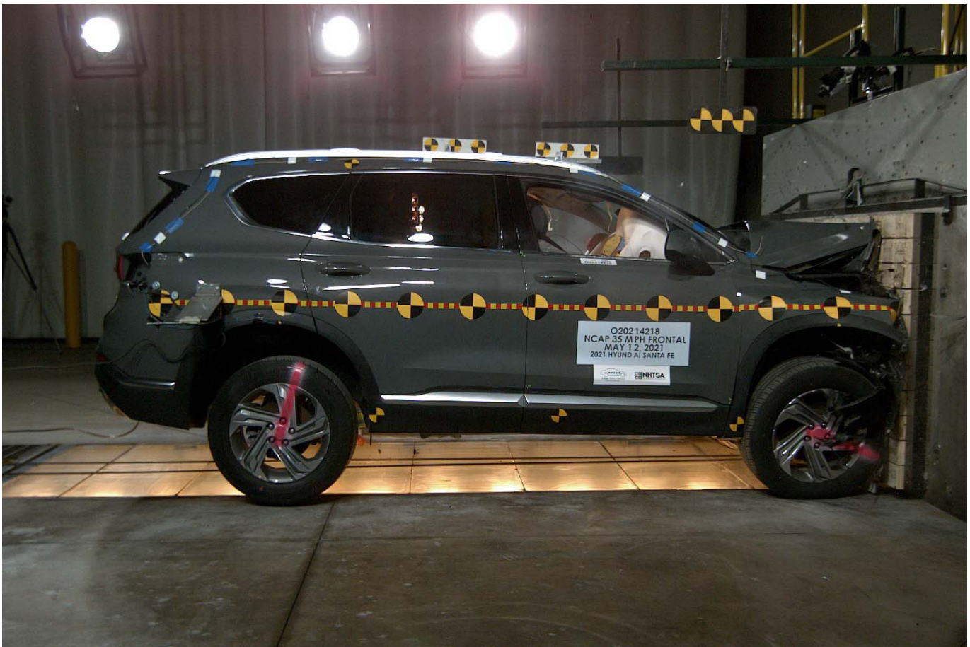
Photo No. 082 - 2021 Hyundai Santa Fe SEL AWD 5-Door SUV Frontal Impact Event
