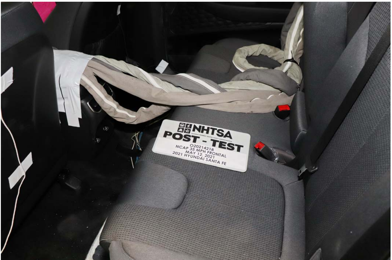
Photo No. 029 - Post-Test Dummy Cable Routing
