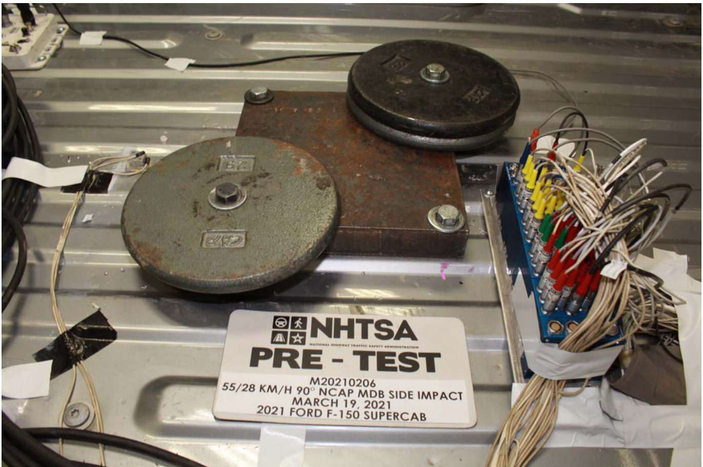
Photo No. 094 - Pre-Test Ballast View
