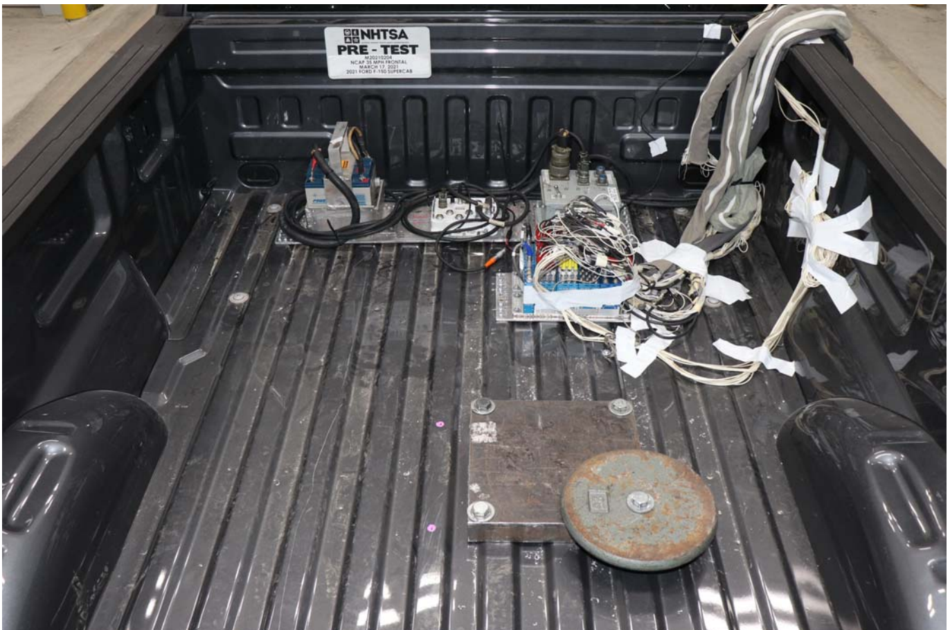
Photo No. 074 - Ballast Installed in Vehicle
