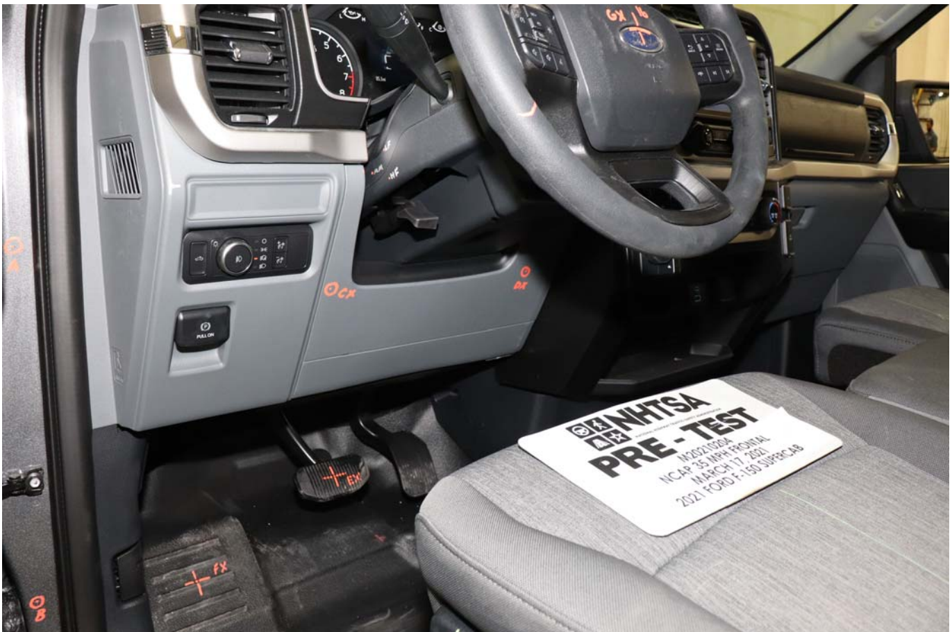
Photo No. 044 - Pre-Test Driver Side Knee Bolster
