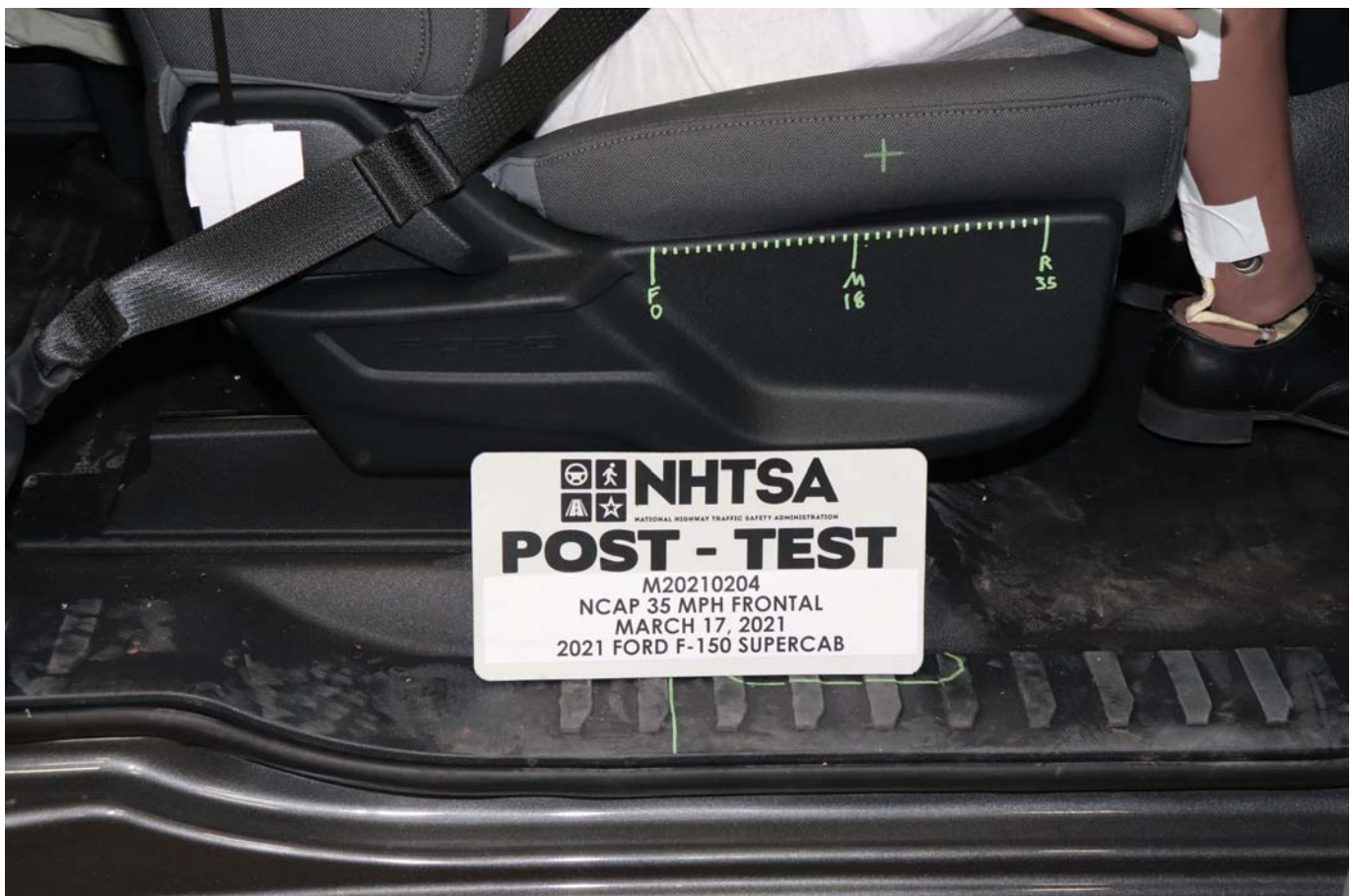
Photo No. 060 - Post-Test Passenger Seat Fore-Aft Markings
