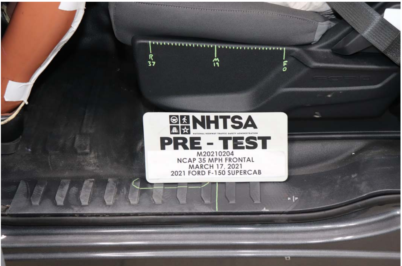
Photo No. 036 - Pre-Test Driver Seat Fore-Aft Markings
