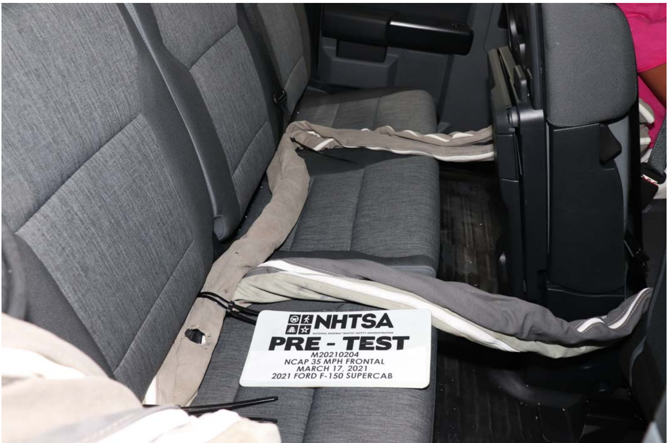
Photo No. 028 - Pre-Test Dummy Cable Routing
