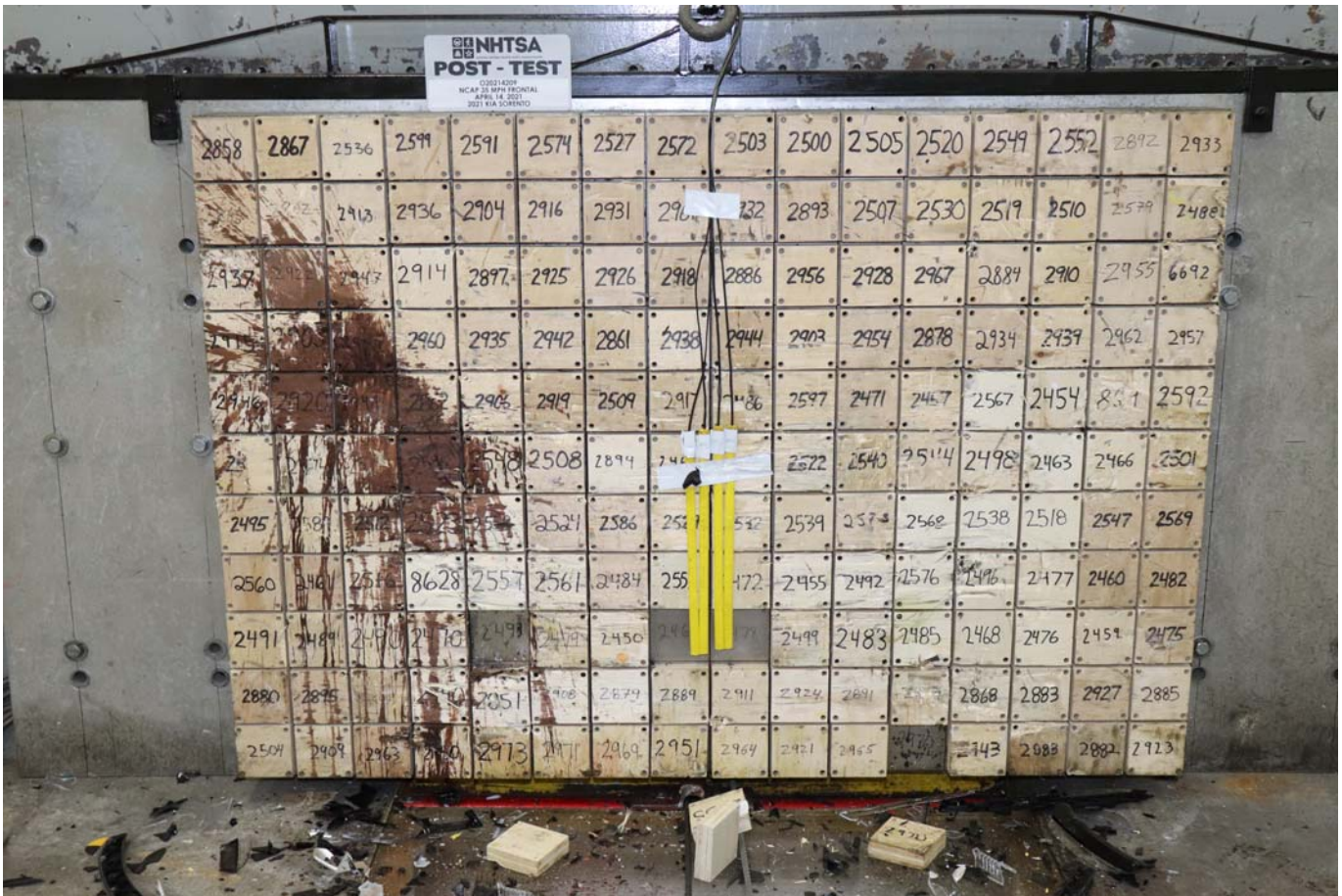
Photo No. 003 - Post-Test Load Cell Wall
