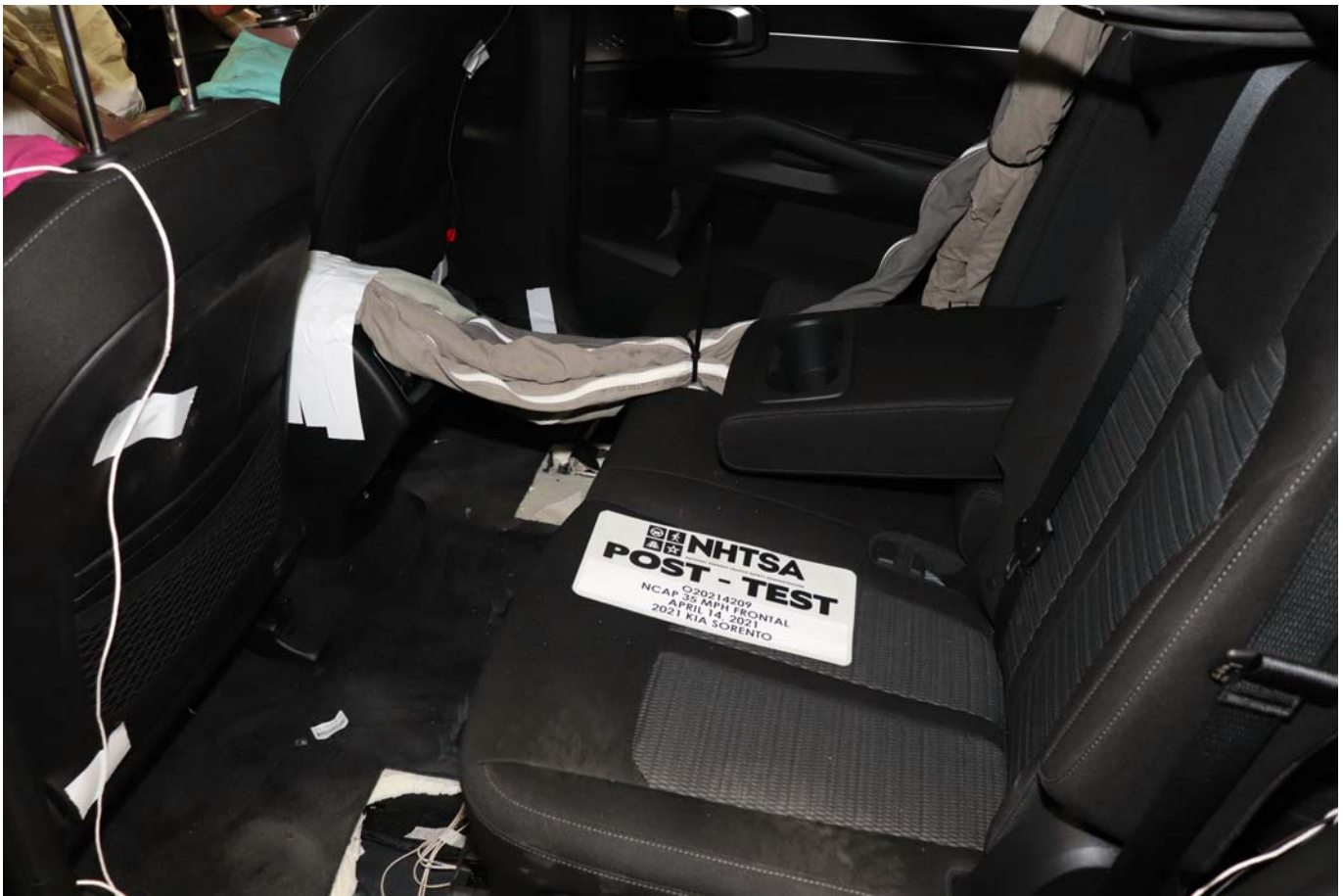
Photo No. 029 - Post-Test Dummy Cable Routing
