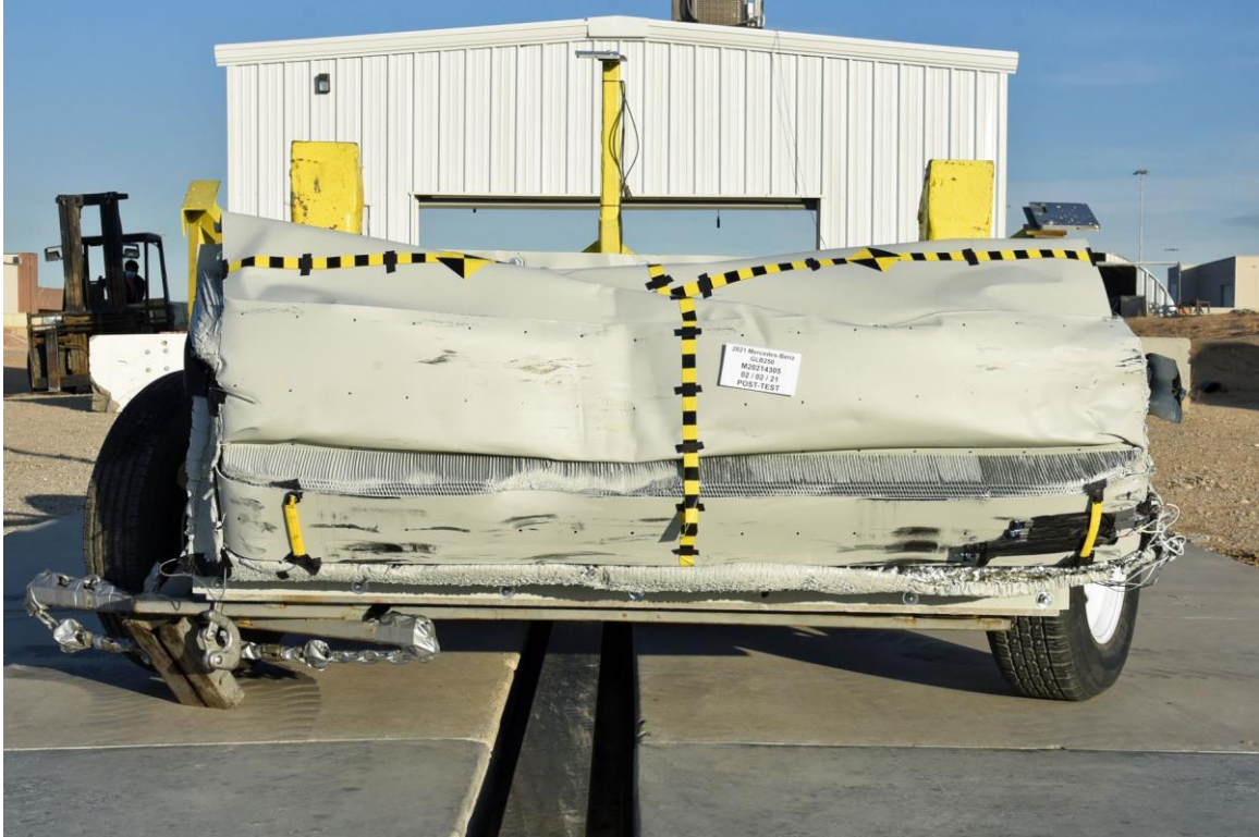
FIGURE 85. Post-Test Front View of MDB Impactor Face
