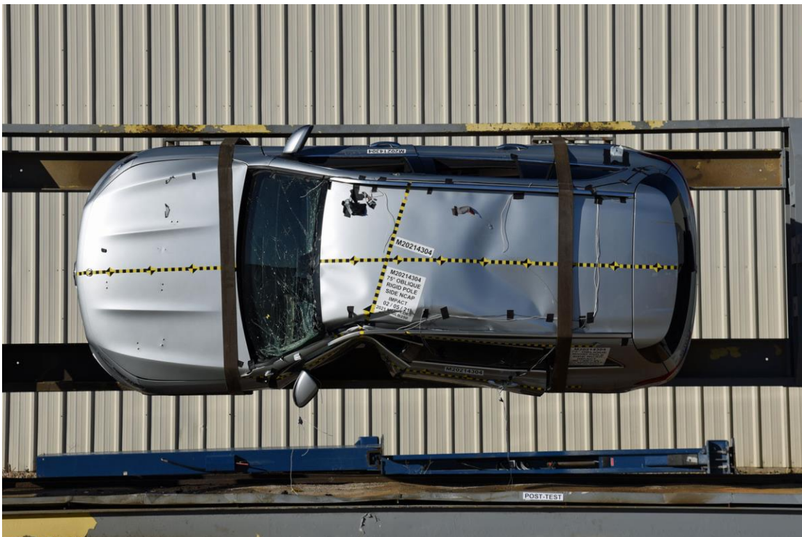
FIGURE 66. FMVSS No. 301 Static Rollover 90 Degrees
