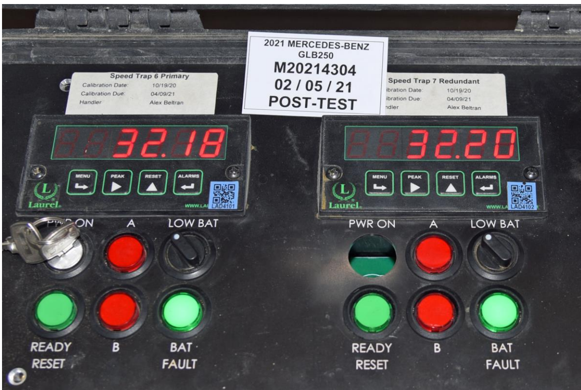
FIGURE 64. Post-Test Primary and Redundant Speed Trap Read-Out
