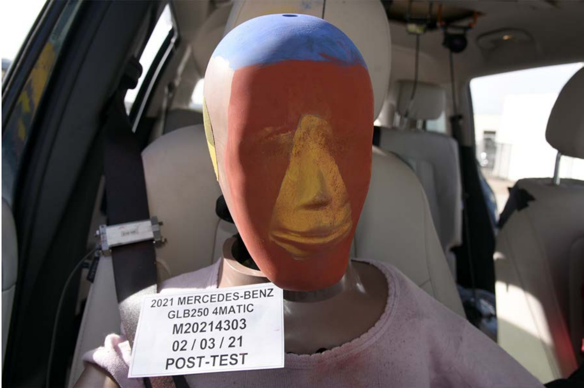
FIGURE 71. Post-Test Passenger Dummy Face
