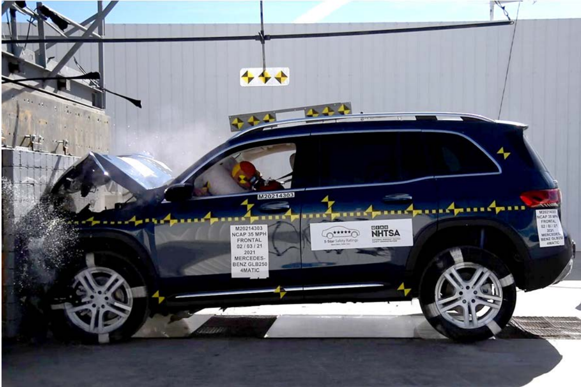
FIGURE 82. 2021 Mercedes-Benz GLB250 4MATIC Frontal Impact Event
