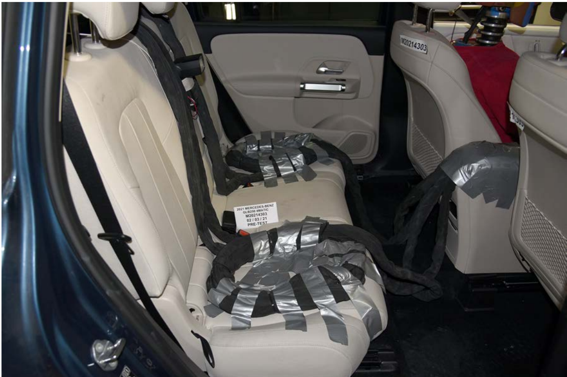
FIGURE 28. Pre-Test Dummy Cable Routing
