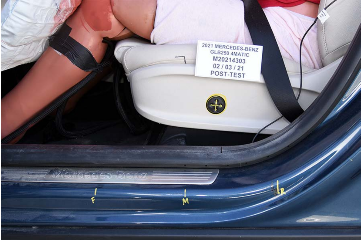
FIGURE 37. Post-Test Driver's Seat Fore-Aft Markings
