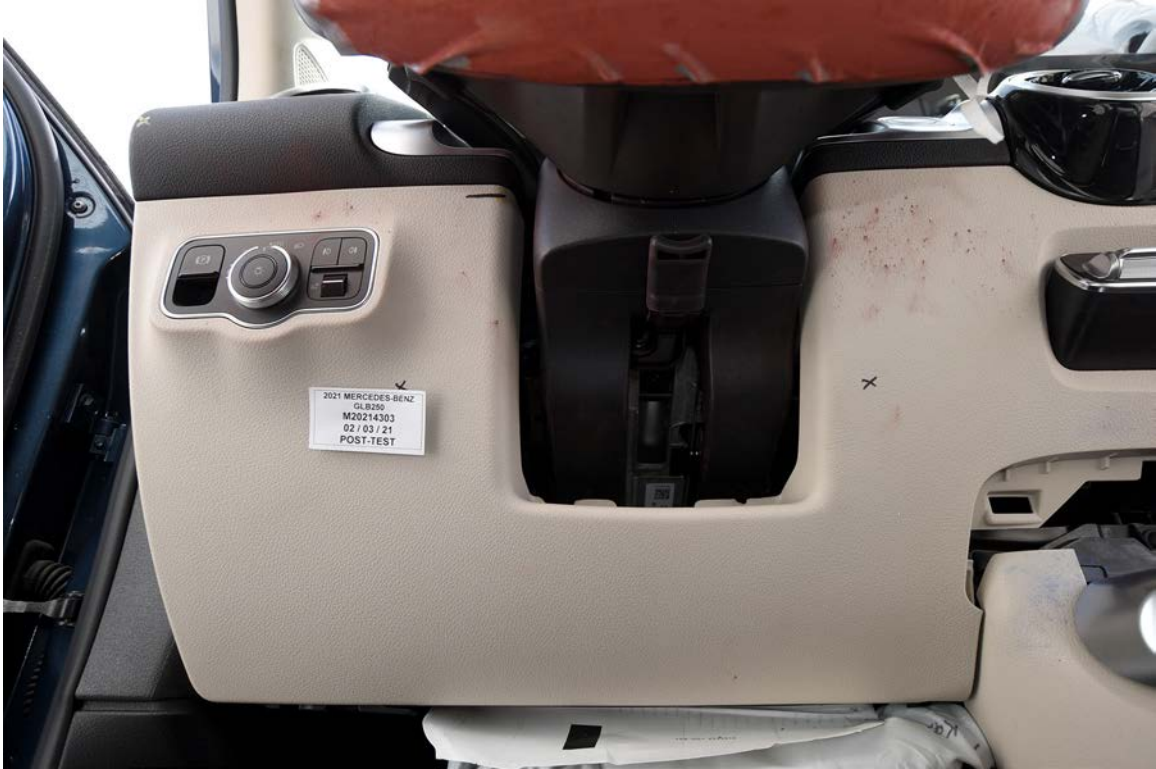
FIGURE 45. Post-Test Driver's Side Knee Bolster
