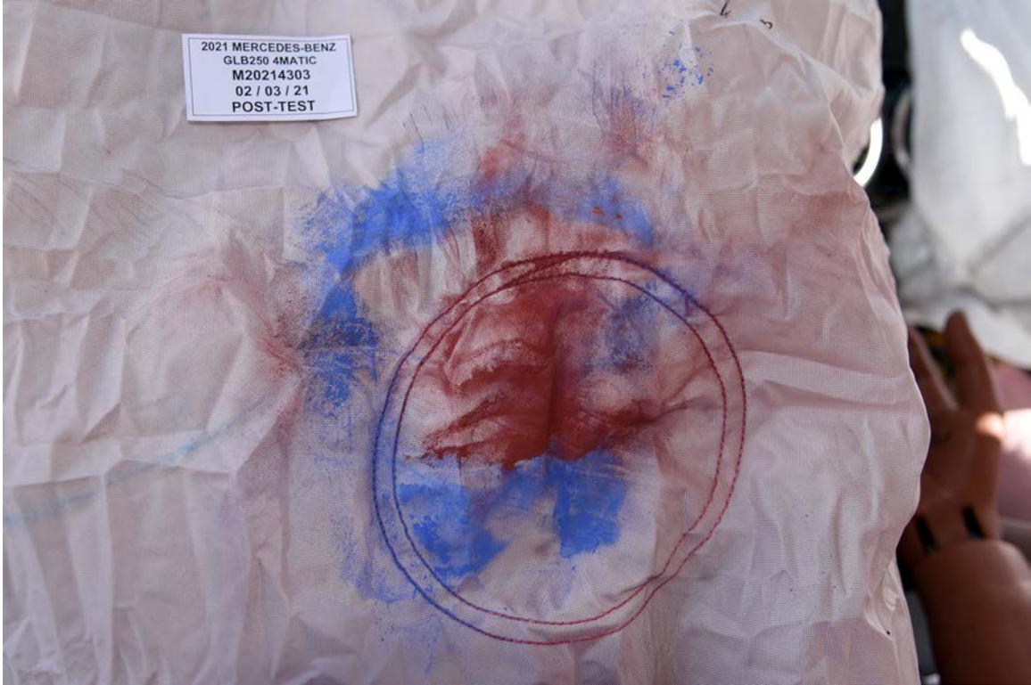
FIGURE 49. Post-Test Driver Dummy Contact with Airbag
