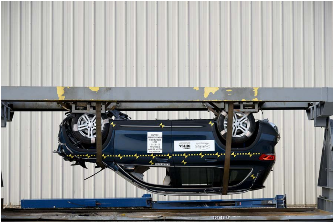
FIGURE 79. Vehicle at 180° on Static Rollover Device
