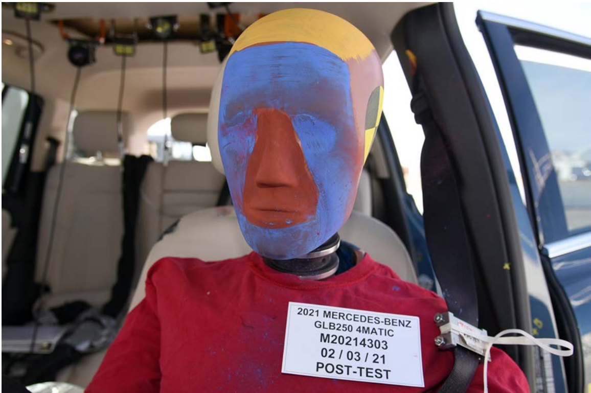
FIGURE 48. Post-Test Driver Dummy Face
