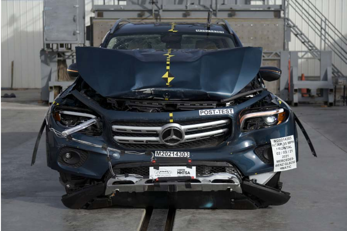
FIGURE 9. Post-Test Front View of Test Vehicle
