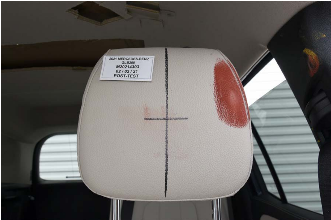
FIGURE 50. Post-Test Driver Dummy Contact with Headrest
