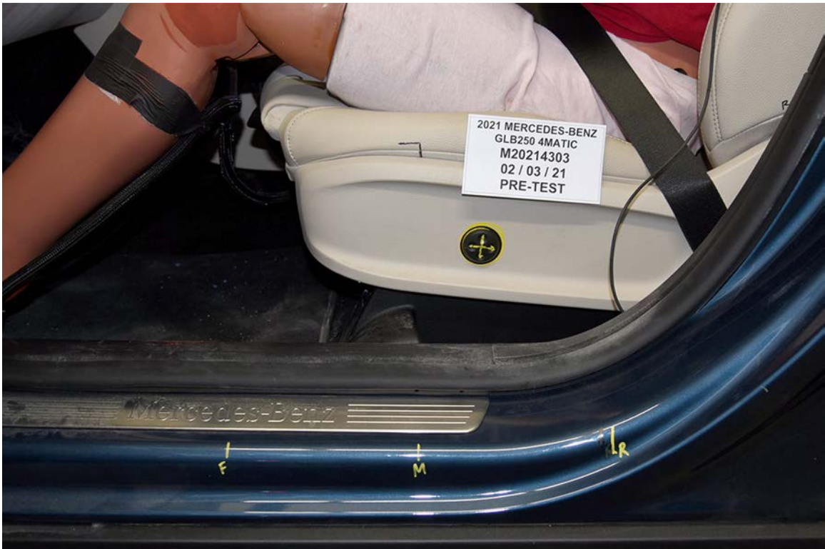
FIGURE 36. Pre-Test Driver's Seat Fore-Aft Markings
