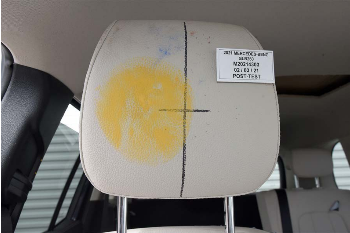
FIGURE 73. Post-Test Passenger Dummy Contact with Headrest
