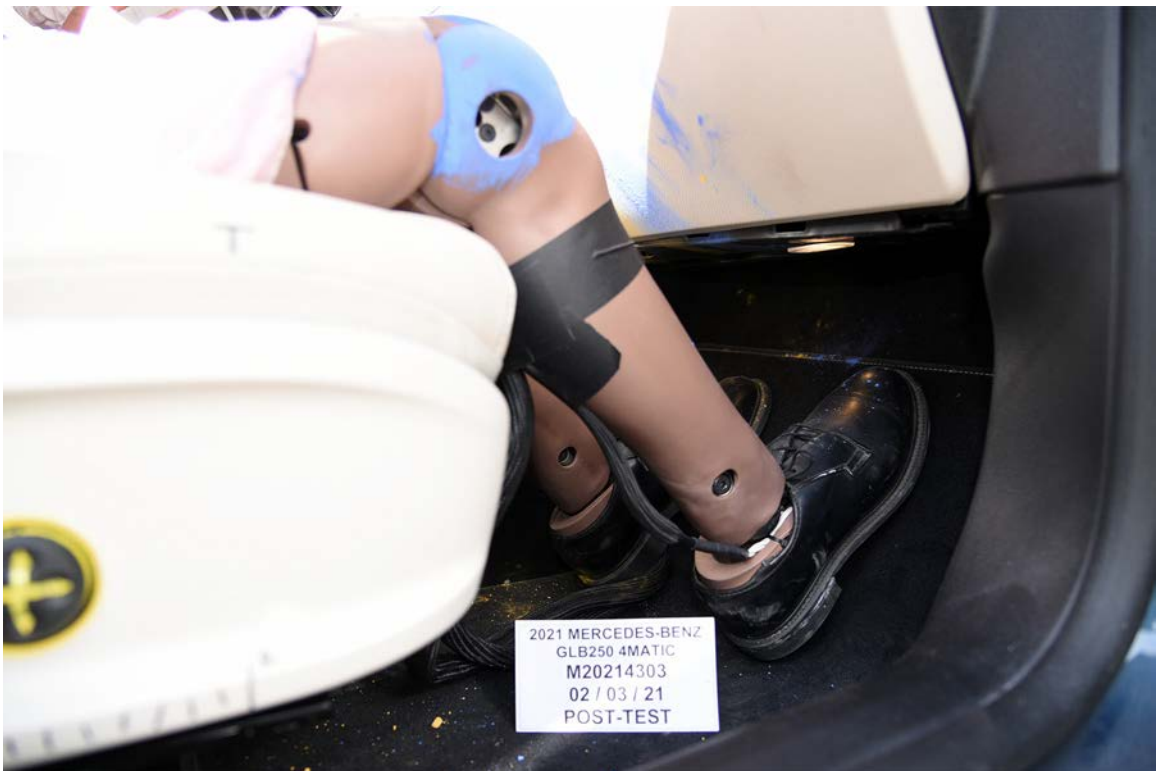
FIGURE 66. Post-Test Passenger Dummy Feet
