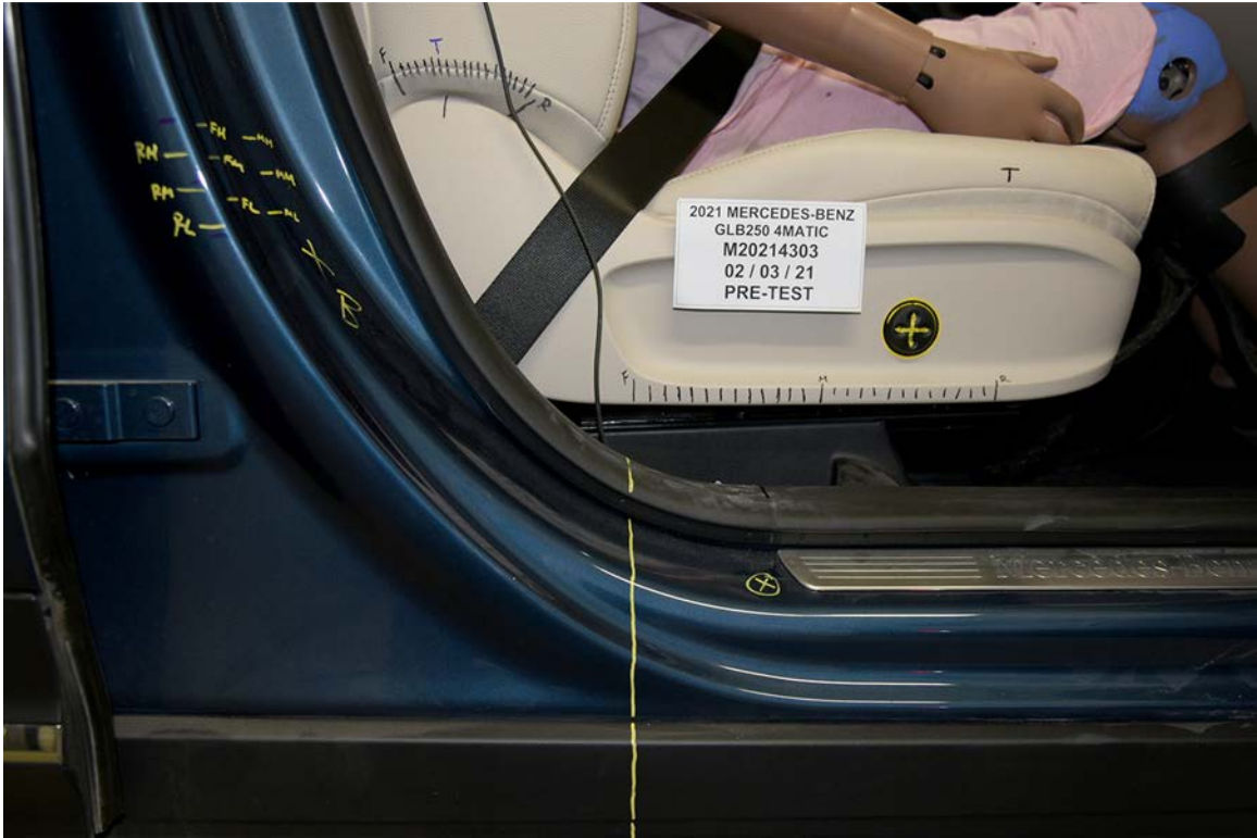
FIGURE 59. Pre-Test Passenger's Seat Fore-Aft Markings
