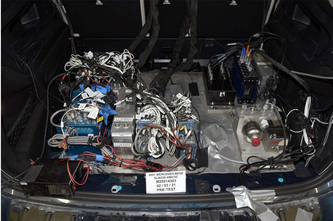
FIGURE 74. Photograph of Ballast Installed in Vehicle
