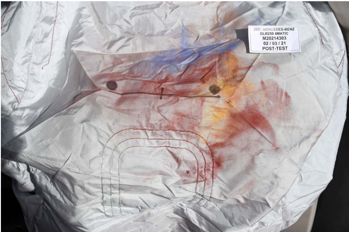
FIGURE 72. Post-Test Passenger Dummy Contact with Airbag
