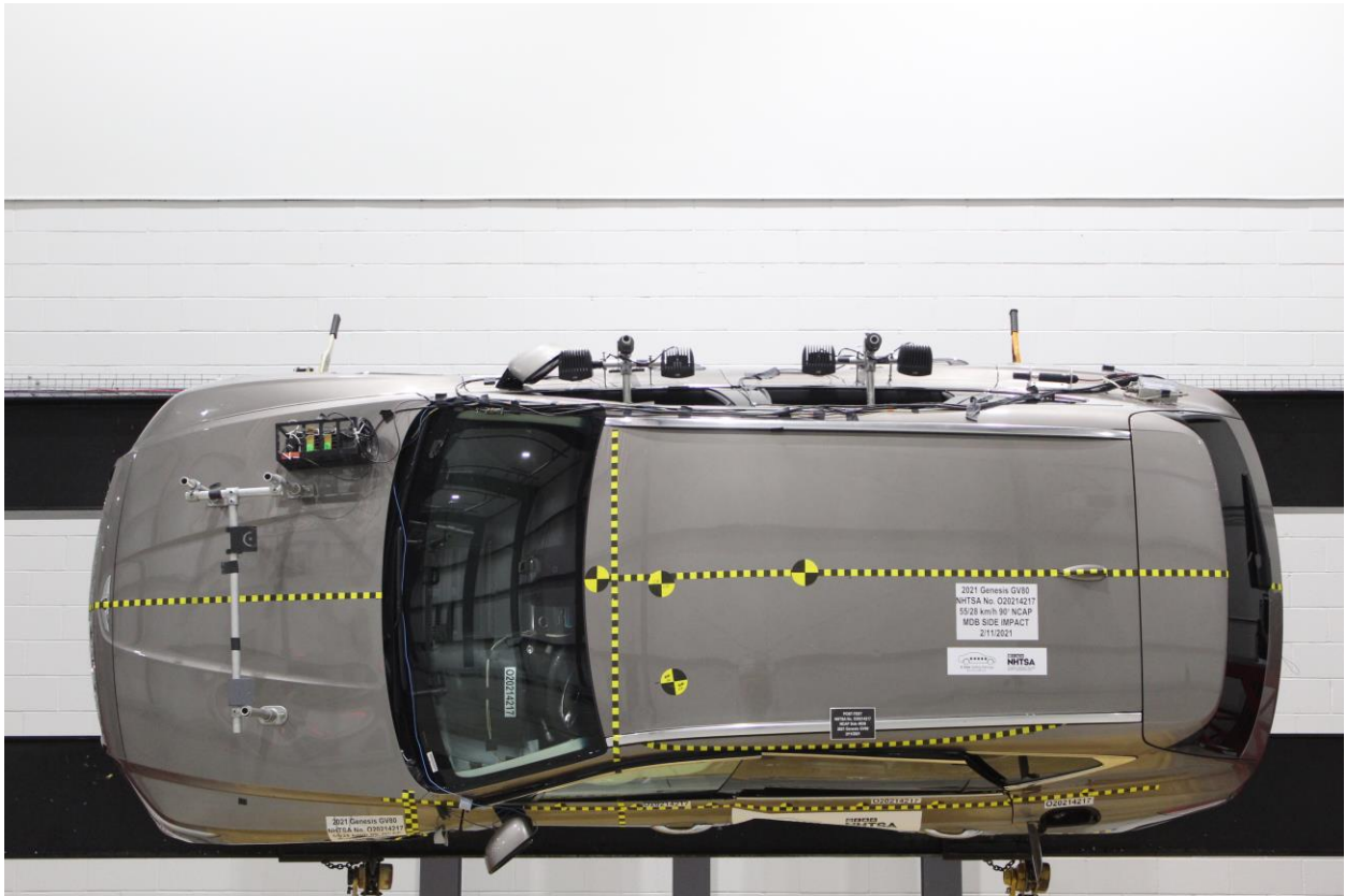
Figure A-97: FMVSS No. 301 Static Rollover 90 Degrees
