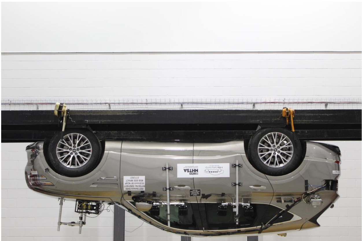
Figure A-98: FMVSS No. 301 Static Rollover 180 Degrees
