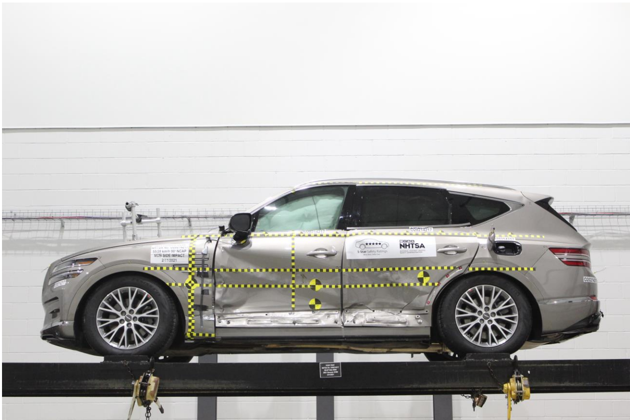
Figure A-96: FMVSS No. 301 Static Rollover 0 Degrees
