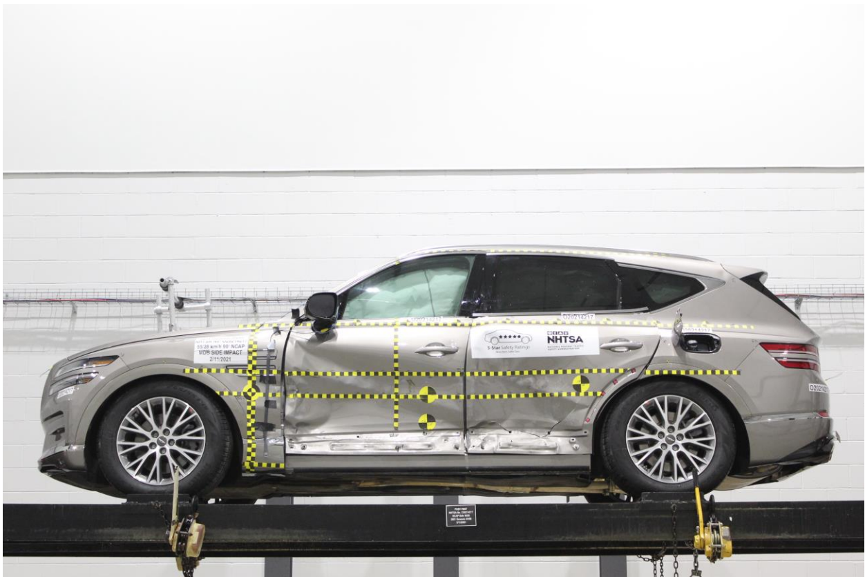
Figure A-100: FMVSS No. 301 Static Rollover 360 Degrees
