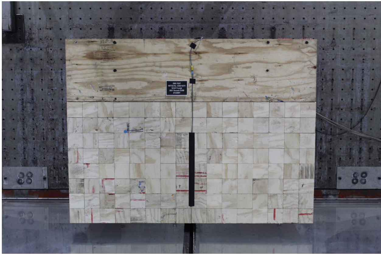
Figure A-2: Pre-Test Load Cell Wall
