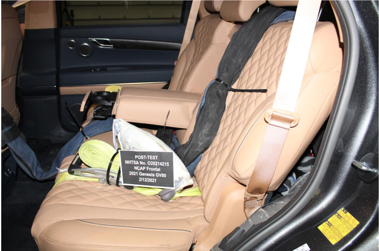
Figure A-29: Post-Test Dummy Cable Routing
