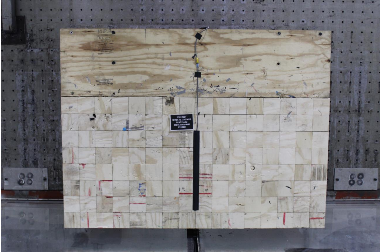
Figure A-3: Post-Test Load Cell Wall
