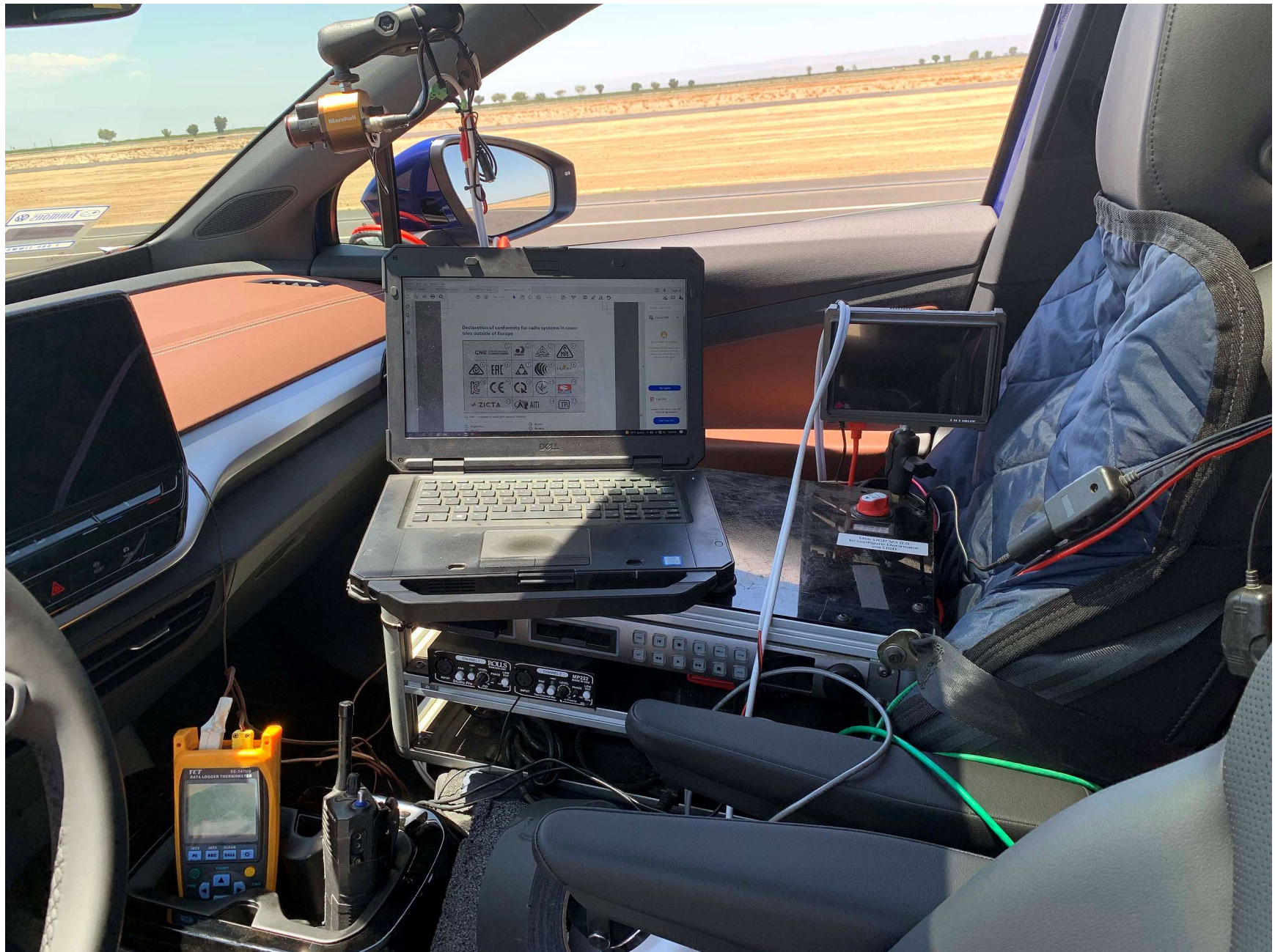
Figure A10. Computer Installed in Subject Vehicle
