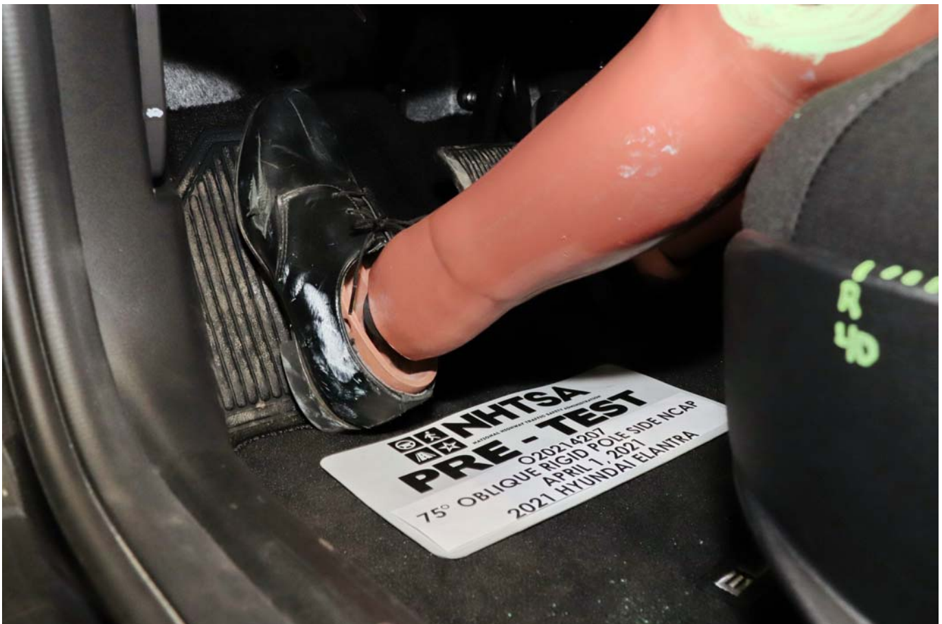
Photo No. 032 - Pre-Test Placement of Dummy Feet
