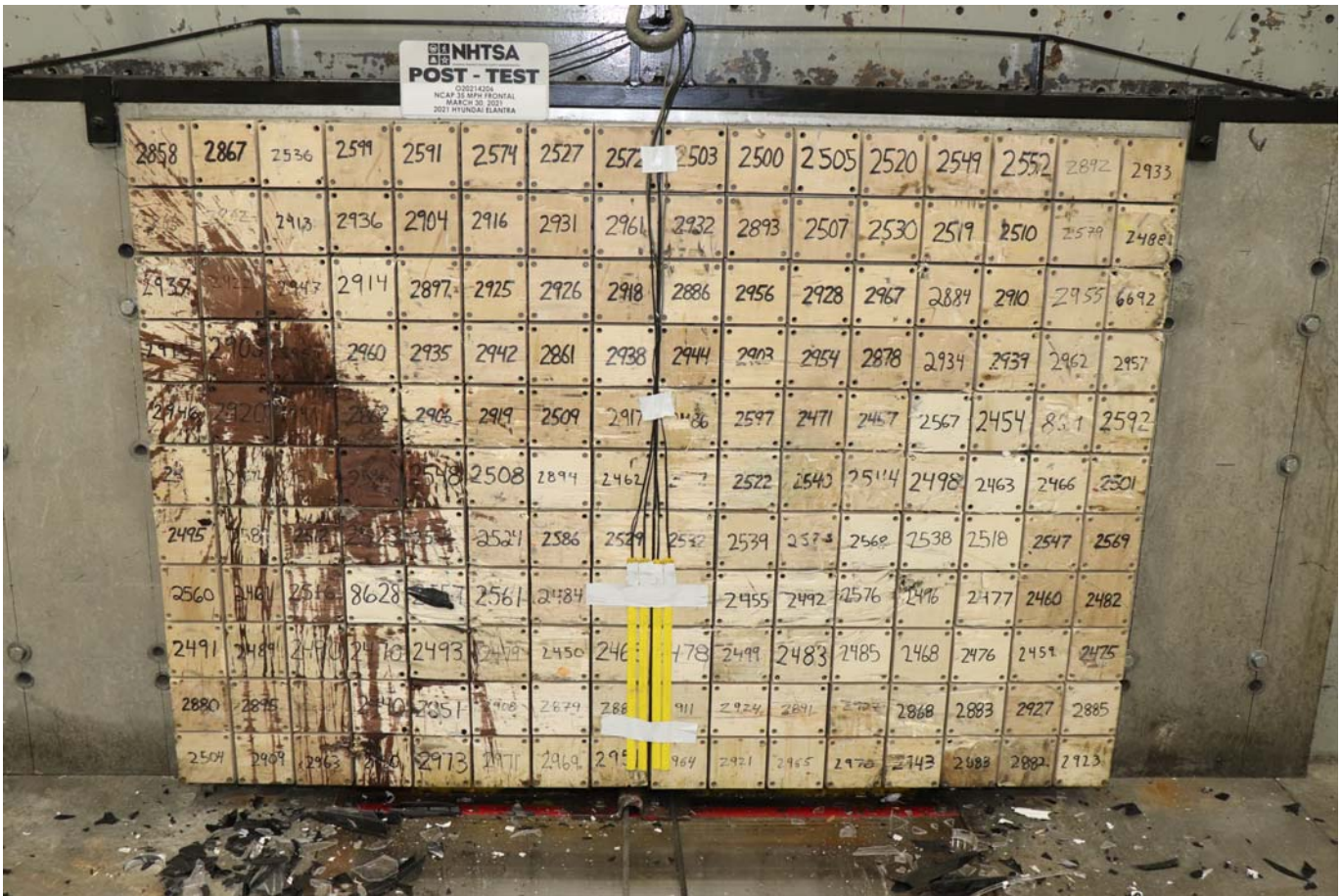
Photo No. 003 - Post-Test Load Cell Wall
