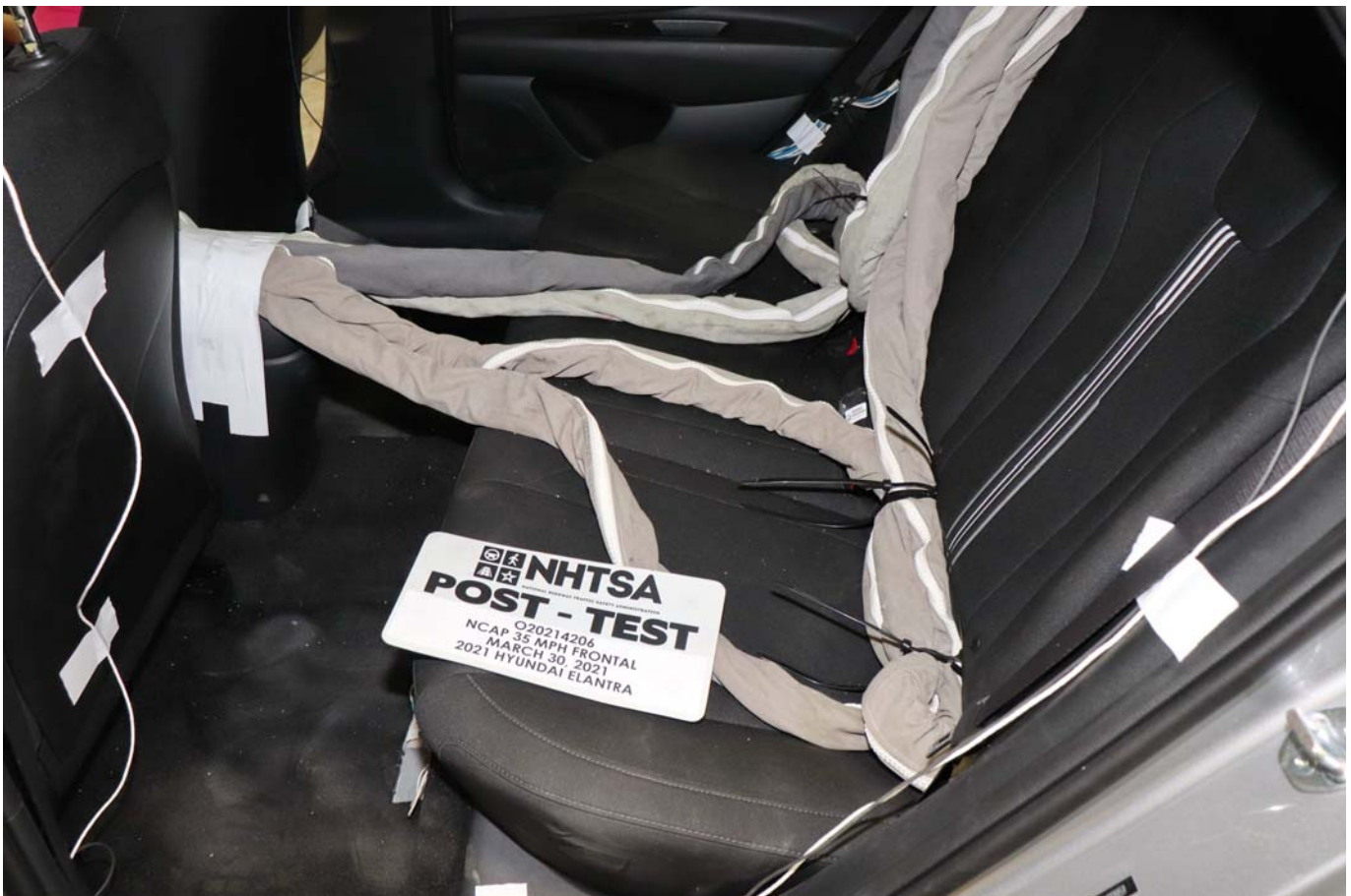
Photo No. 029 - Post-Test Dummy Cable Routing
