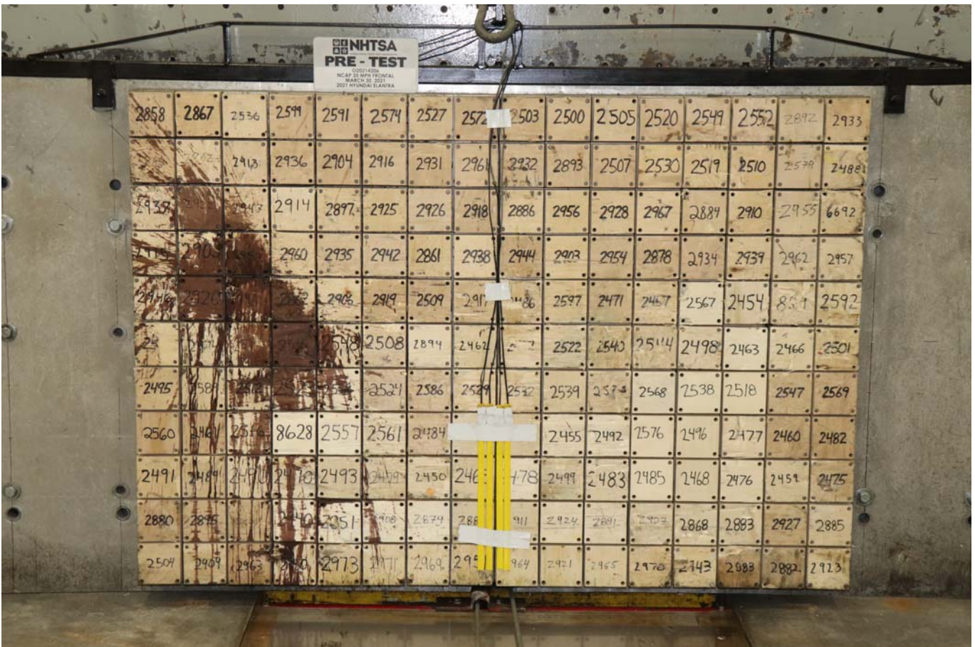
Photo No. 002 - Pre-Test Load Cell Wall
