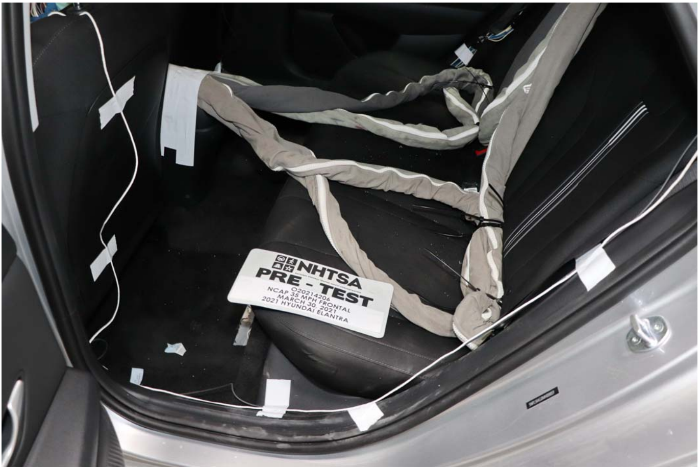
Photo No. 028 - Pre-Test Dummy Cable Routing
