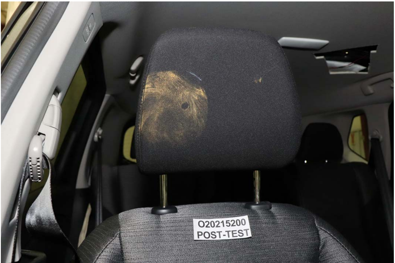
Photo No. 073 - Post-Test Passenger Dummy Contact with Headrest
