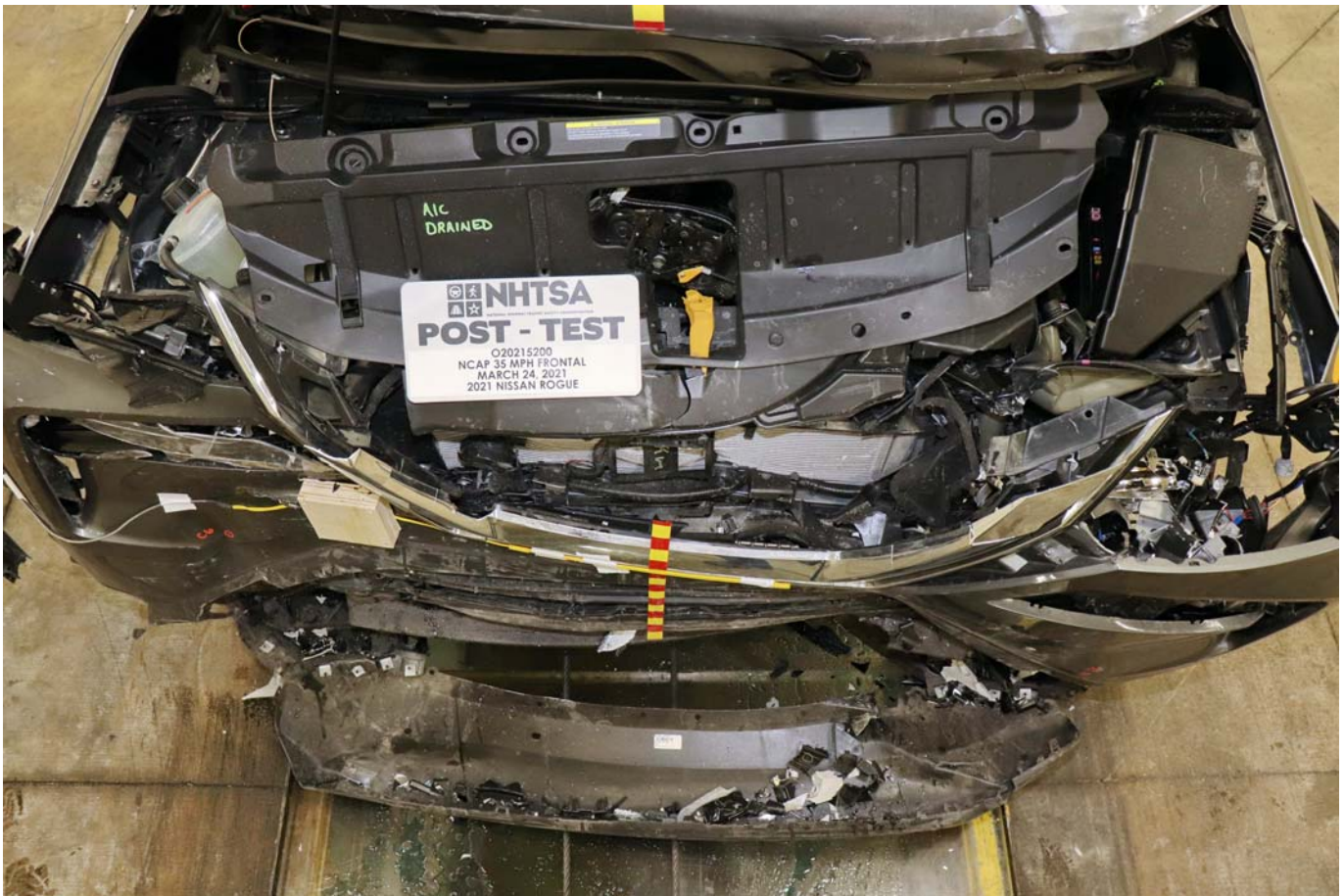
Photo No. 021 - Post-Test Engine Compartment View
