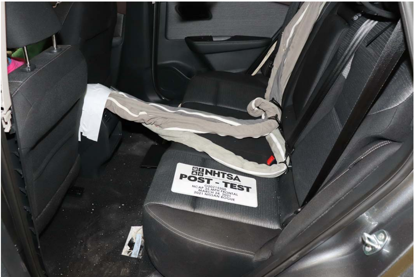
Photo No. 029 - Post-Test Dummy Cable Routing
