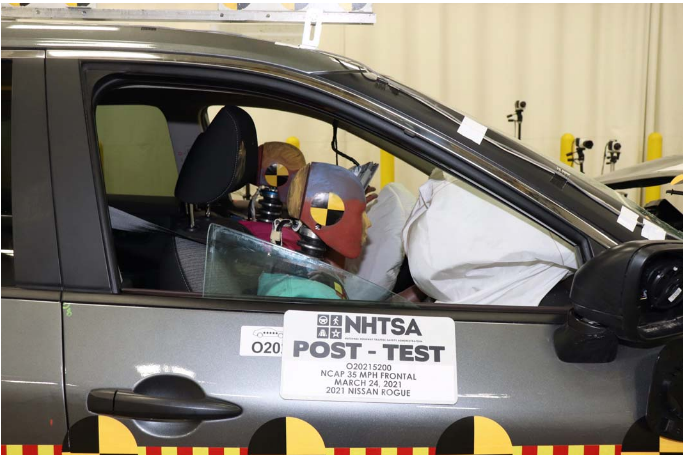
Photo No. 056 - Post-Test Passenger Dummy Window View
