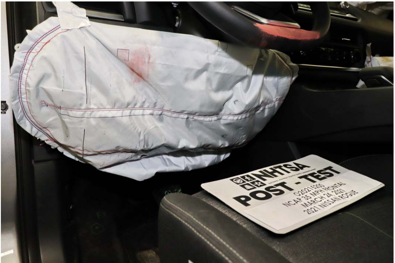
Photo No. 045 - Post-Test Driver Side Knee Bolster
