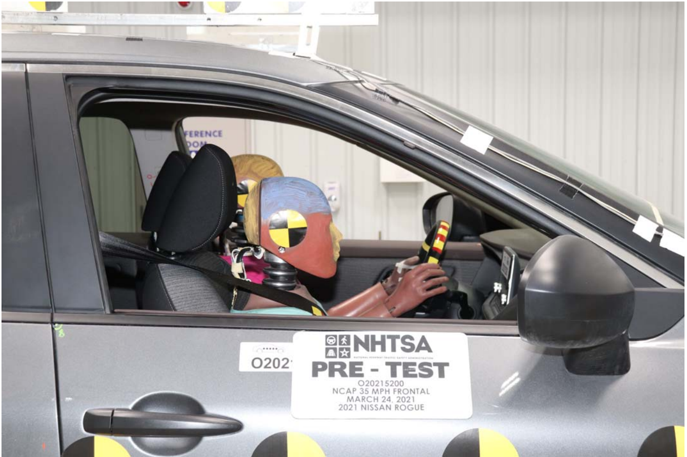
Photo No. 055 - Pre-Test Passenger Dummy Window View
