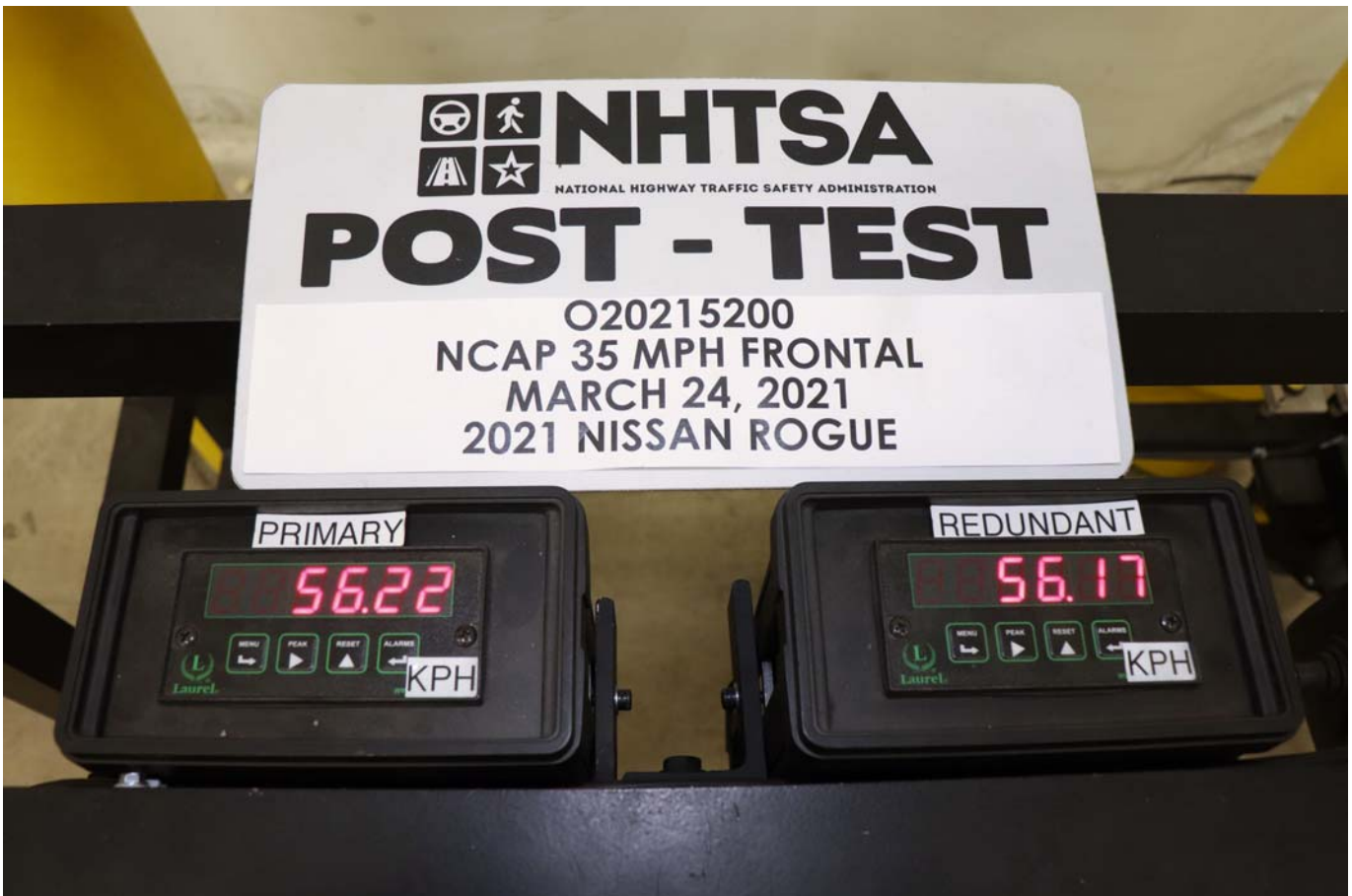
Photo No. 076 - Post-Test Speed Trap Read-Out
