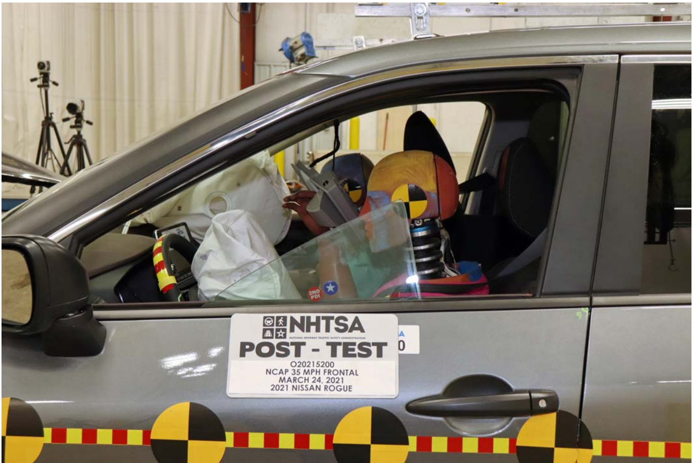
Photo No. 033 - Post-Test Driver Dummy Window View
