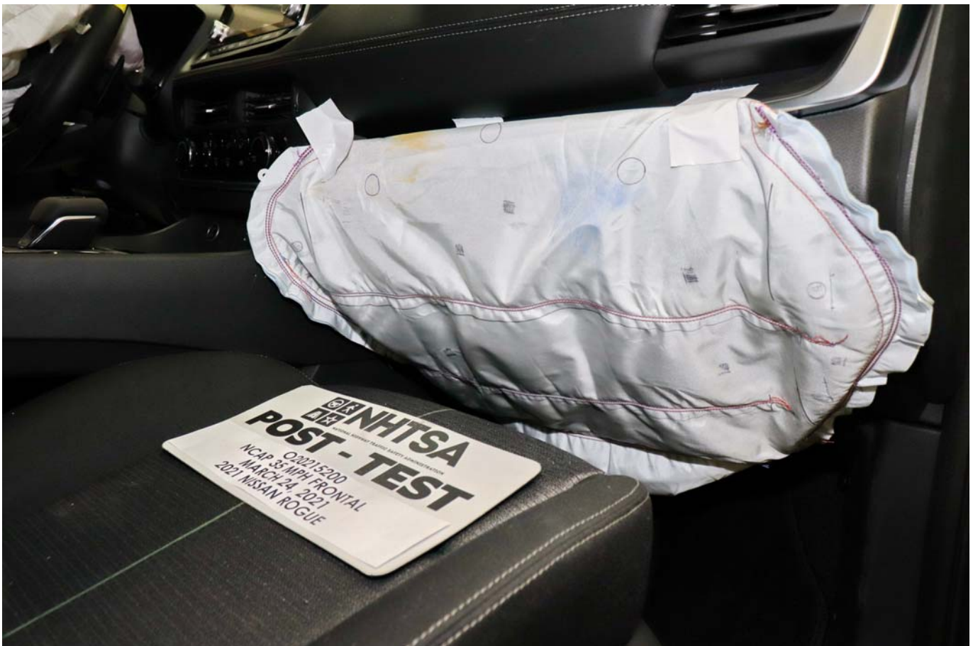
Photo No. 068 - Post-Test Passenger Side Knee Bolster
