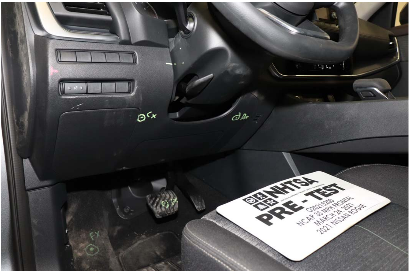
Photo No. 044 - Pre-Test Driver Side Knee Bolster
