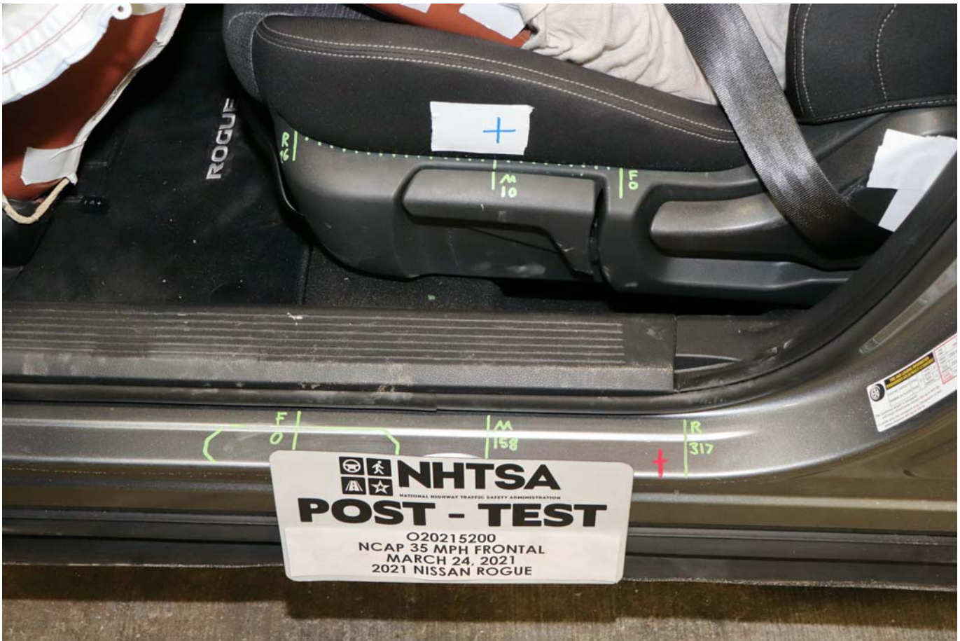
Photo No. 037 - Post-Test Driver Seat Fore-Aft Markings
