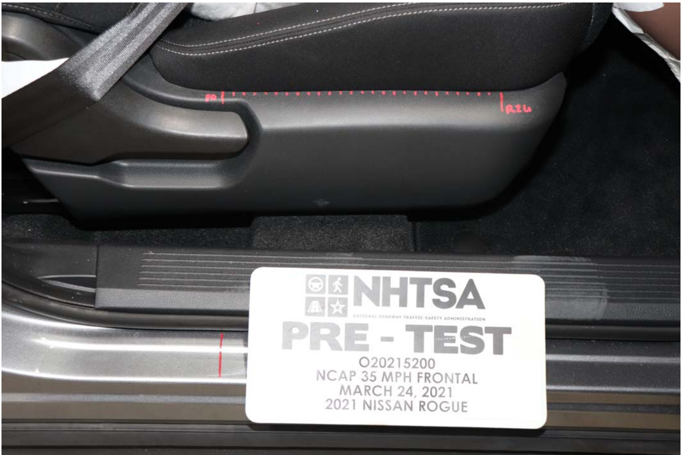
Photo No. 059 - Pre-Test Passenger Seat Fore-Aft Markings
