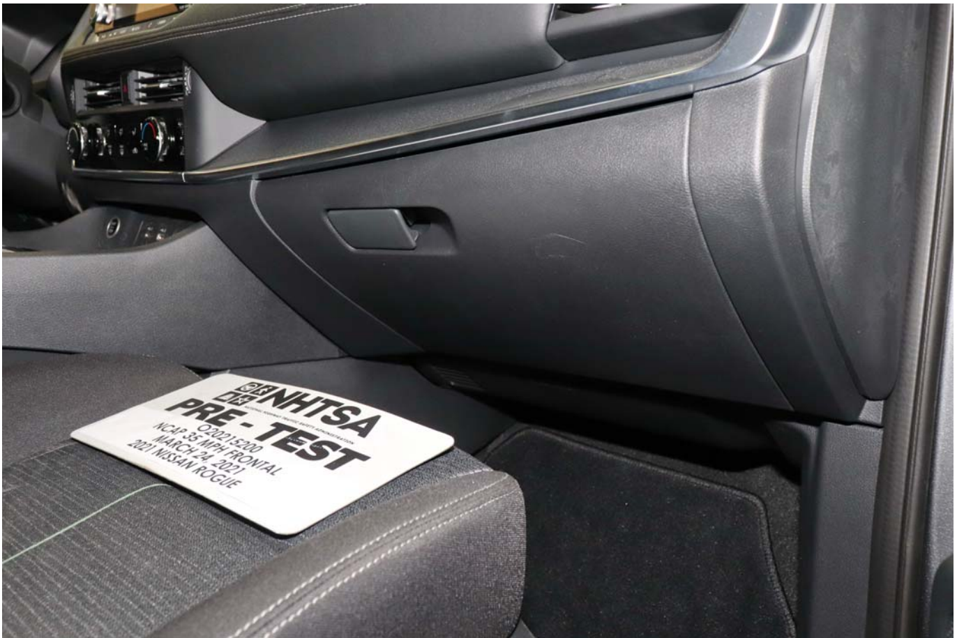
Photo No. 067 - Pre-Test Passenger Side Knee Bolster
