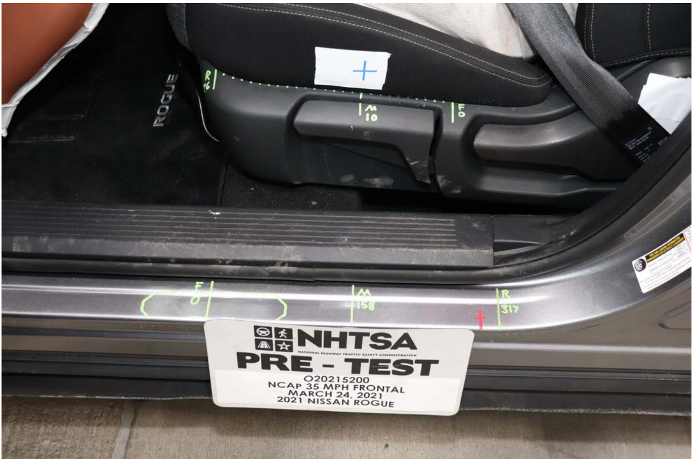
Photo No. 036 - Pre-Test Driver Seat Fore-Aft Markings
