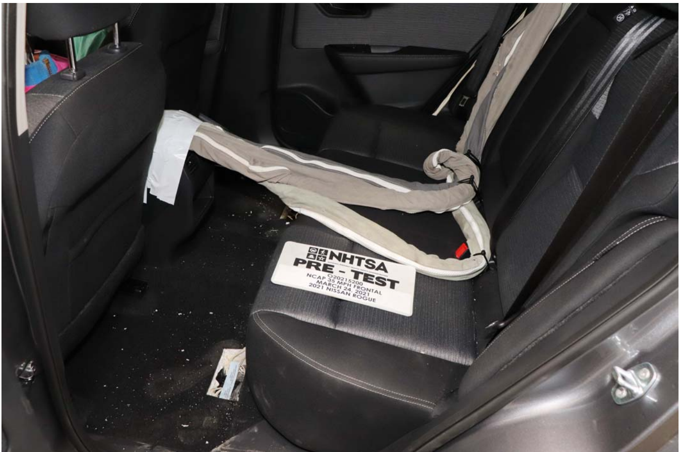
Photo No. 028 - Pre-Test Dummy Cable Routing
