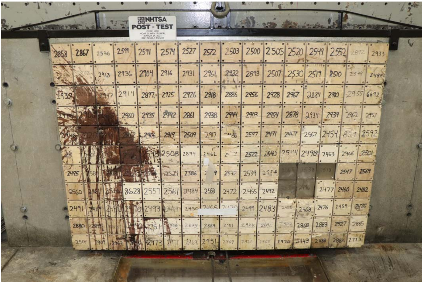
Photo No. 003 - Post-Test Load Cell Wall
