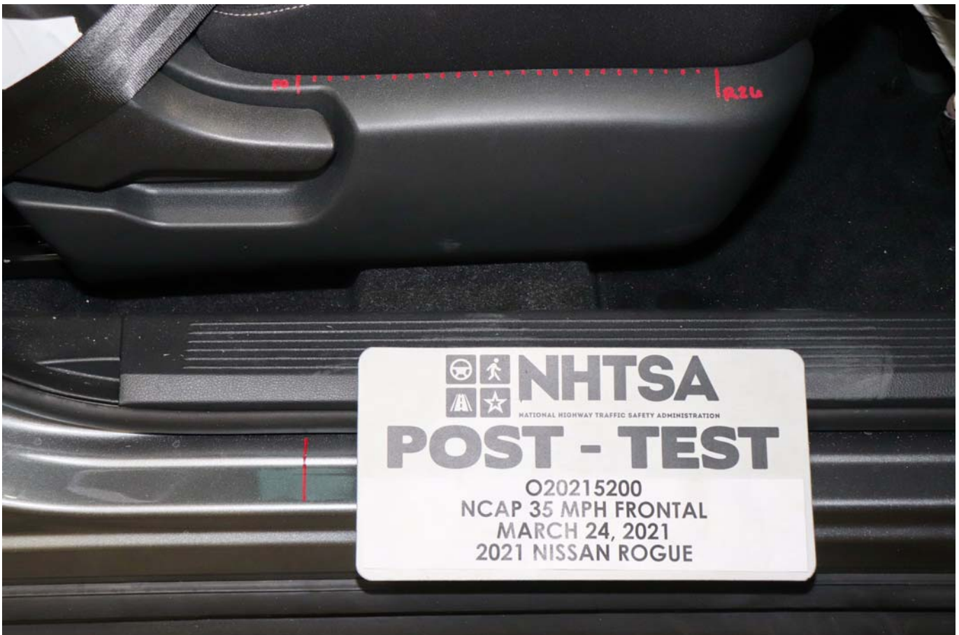
Photo No. 060 - Post-Test Passenger Seat Fore-Aft Markings
