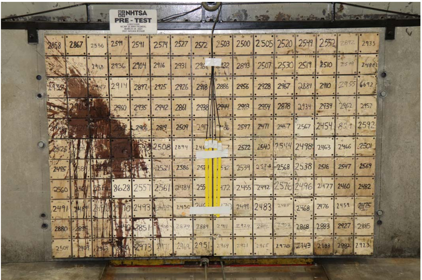
Photo No. 002 - Pre-Test Load Cell Wall
