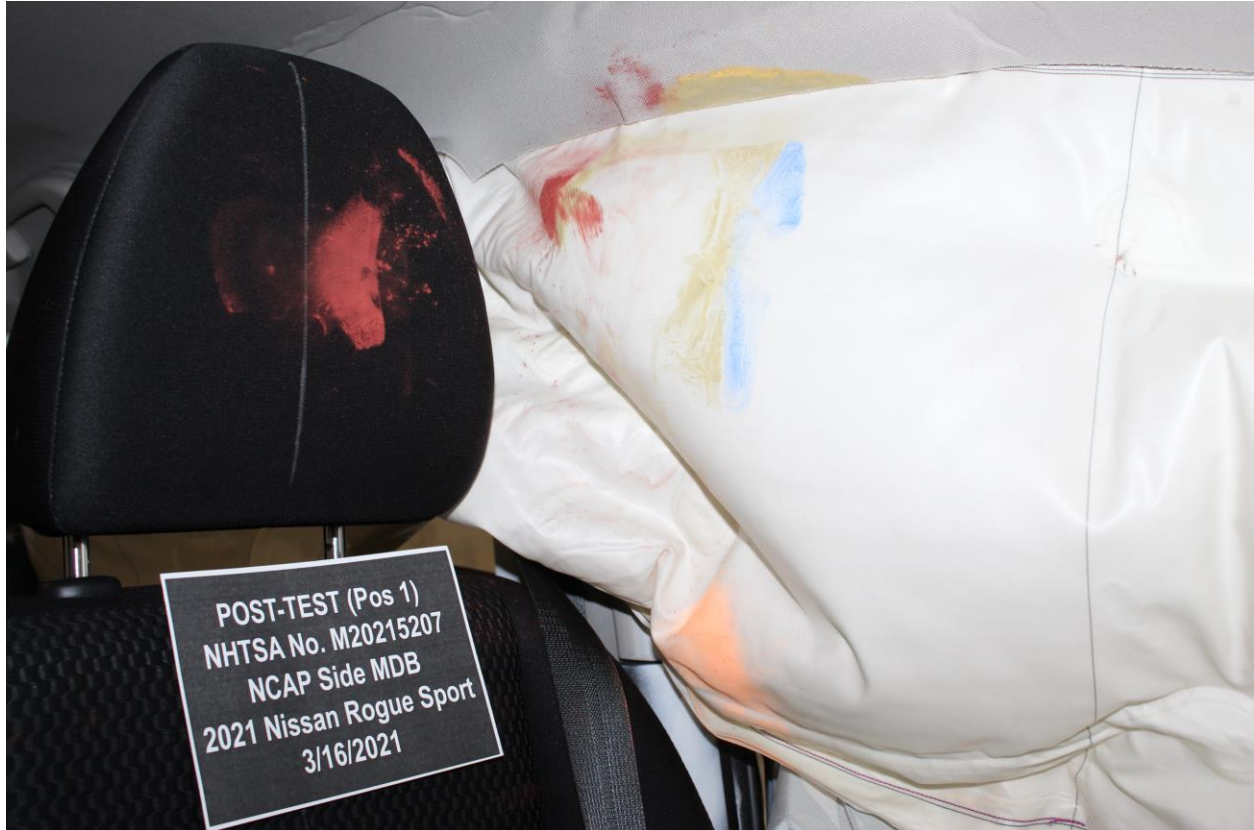
Figure A-48: Post-Test Driver Dummy Close-Up Head Contact with Vehicle View
