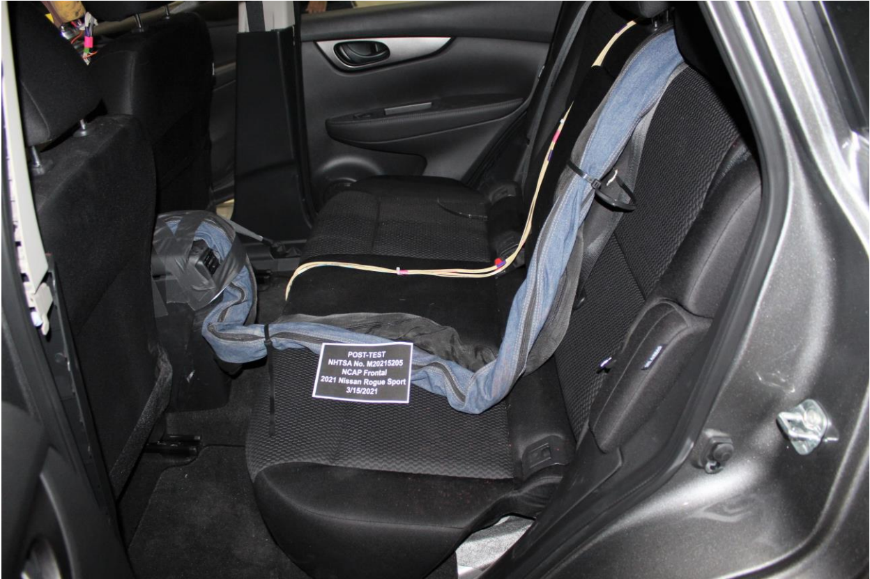
Figure A-29: Post-Test Dummy Cable Routing
