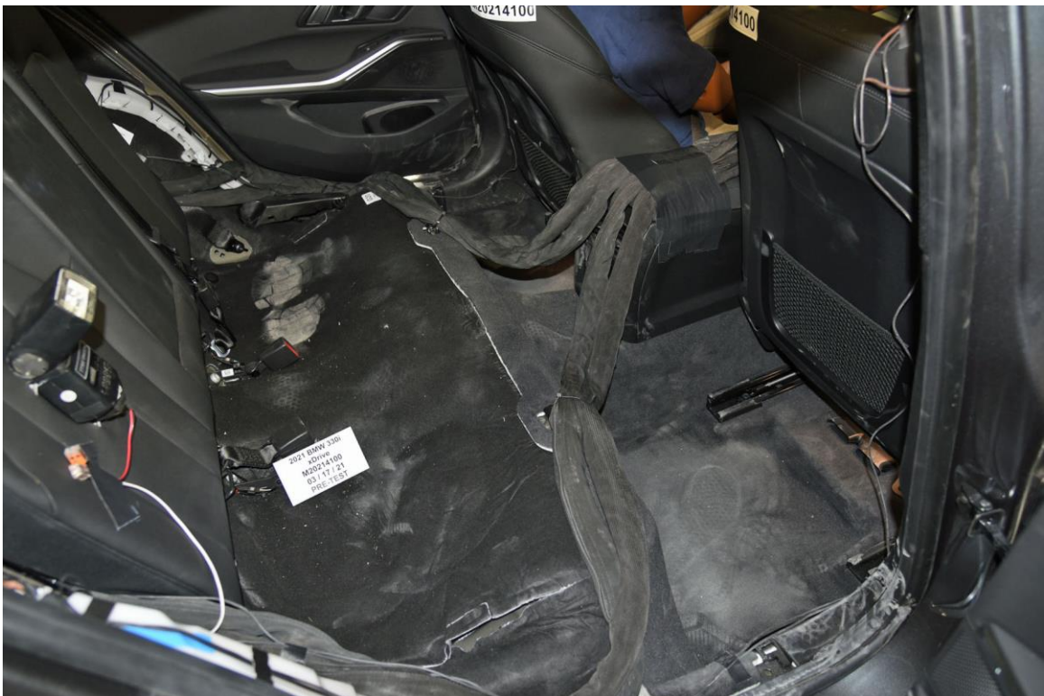
FIGURE 28. Pre-Test Dummy Cable Routing
